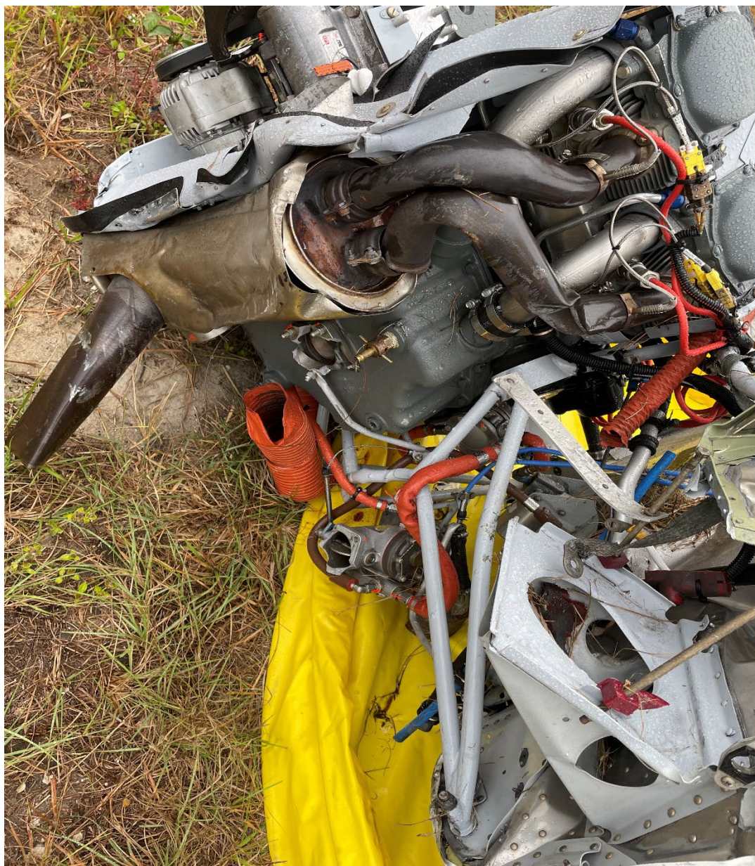
Photo 2 – View of engine separated from firewall showing bent engine mount and separated fuel servo.
