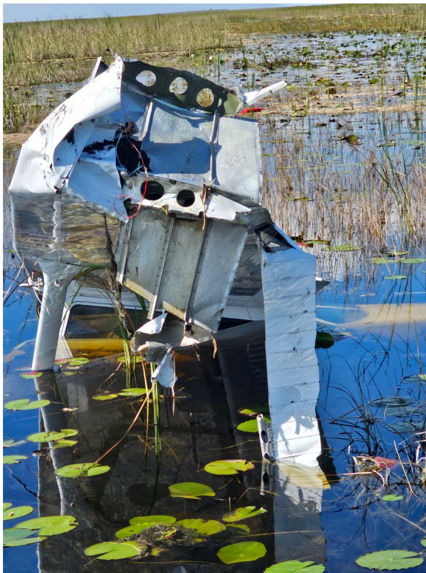
Photograph 2 - FAA Digital Photograph Left Side View of the Airplane At the Accident Site. Note the damage to the Left Wing
