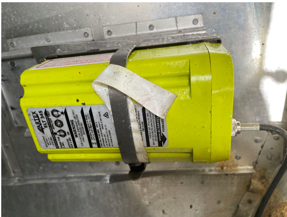
Photograph 7 - FAA Digital Photograph View of the Installed Emergency Locator Transmitter Note the BNC Antenna Connector Still Attached
