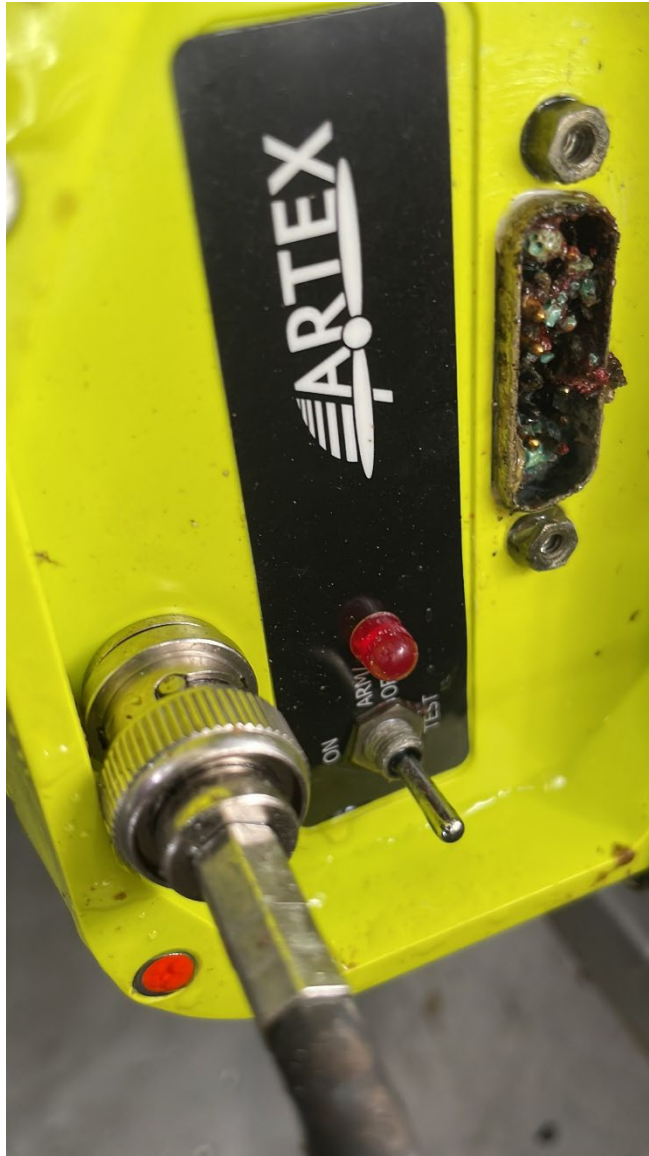
Photograph 8 - FAA Digital Photograph View Showing the Antenna BNC Connector Installed But the 15-Pin D-SUB Connector Separated
