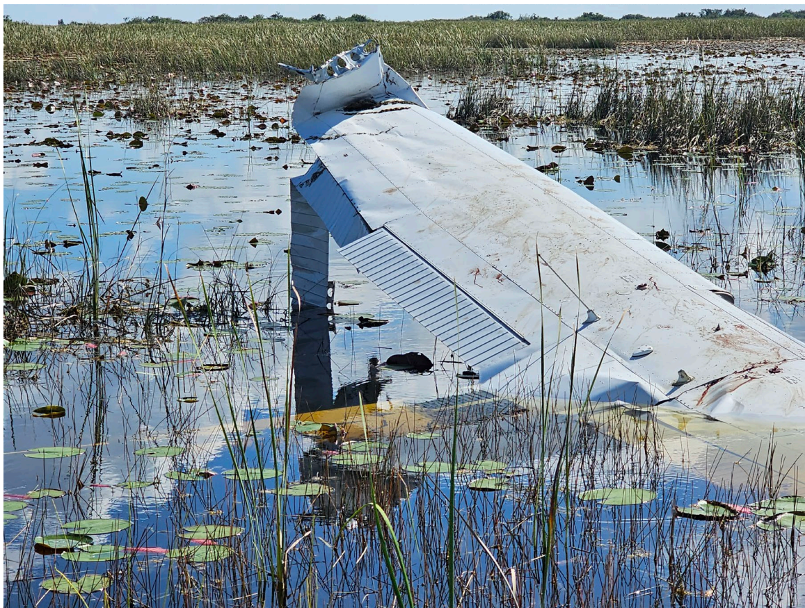
Photograph 3 - FAA Digital Photograph View Showing the Upper Inboard Portion of the Right Wing and the Full Span of the Upper Portion of the Left Wing. Note the Compression Wrinkles in the Upper Wing Skins of Both Wings
