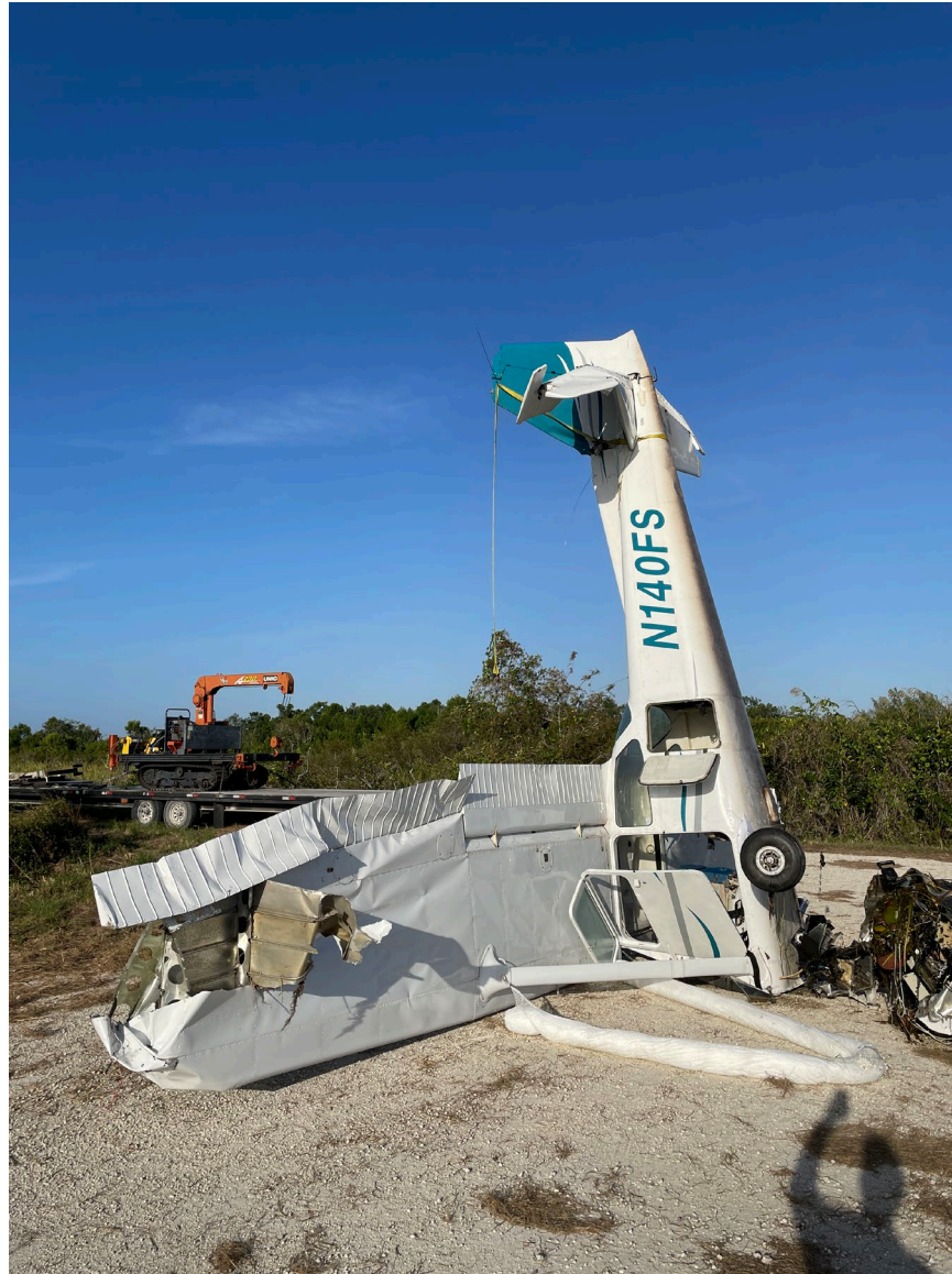
Photograph 6 - FAA Digital Photograph Left Side View of the Airplane Following Recovery. Note the Extensive Damage to the Left Wing
