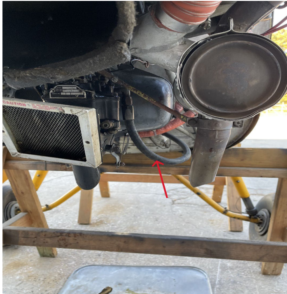
Photograph 4 - Failed carburetor fuel line from (Courtesy of NTSB)
