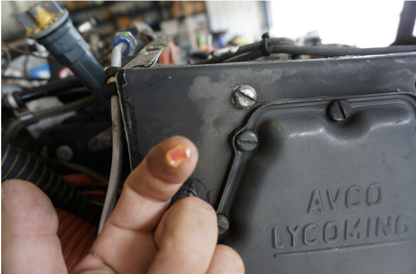
Photograph 21 - Fuel Distribution Manifold - Positive Reaction for Water
