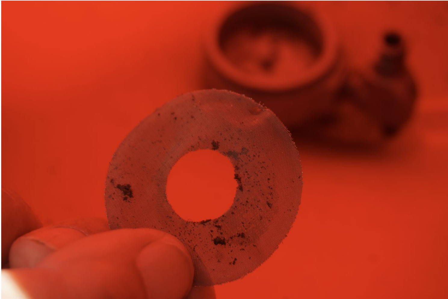
Photograph 19 - Fuel Strainer Screen
