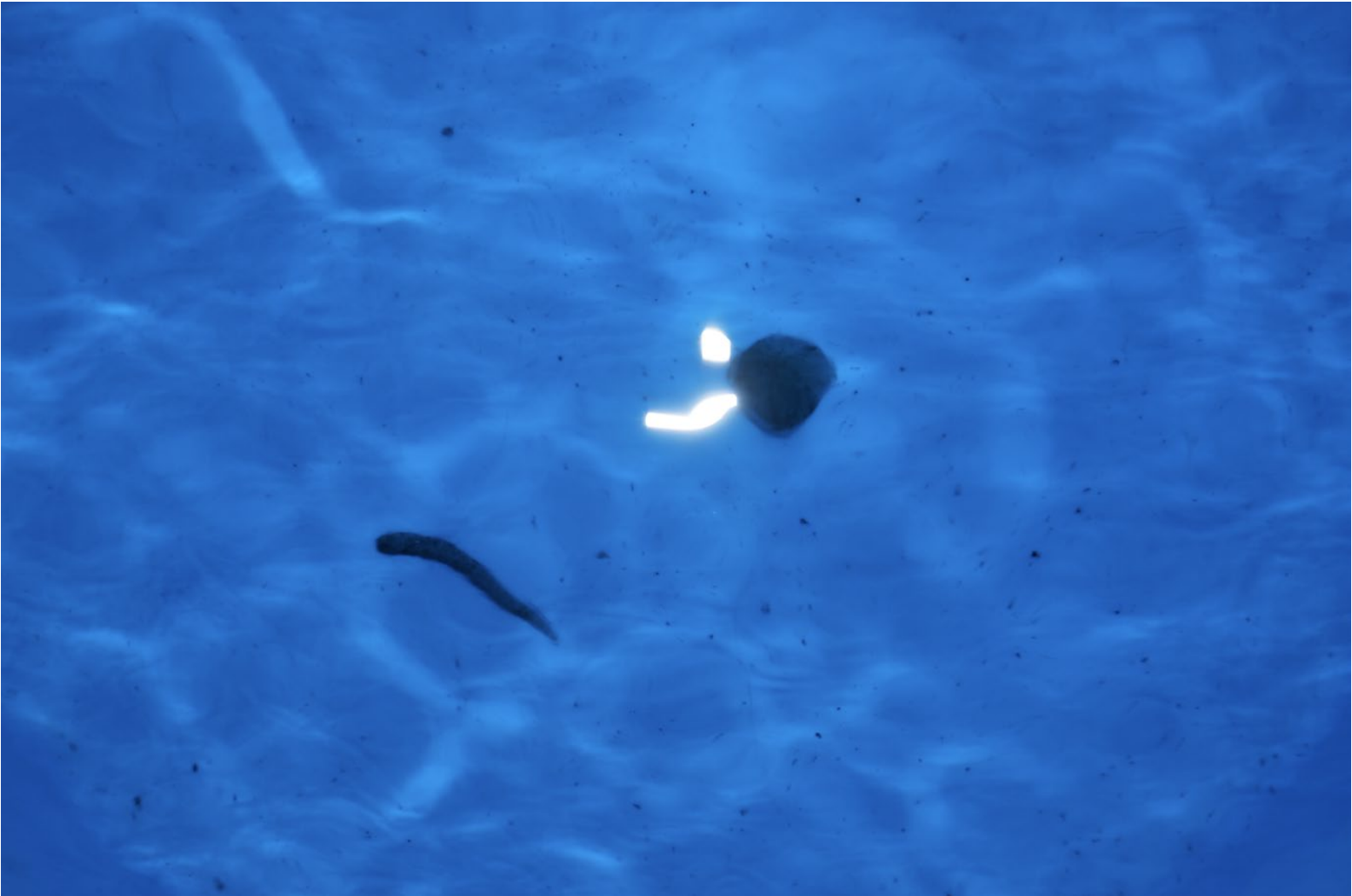
Photograph 16 - Contents of Right Wing Fuel Tanks after Draining
