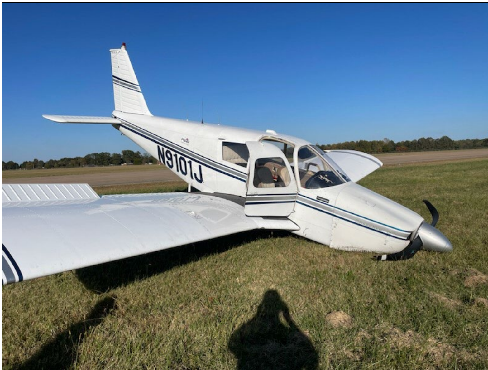
Figure 1: Overview of the airplane at the accident site with a collapsed nose landing gear (Photo Courtesy of FAA)
