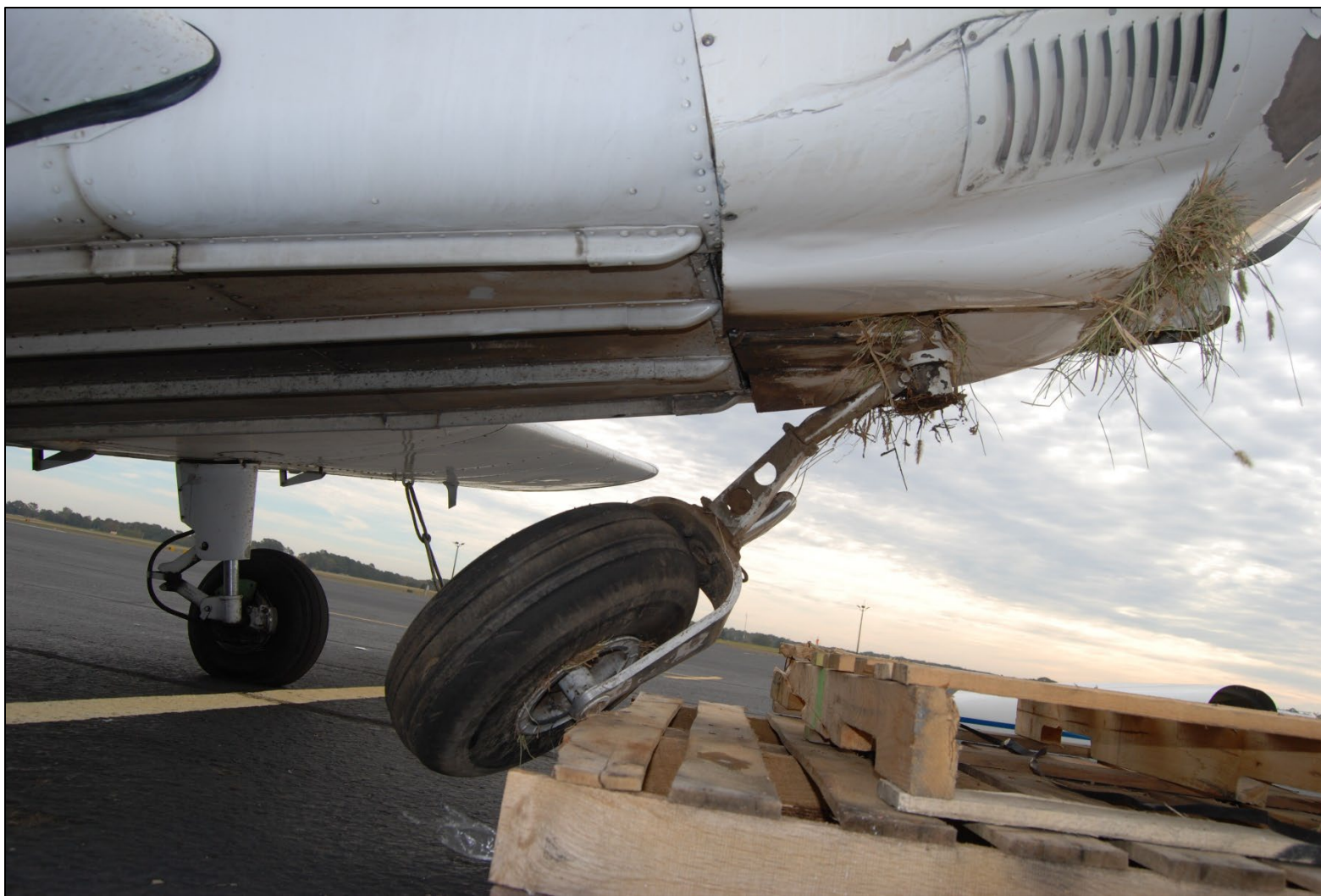
Figure 2: View of the collapsed nose landing gear (Photo Courtesy of FAA)
