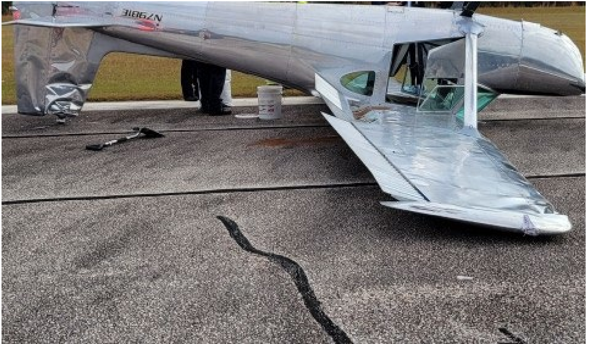
Photo 1 – Photo From NTSB Duty Officer. Left Side View of the Inverted Airplane Where it Came to Rest. Note the Structural Damage to the Vertical Stabilizer.
