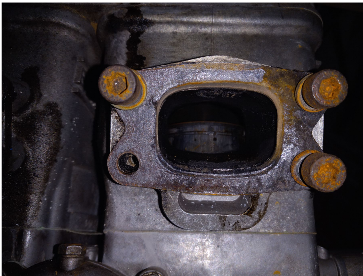
Photograph 4 - Scoring Damage to Forward Piston (Courtesy of FAA)
