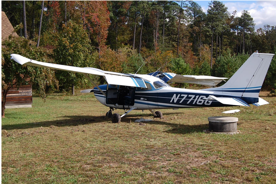
Photograph 1 - View of left side of airplane showing damage to both wings. (Courtesy of FAA)
