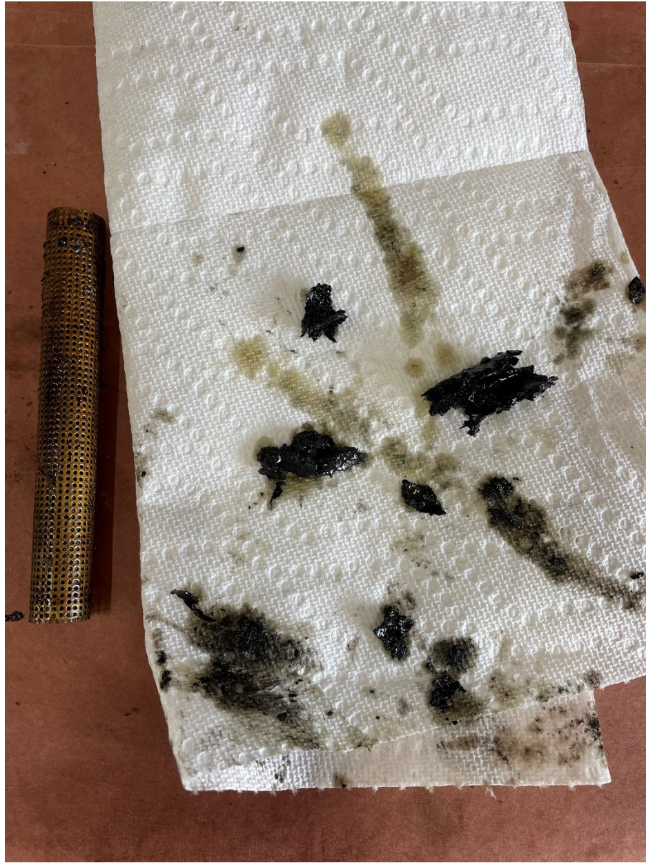
Photo 4 – Sludge-like carbon material found in oil suction screen
