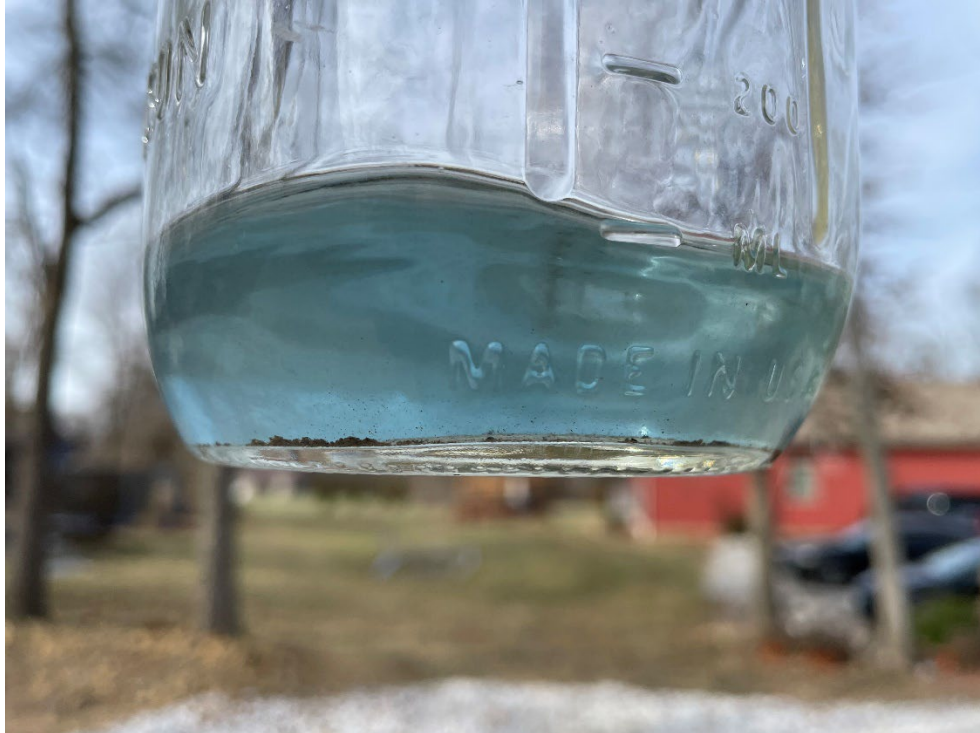
Photo 1 – Fuel recovered from gascolator, note fine particulates
