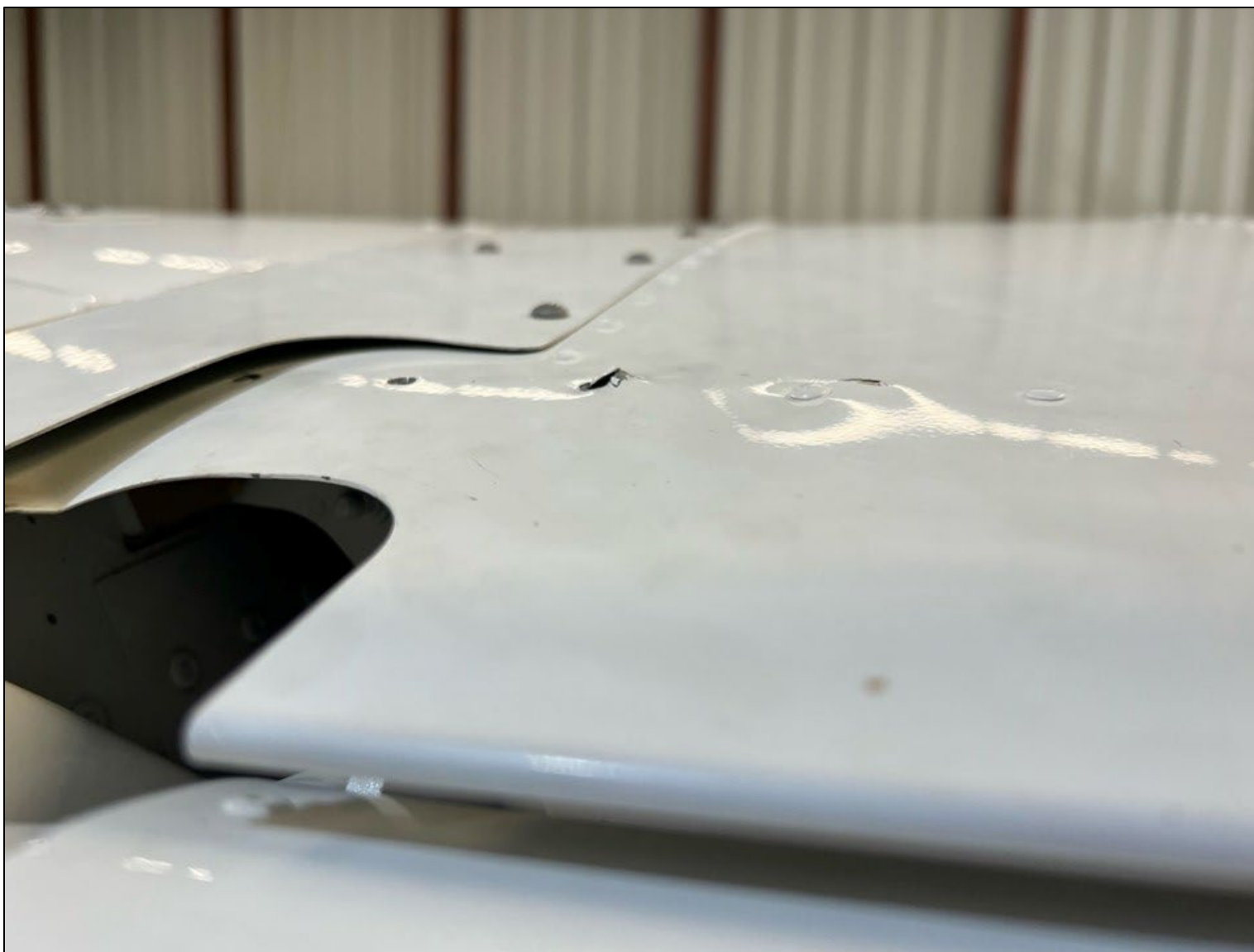
Figure 1: Overview of the substantially damage right wing (Photo Courtesy FAA)
