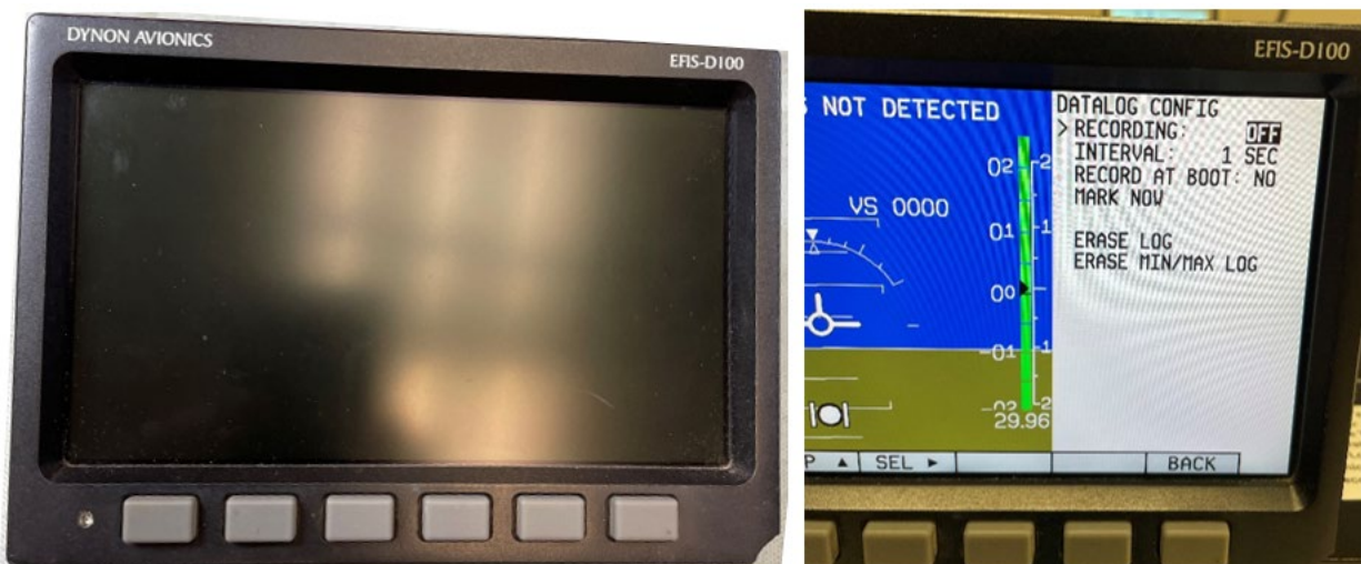
Figure 2. Dynon EFIS-D100 as received by the NTSB Vehicle Recorder Laboratory (left) and the Dynon EFIS-D100 powered on (right) with the datalog config page showing the recording feature set to "off."
