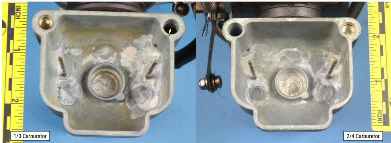
Figure 5. Closer photographs of the interior of the float chamber with the floats removed. Areas of white film and accumulations of white and yellow material deposits were observed on the base of both float chambers. Similar white deposits were observed around the sidewall of the 1/3 carburetor float chamber jet as indicated by the yellow arrow.
