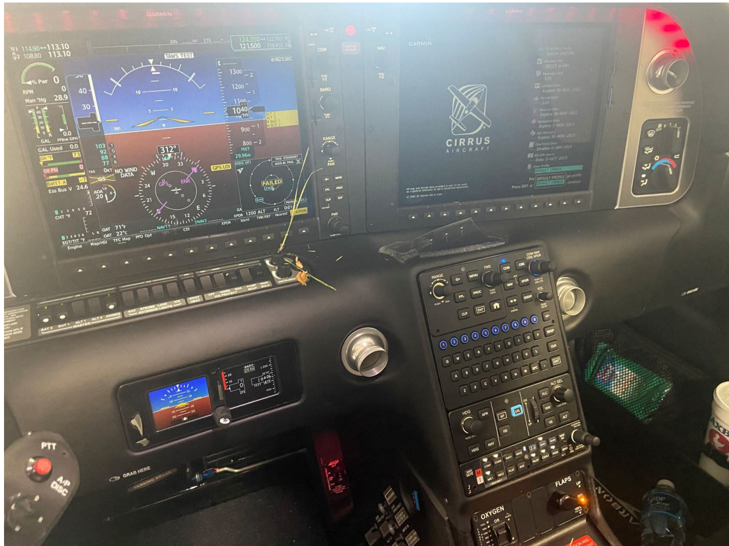
Photograph 6 - PFD, MFD, and MD302 operating after accident (Courtesy of FAA)
