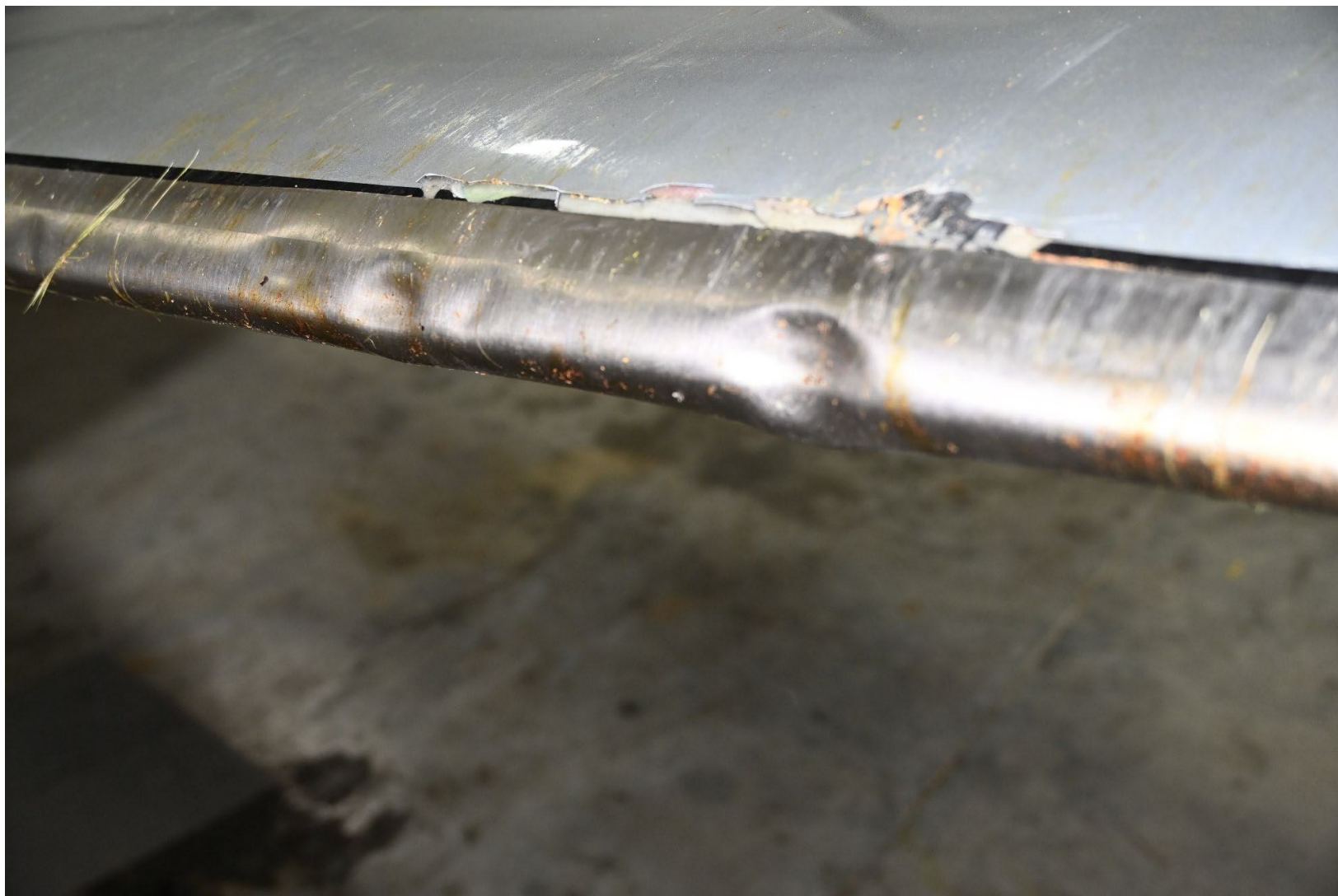
Photograph 4 - Damage to the left wing (Courtesy of Cirrus)
