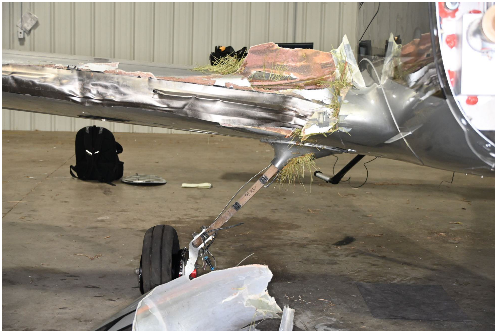
Photograph 3 - Damage to the right wing (Courtesy of Cirrus)
