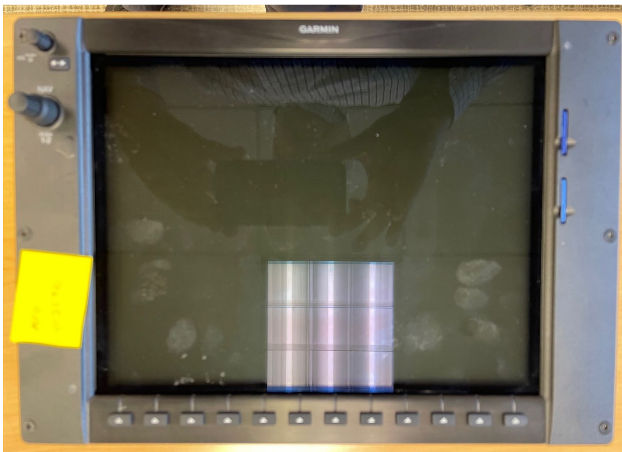
Figure 2. The airplane's MFD, as marked by investigators, removed from the airplane.
