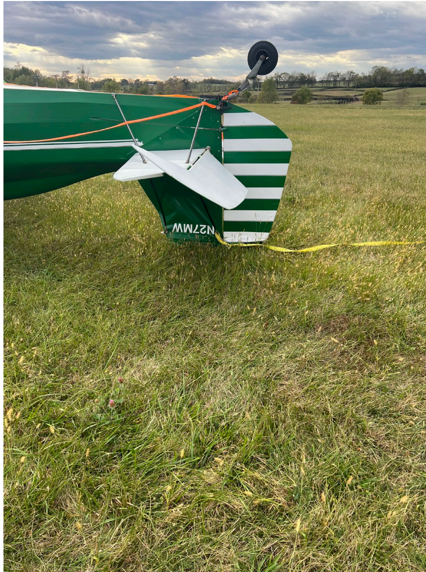
Photograph 2 - Vertical Stabilizer and Rudder Damage (Courtesy of FAA)
