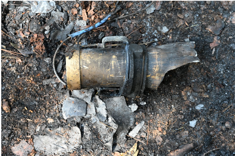
Damaged Portion of the CAPS System (Courtesy of Cirrus)
