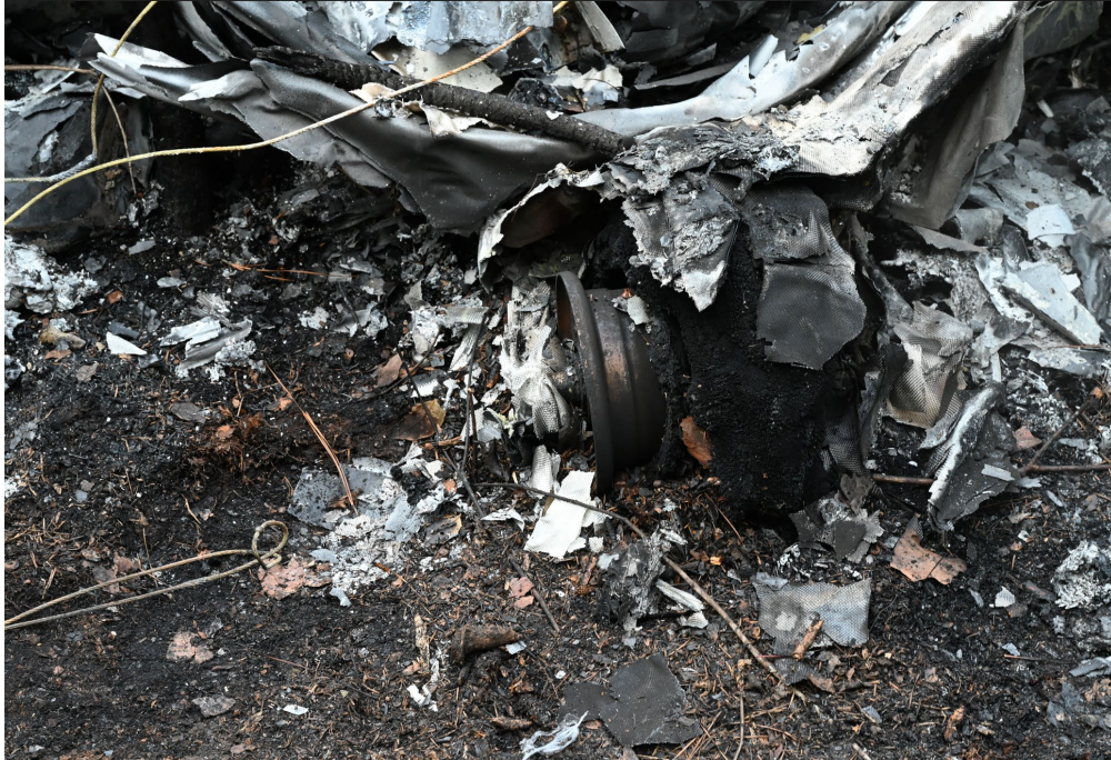
Left Main Landing Gear (Courtesy of Cirrus)
