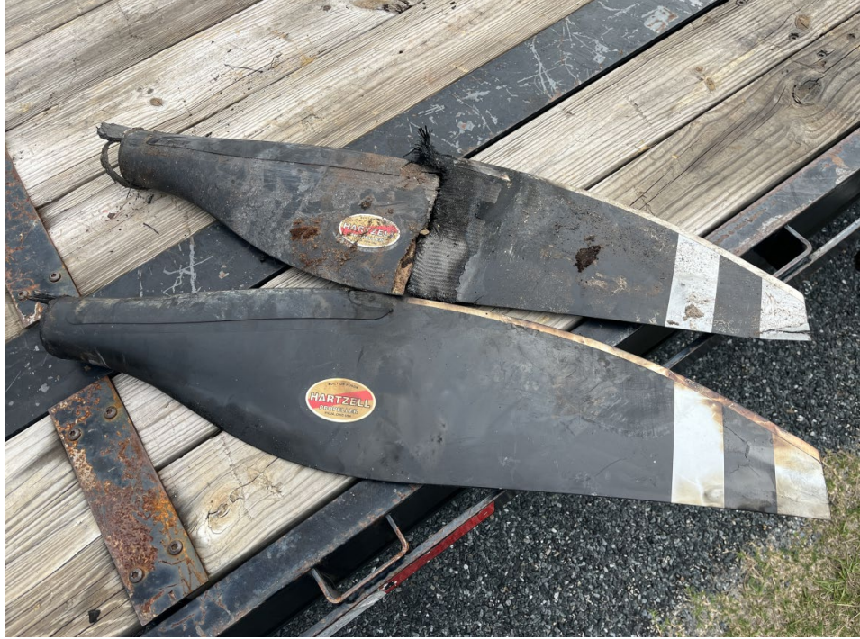
Propeller Blade Damage
