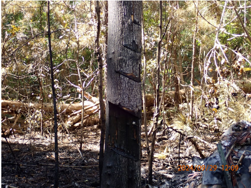
Propeller Strike Signatures in Tree
