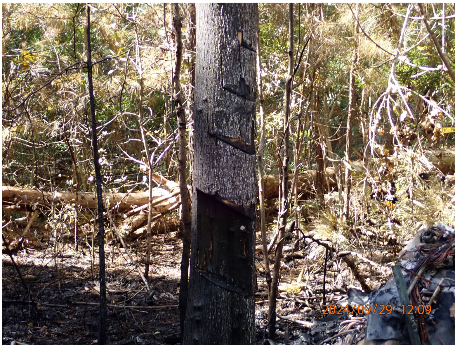
Photograph 2 - Propeller Strike Marks in a Tree at the Nose of the Airplane On-Scene
