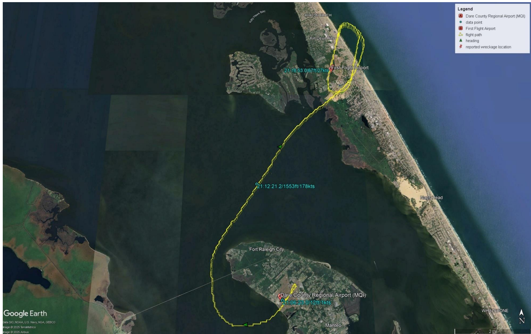
Figure 14. Google Earth overlay of the entire accident flight. Note that the zig-zag shape flight path was due to an Appareo RDM issue in recording GPS location data and not necessarily the exact flight pattern.
