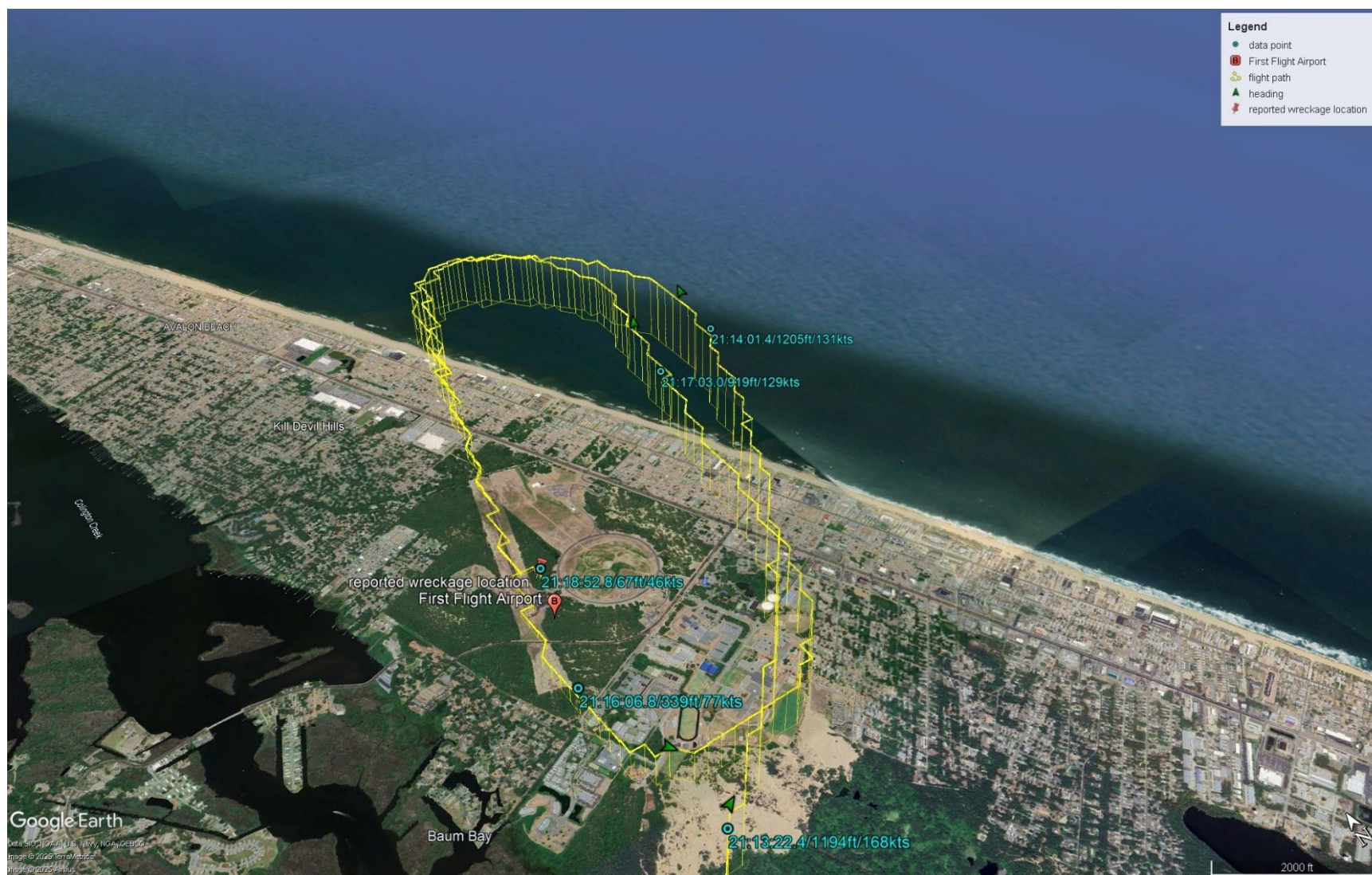
Figure 15. Google Earth overlay of the final portion of the accident flight. Note that the zig-zag shape flight path was due to an Appareo RDM issue in recording GPS location data and not necessarily the exact flight pattern.
