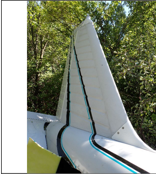
Figure 13: Vertical stabilizer and rudder
