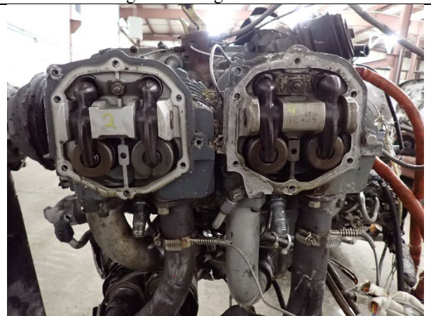
Figure 26: No. 2 and No. 4 cylinder overhead components
