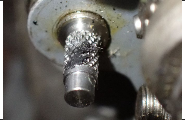
Figure 36: Fuel injection servo throttle stop pin (missing plastic)
