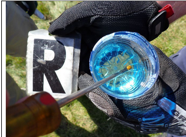
Figure 19: Fuel sample from right fuel tank (testing with water finding paste)
