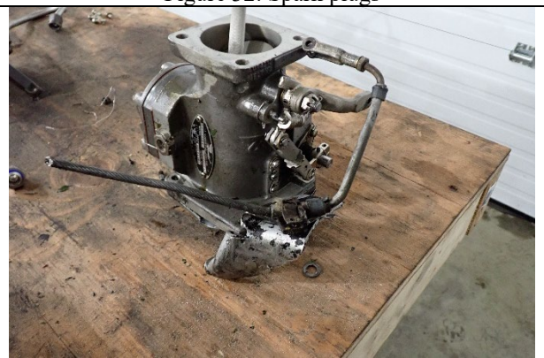
Figure 34: Fuel injection servo after removal
