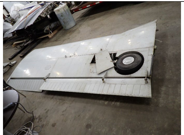
Figure 16: Right wing overview after recovery
