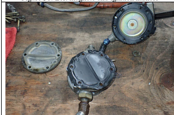
Figure 33: Fuel pump after disassembly
