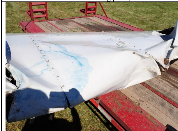
Figure 21: Left wing fuel tank with blue staining
