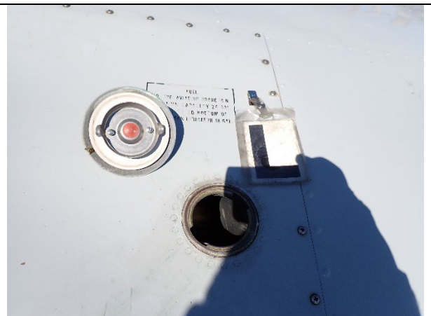
Figure 22: Left fuel cap and filler port
