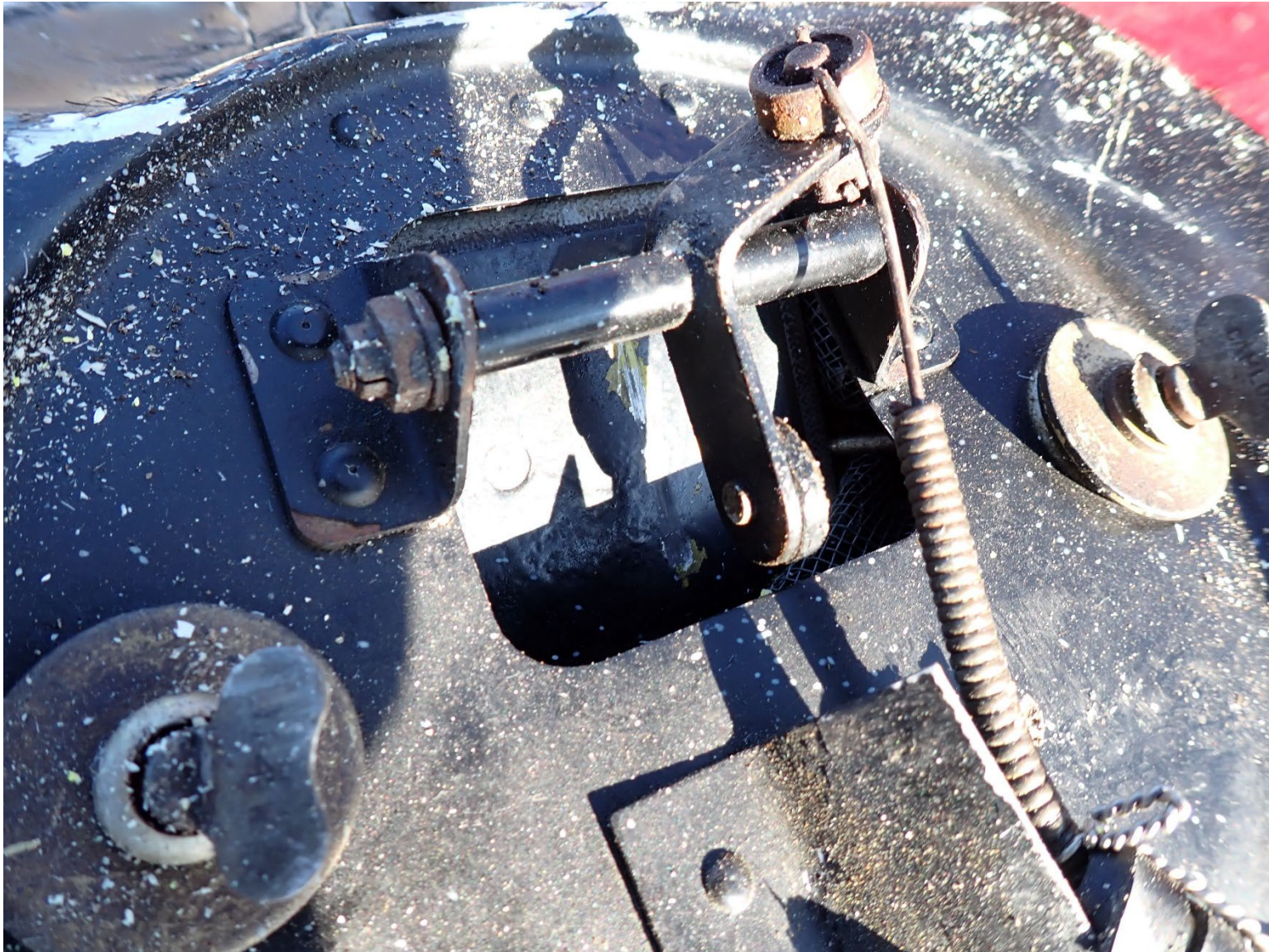
Photograph 8 - Alternate air door
