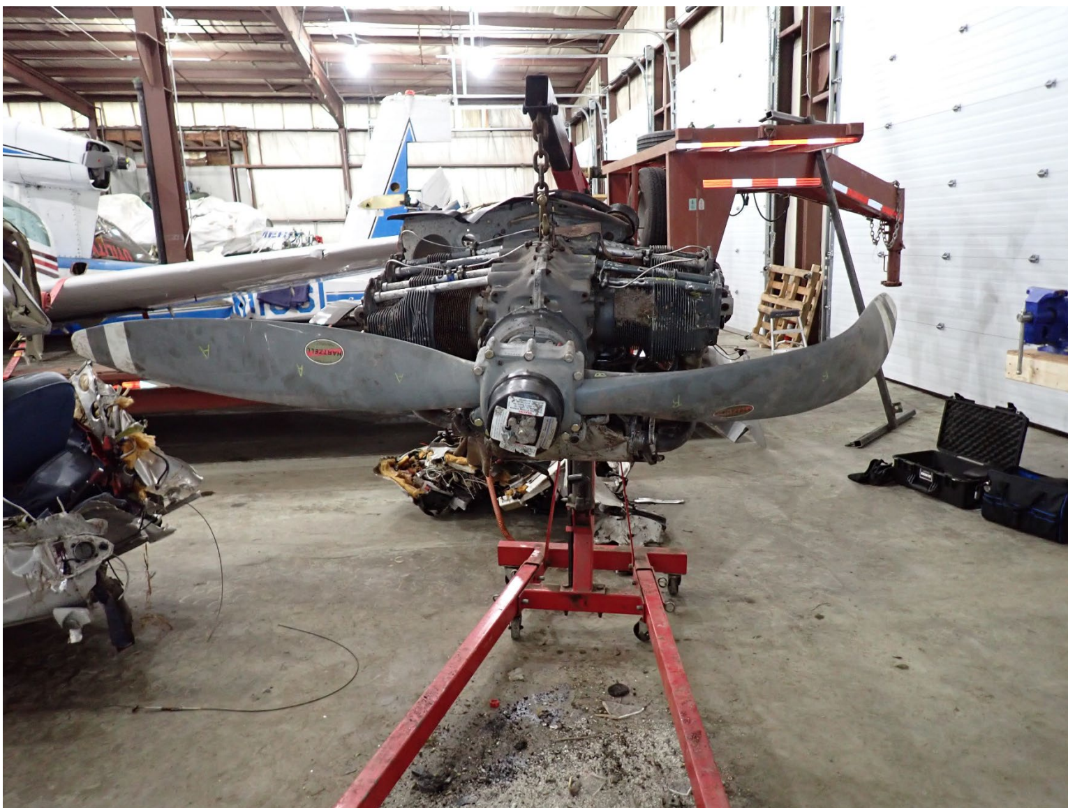
Photograph 10 - Engine overview after recovery
