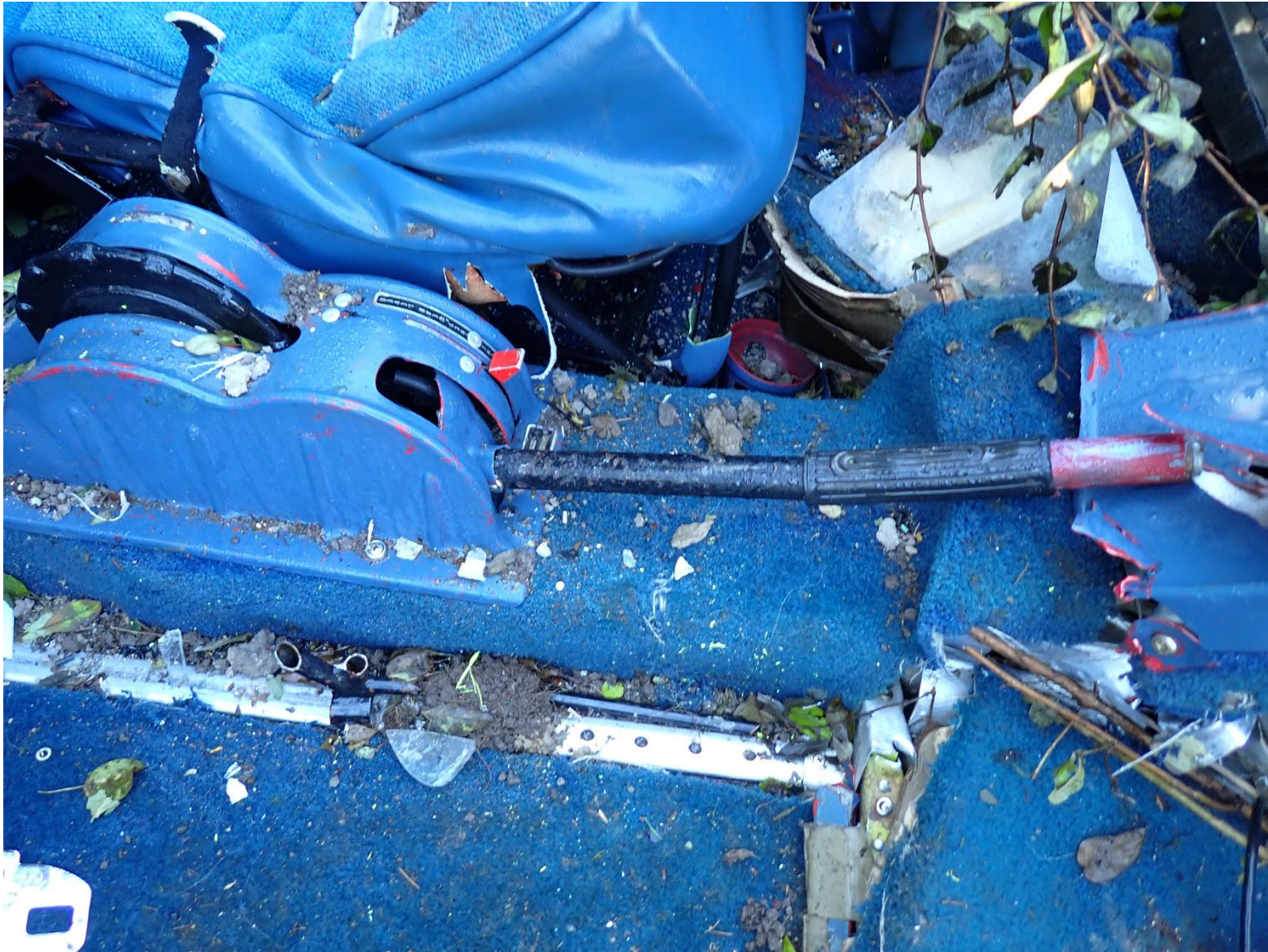
Photograph 3 - Flap control bar
