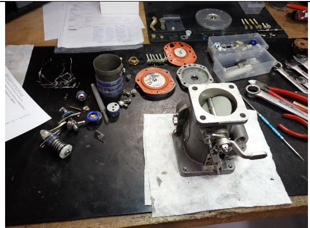
Photograph 4: Fuel servo disassembled
