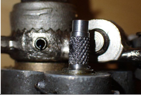
Photograph 7: Servo throttle stop with visible wear
