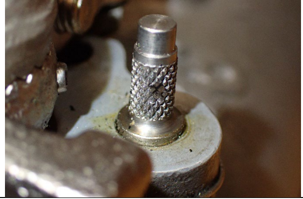
Photograph 8: Servo throttle stop with visible wear
