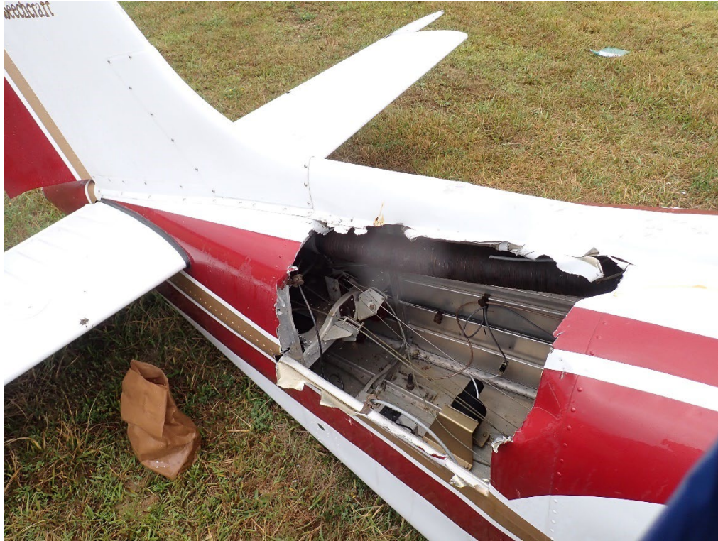
Figure 2: Empennage with hole cut into interior to access the control cables and ELT.
