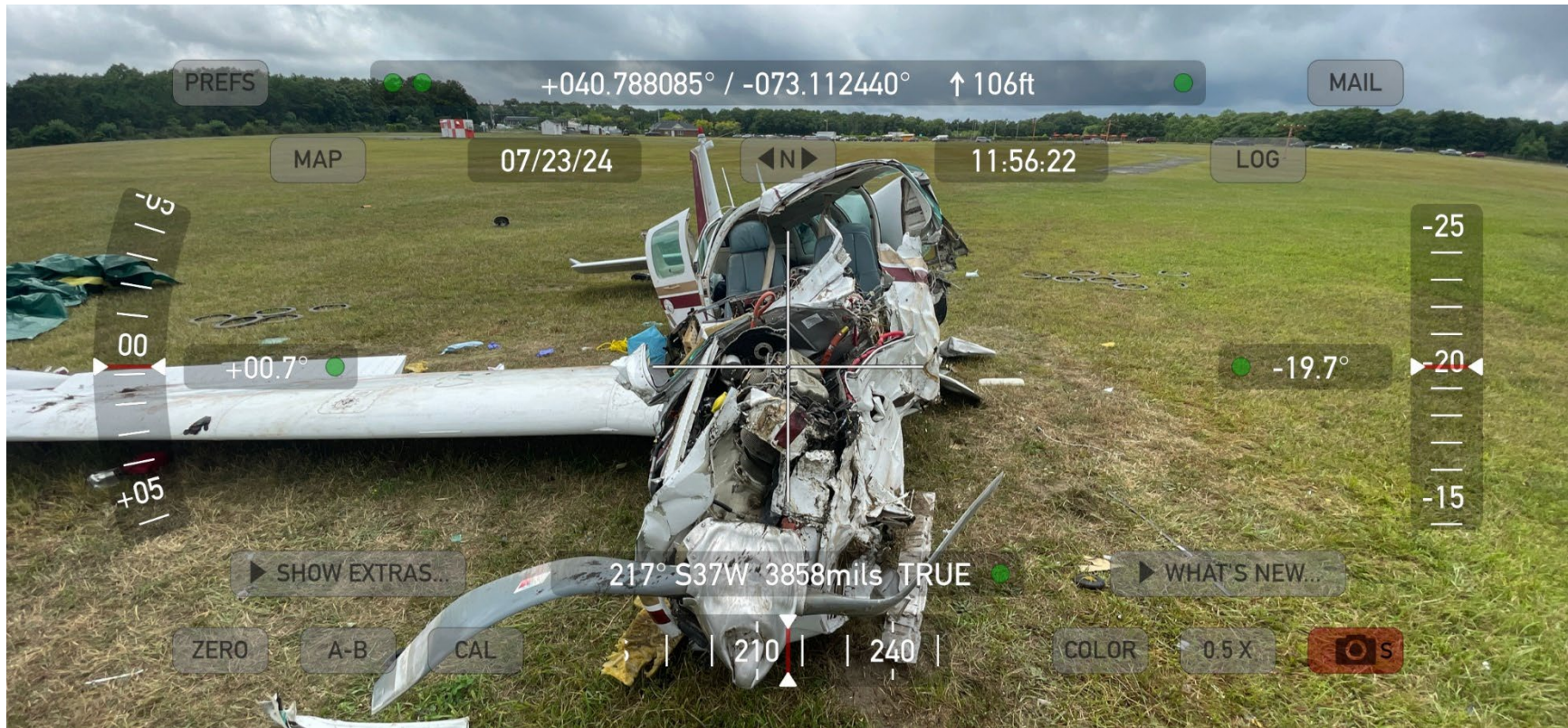
Photograph 2 - Theodolite view of wreckage showing lat/long, elevation and magnetic heading. (NTSB)
