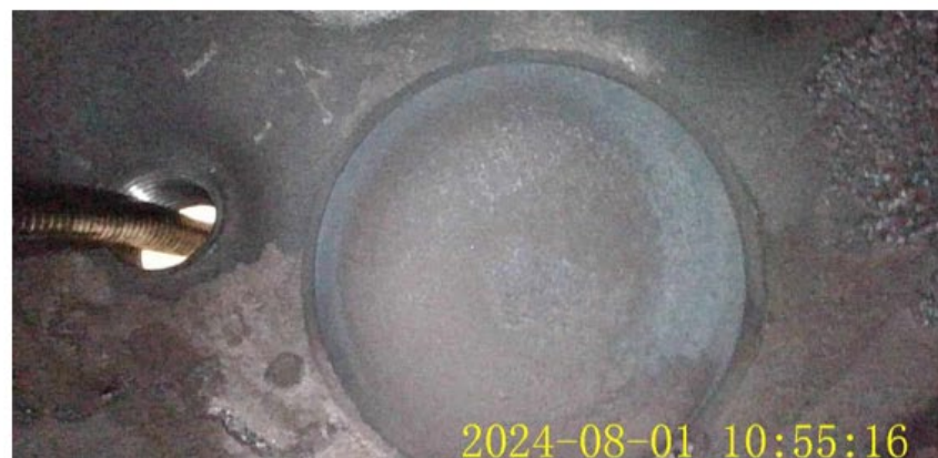
Photograph 15 - Borescope of number 2 cylinder, valves, and piston. Equivalent results were observed on all 6. (NTSB)
