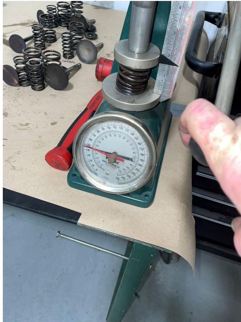
Photograph 14 - View of valve spring testing. All six cylinders exhibited equivalent results. (NTSB)
