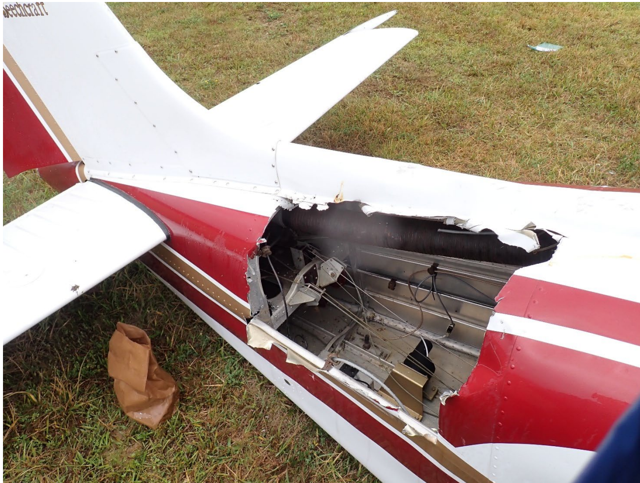
Photograph 8 - View of empennage with hole cut into fuselage for examination of flight control cables. (NTSB)
