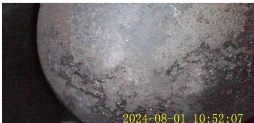
Photograph 15 - Borescope of number 2 cylinder, valves, and piston. Equivalent results were observed on all 6. (NTSB)
