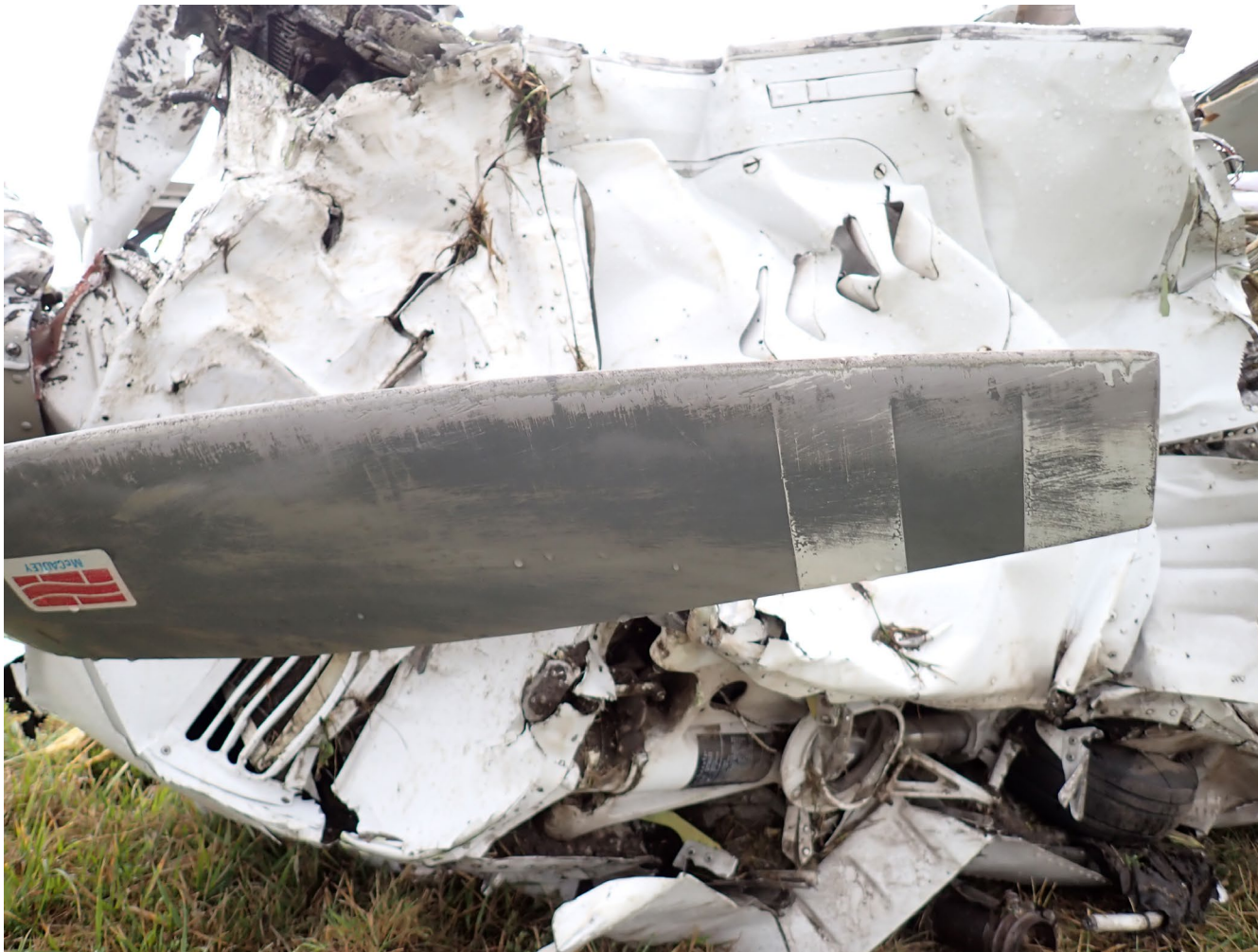
Photograph 7 - View of propeller blade damage. (NTSB)
