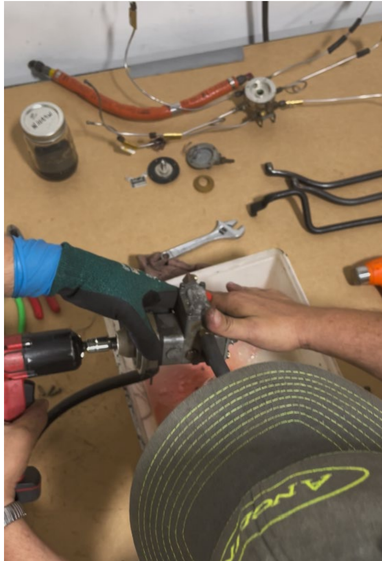
Photograph 13 - View of engine components testing, specifically the engine driven fuel pump. (NTSB)
