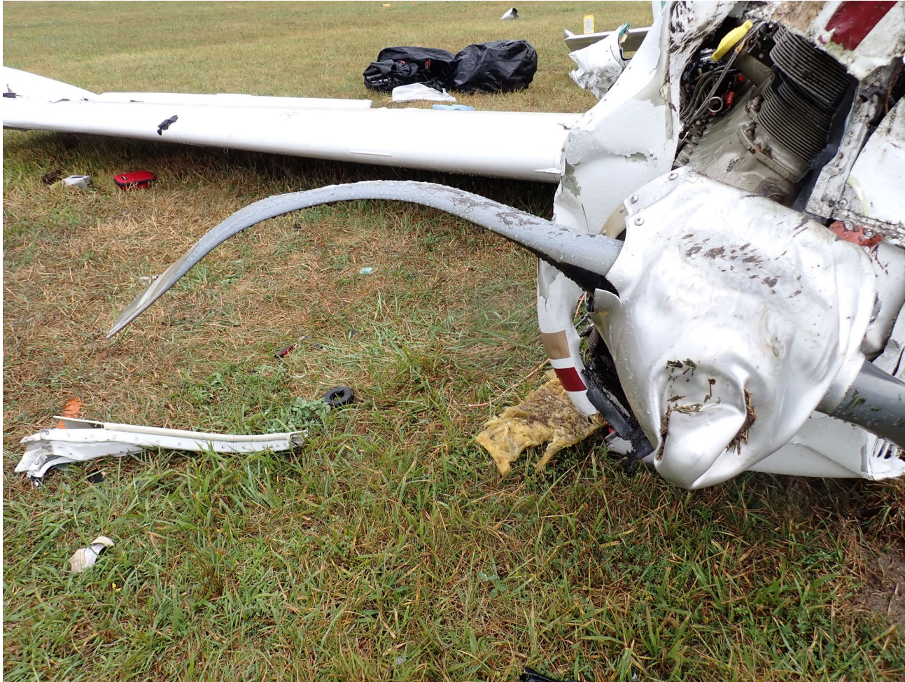
Photograph 6 - View of propeller blade damage. (NTSB)
