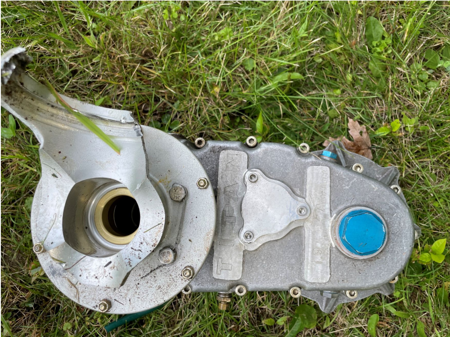
Photograph 3 - Propeller gearbox at accident site
