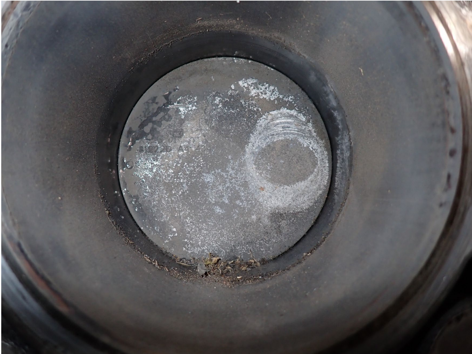
Photograph 10 - No. 1 piston with valve strike impressions
