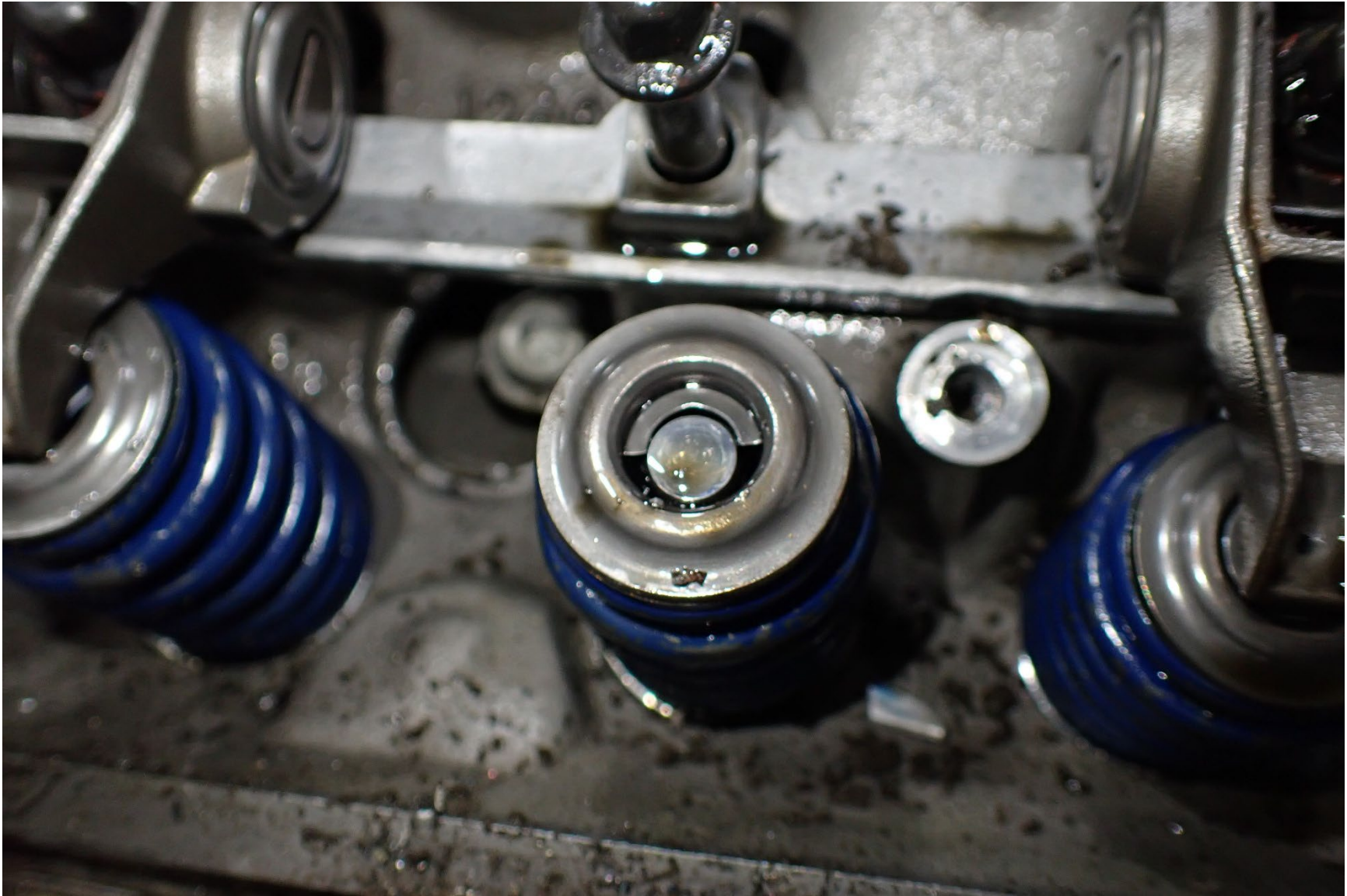
Photograph 9 - No. 3 intake valve missing one valve key
