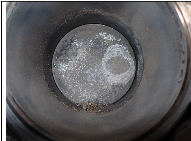
Figure 4: No. 1 piston with valve strike impressions
