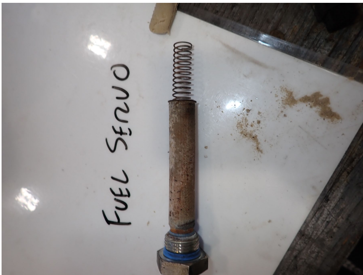
Photograph 9 - Left Engine Fuel Servo Inlet Screen and Debris (NTSB Photo)
