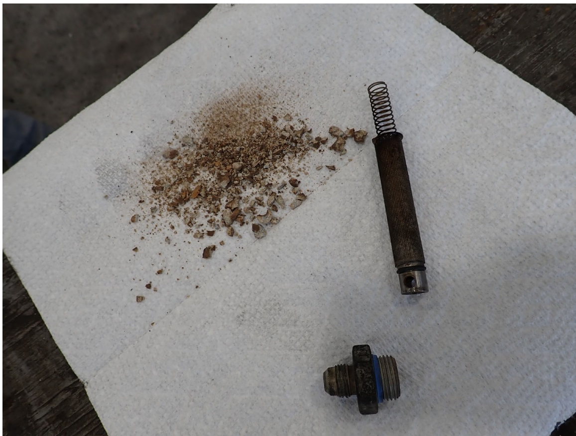
Photograph 12 - Right Engine Fuel Servo Inlet Screen and Debris (NTSB Photo)
