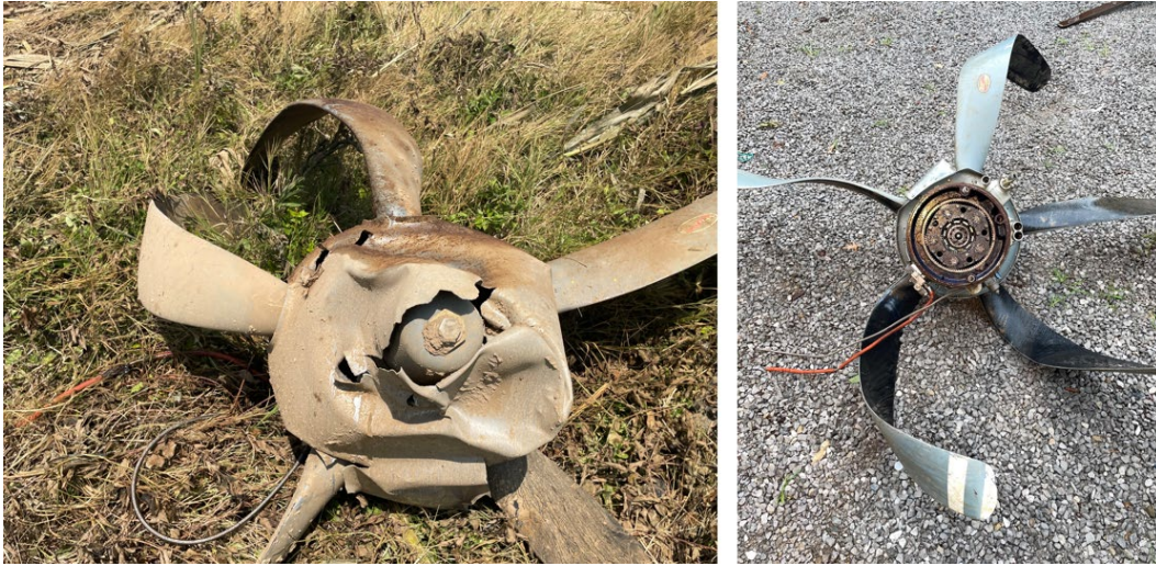
Figure 22 Propeller assy. As found on site (L) and during examination. (R)
