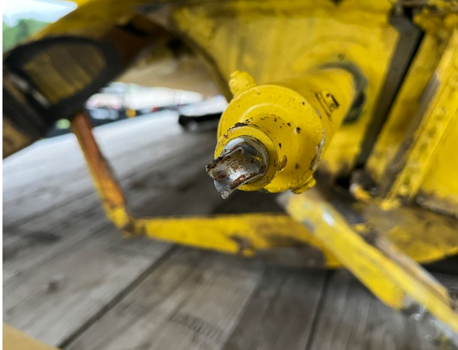
Figure 9 Control rod overload damage.
