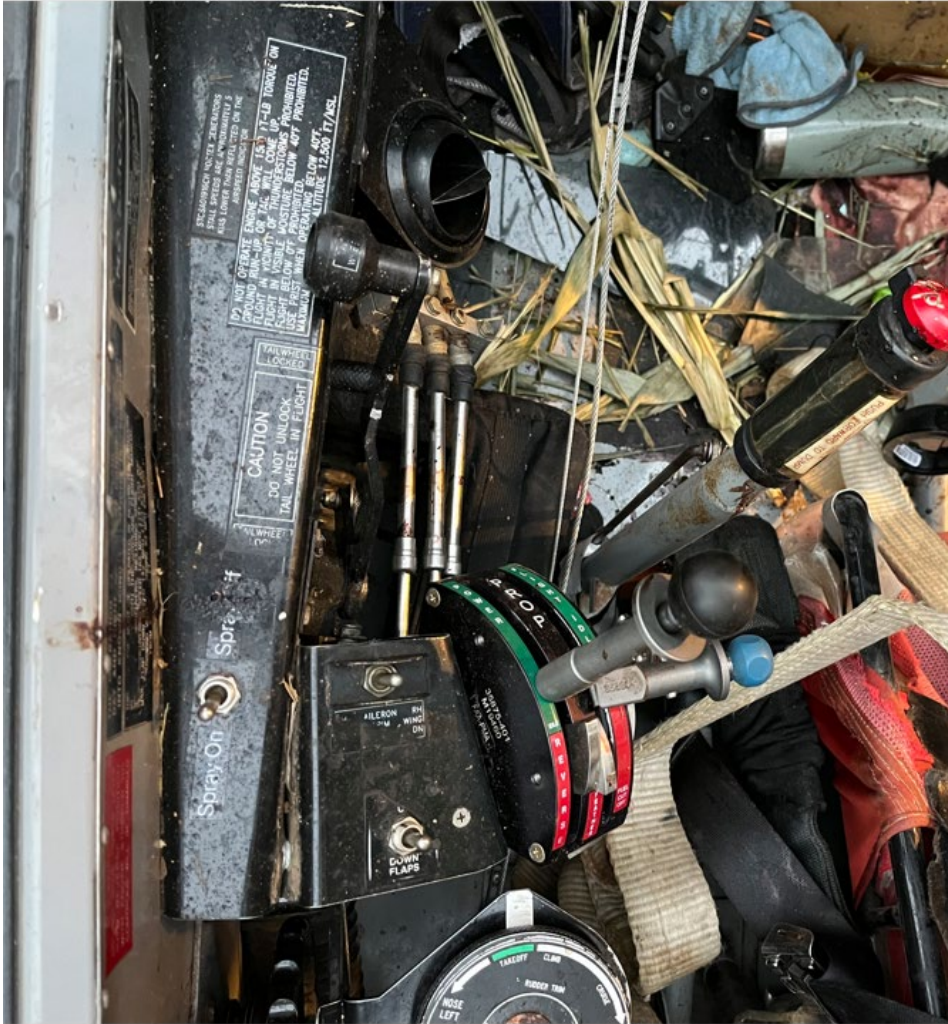
Figure 12 Engine controls as found on site.
