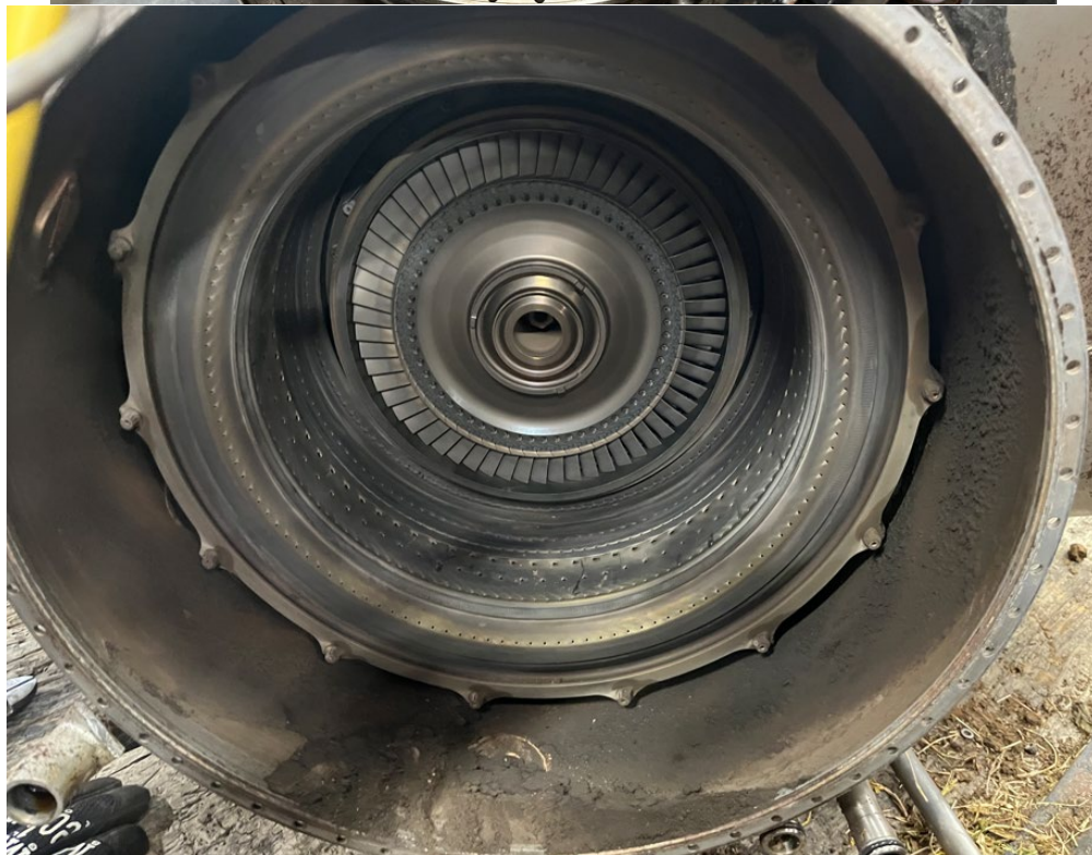
Figure 19 Split open engine and turbines during exam.
