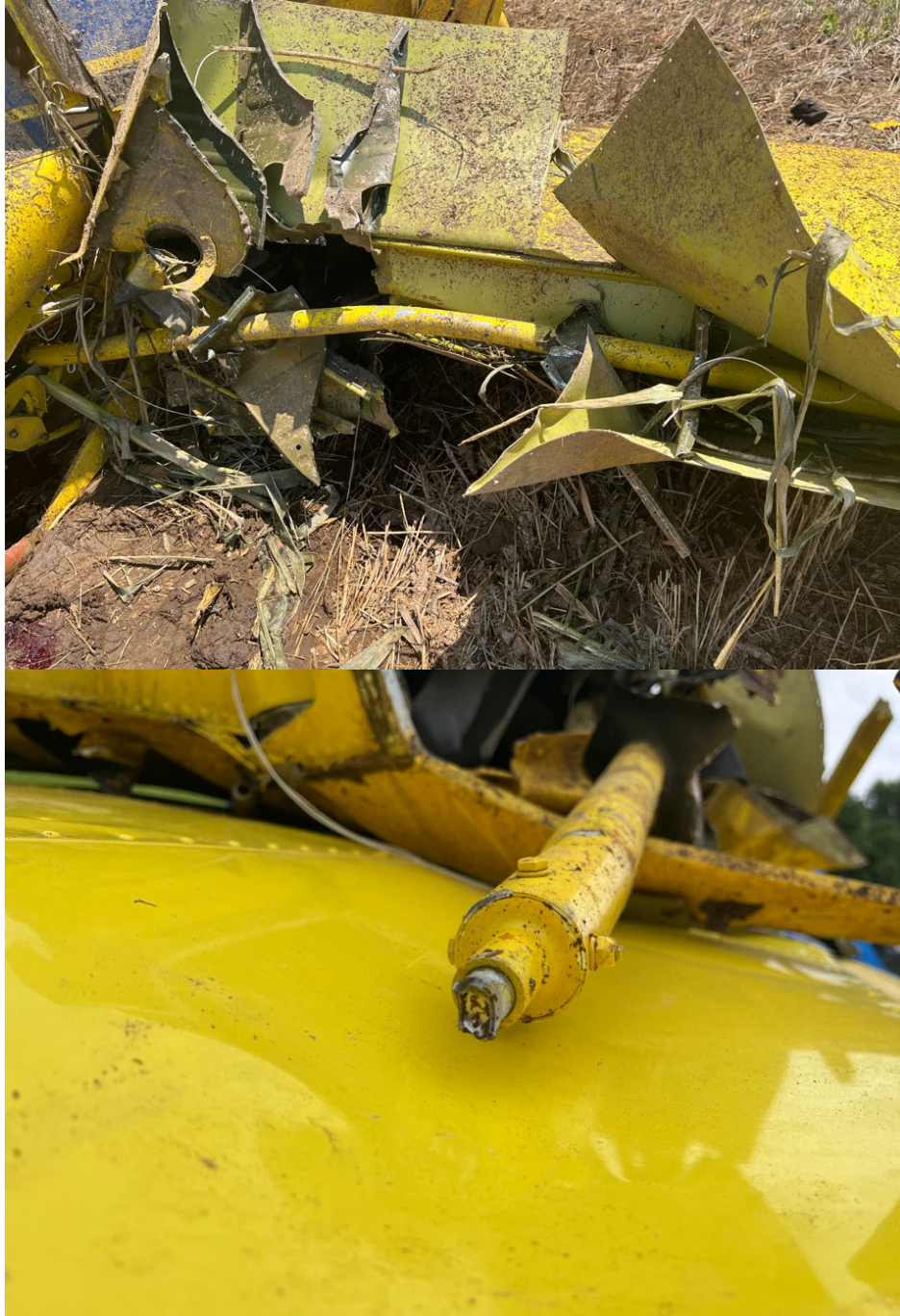
Figure 8 Wing damage and control rod overload damage.
