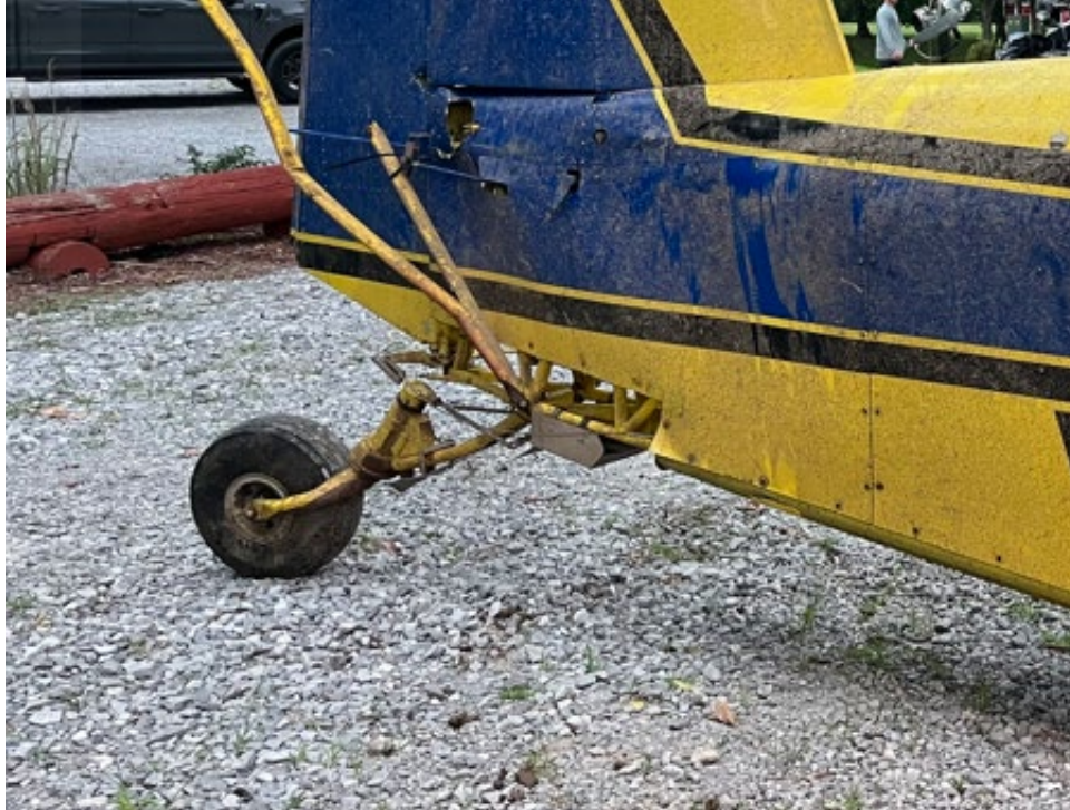
Figure 10 Airframe damage pic (above) with tail wheel (lower)
