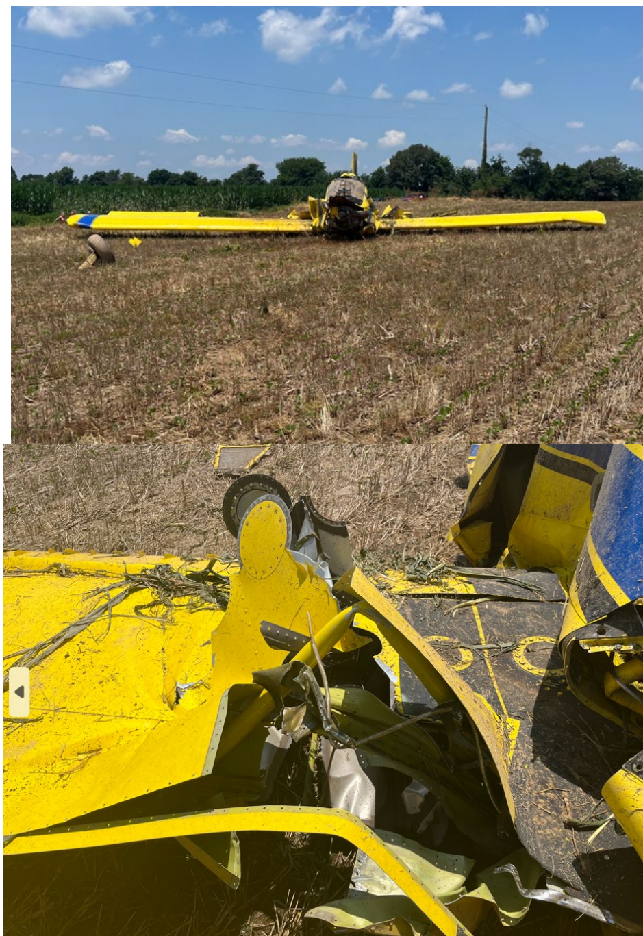
Figure 7 Front view of wreckage (above) and wing damage (lower)
