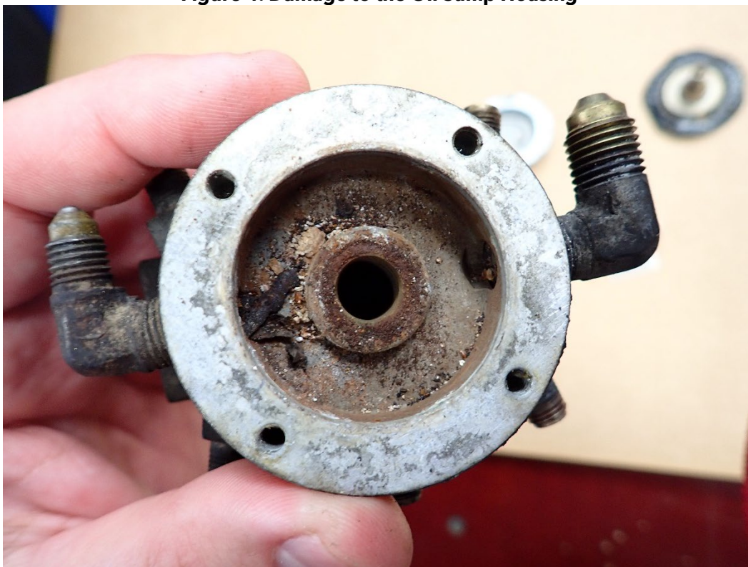
Figure 5: Debris Found Within the Fuel Manifold
