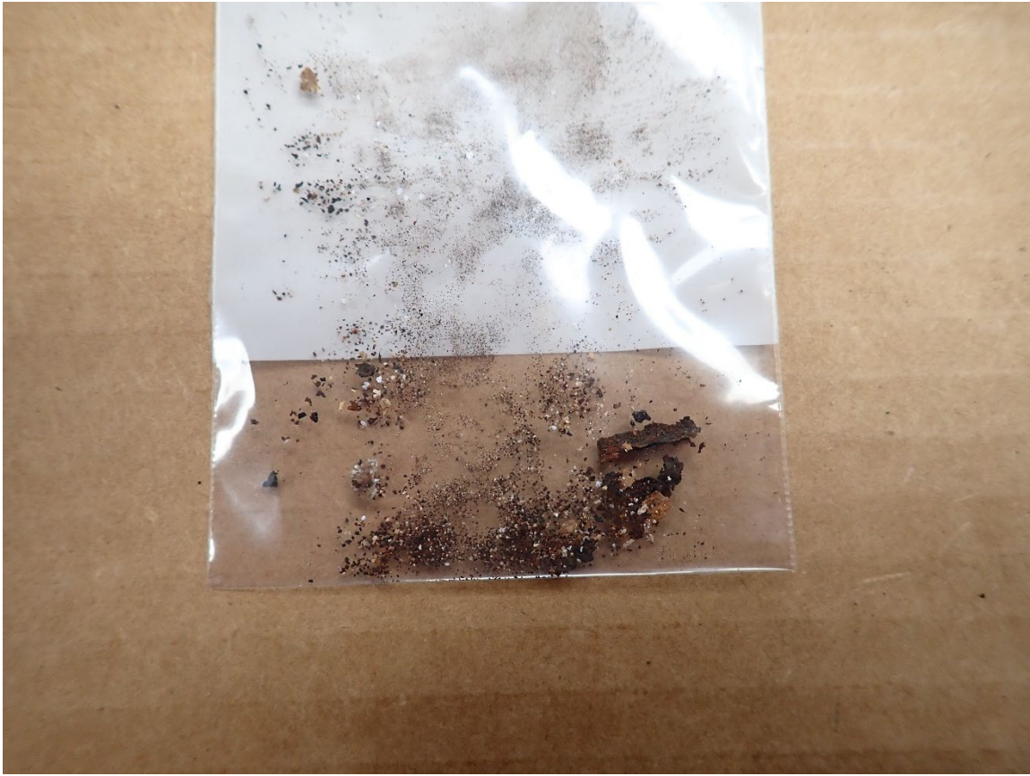
Figure 6: Bagged Debris Removed from the Fuel Manifold
