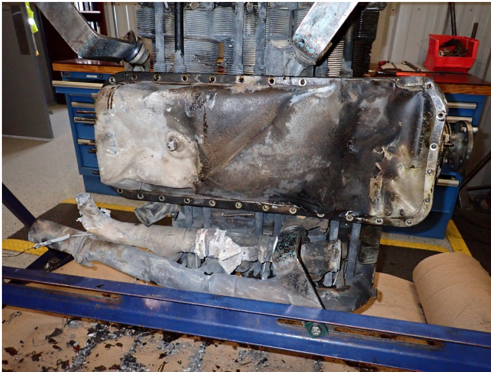
Figure 4: Damage to the Oil Sump Housing
