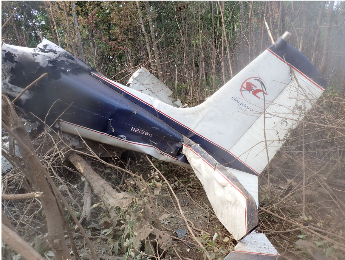
Photograph 3 - Empennage with damaged structure, damaged left horizontal stabilizer and elevator and wrinkling of the vertical stabilizer. (Courtesy of NTSB)
