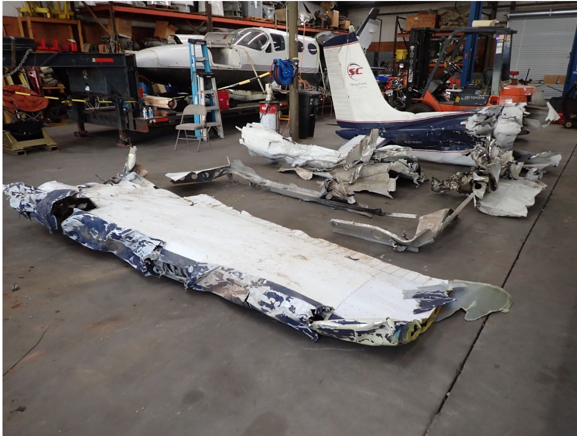
Photograph 4 - Left wing with leading edge, tip and root damage, damaged aileron and crushed flap. (Courtesy of NTSB)
