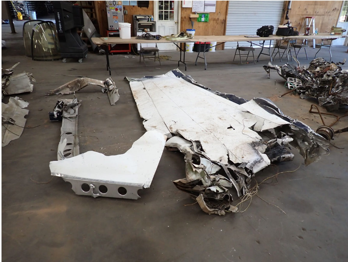
Photograph 5 - Left wing with leading edge, tip and root damage, damaged aileron and crushed flap. (Courtesy of NTSB)
