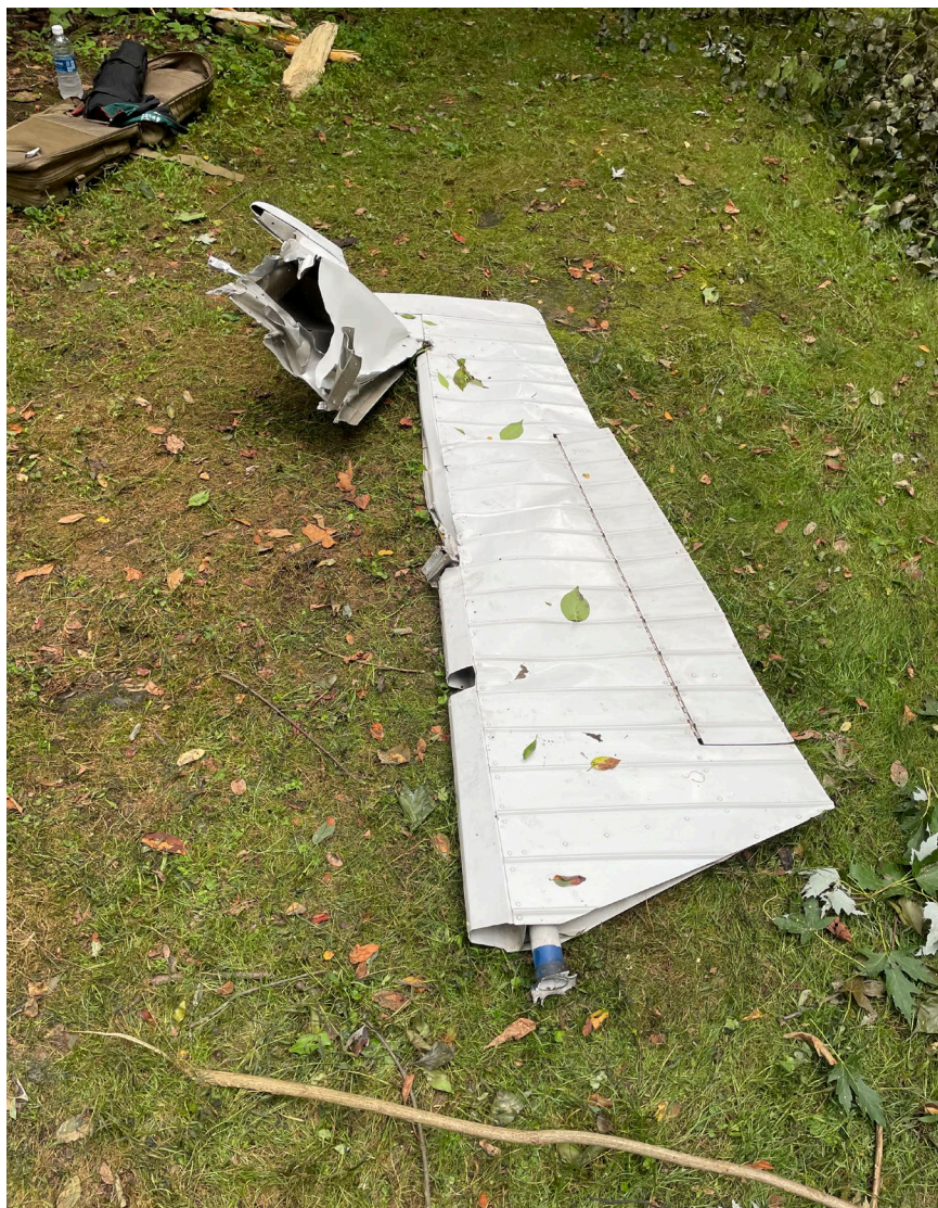
Photograph 6 - Right Elevator (NTSB Photo)
