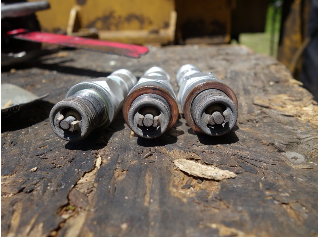
Photo 36: View of the Nos. 2, 4, and 6 bottom spark plugs.
