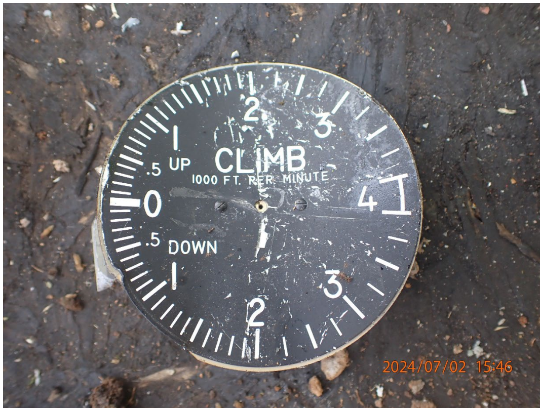
Photo 23: View of the vertical speed indicator with slap mark.
