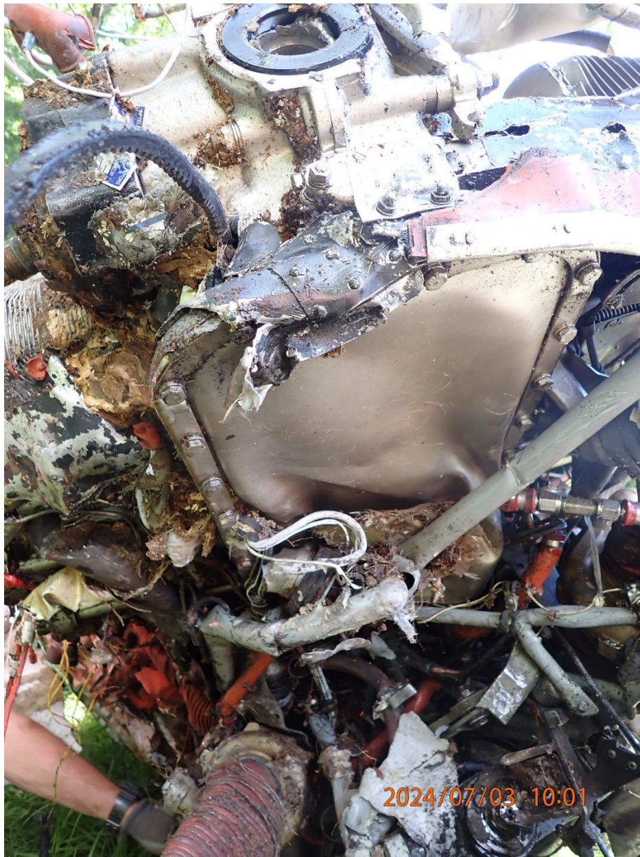
Photo 37: View of the impact crushed oil pan.
