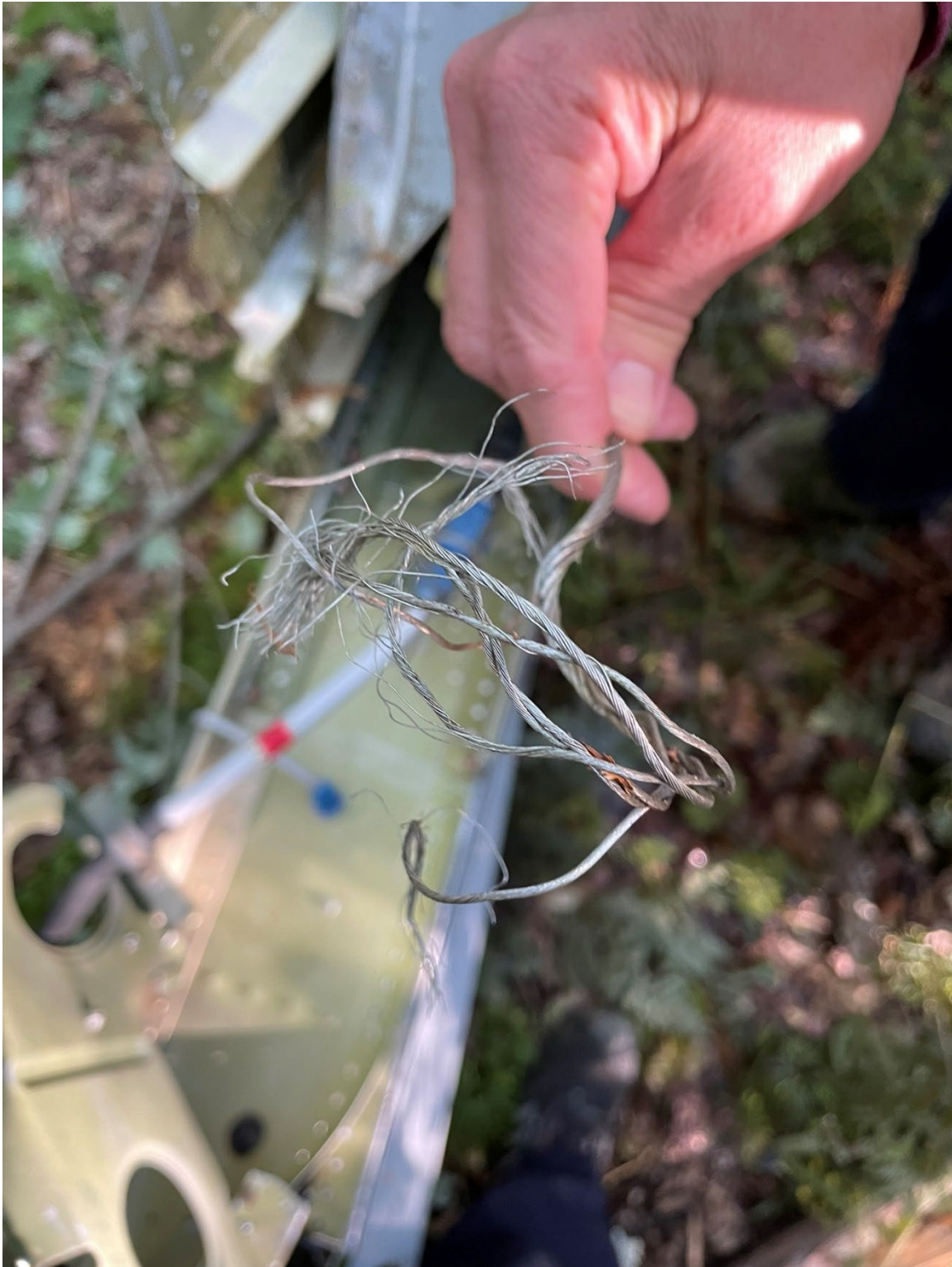
Photo 20: Broomstick of the right aileron drive cable.
