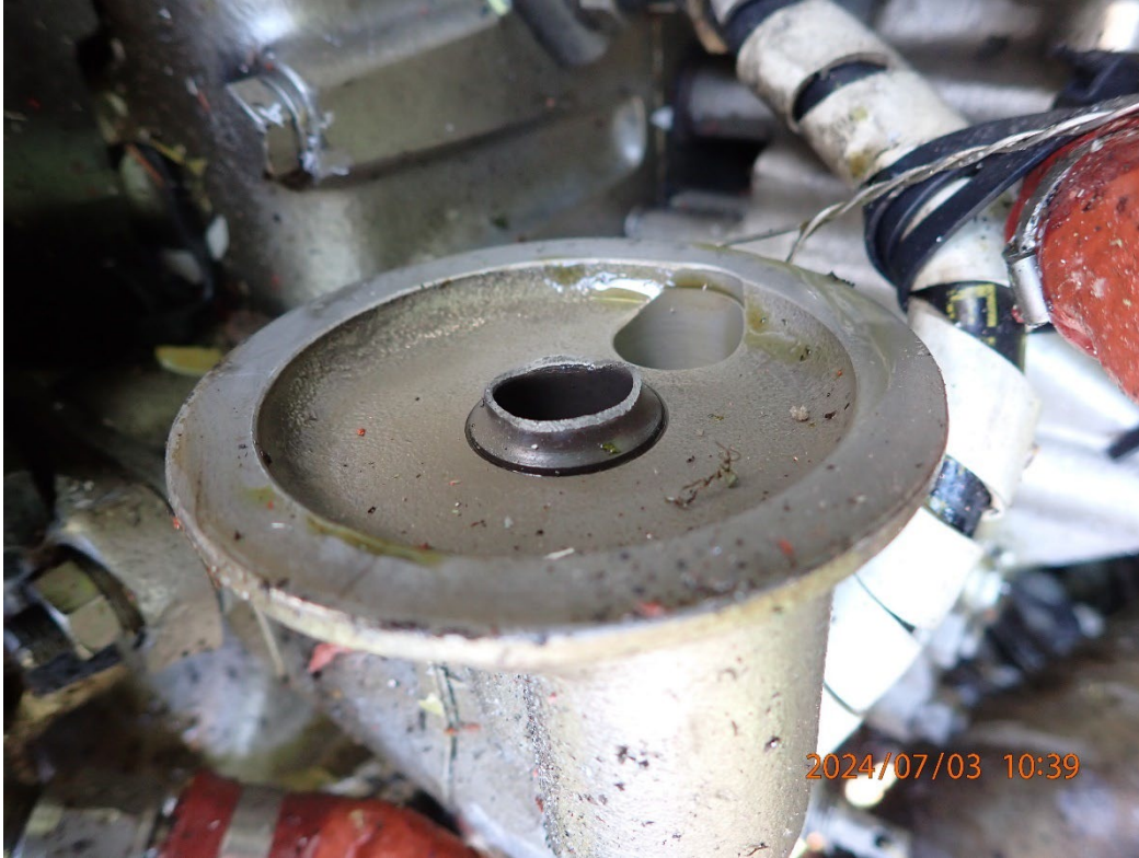
Photo 40: View of the impact fractured oil filter neck.
