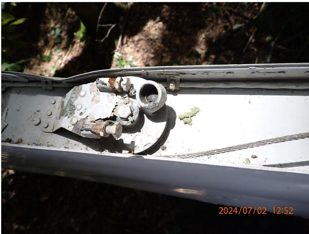
Photo 11: Left aileron sector with balance cable attached.
