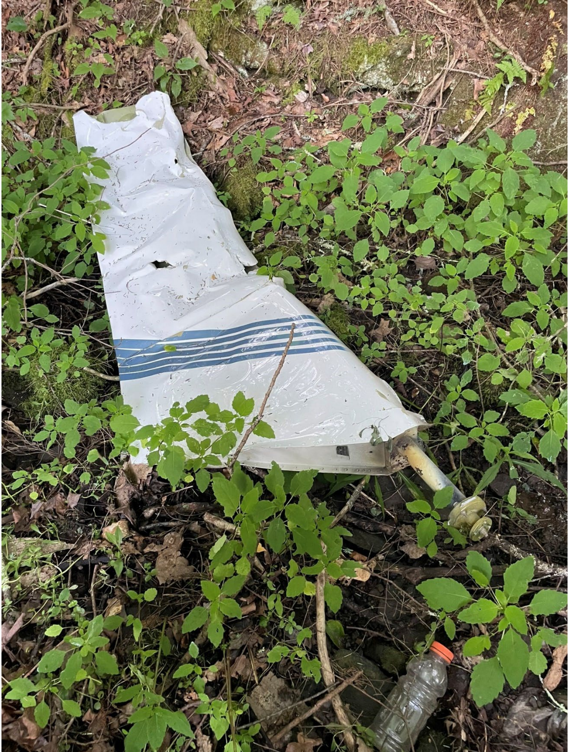
Photo 6: View of the rudder found after the investigative team departed. (Photo courtesy of Trout Creek Fire Department)
