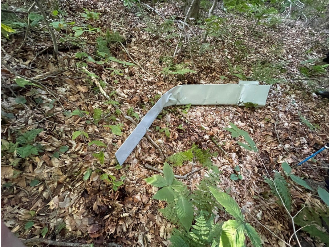
Photo 21: View of the right aileron as found.
