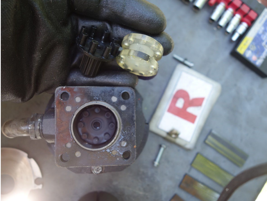
Photo 43: View of the right vacuum pump drive couplings. (Photo Courtesy of Piper)
