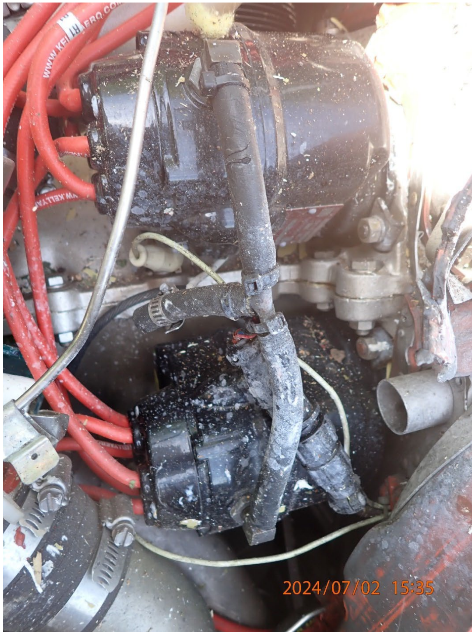
Photo 35: View of the magnetos installed on the engine.
