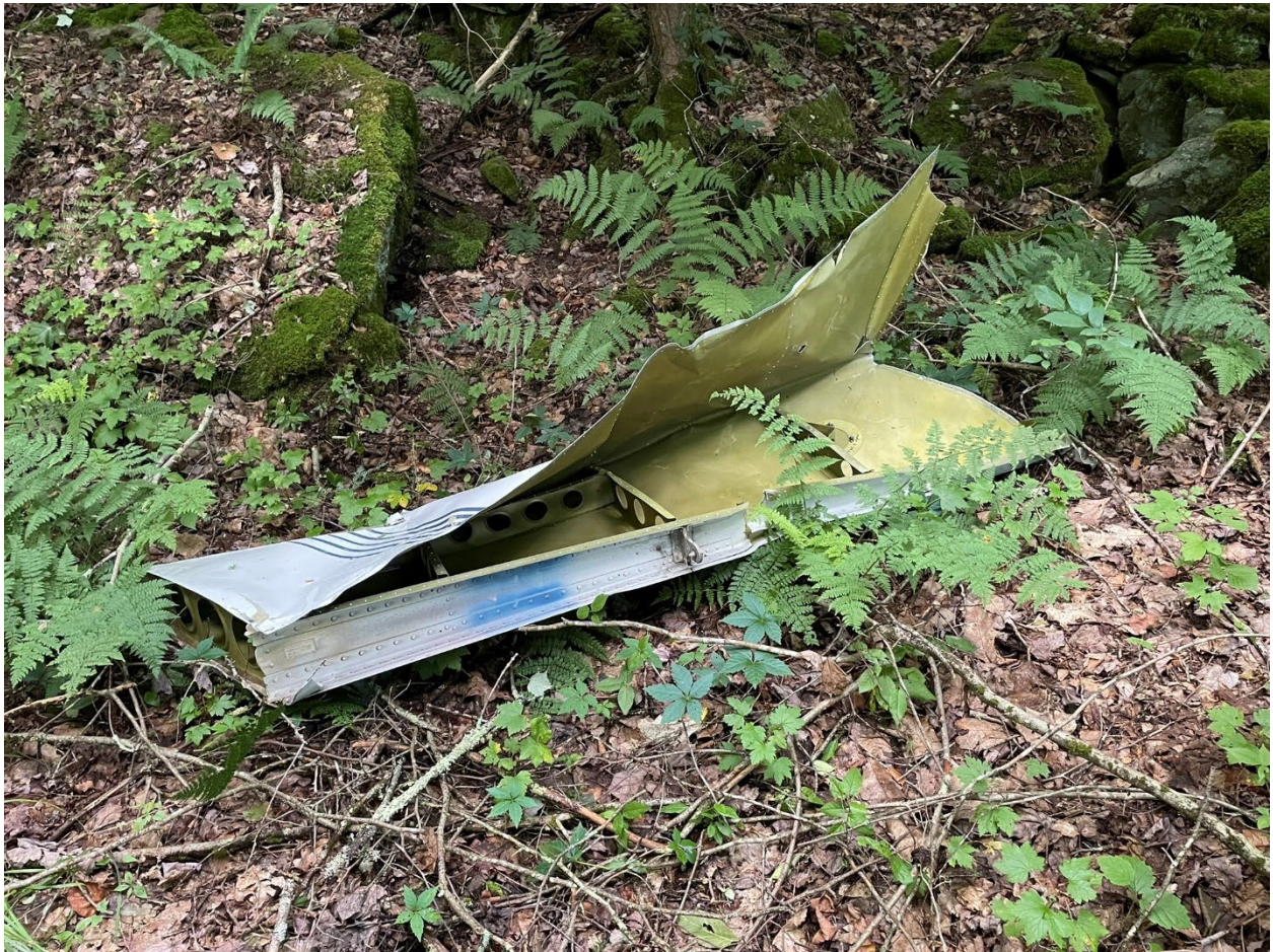
Photo 4: View of the vertical stabilizer as found.
