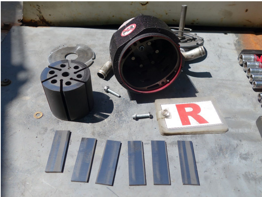
Photo 42: View of the right vacuum pump disassembled. (Photo Courtesy of Piper)
