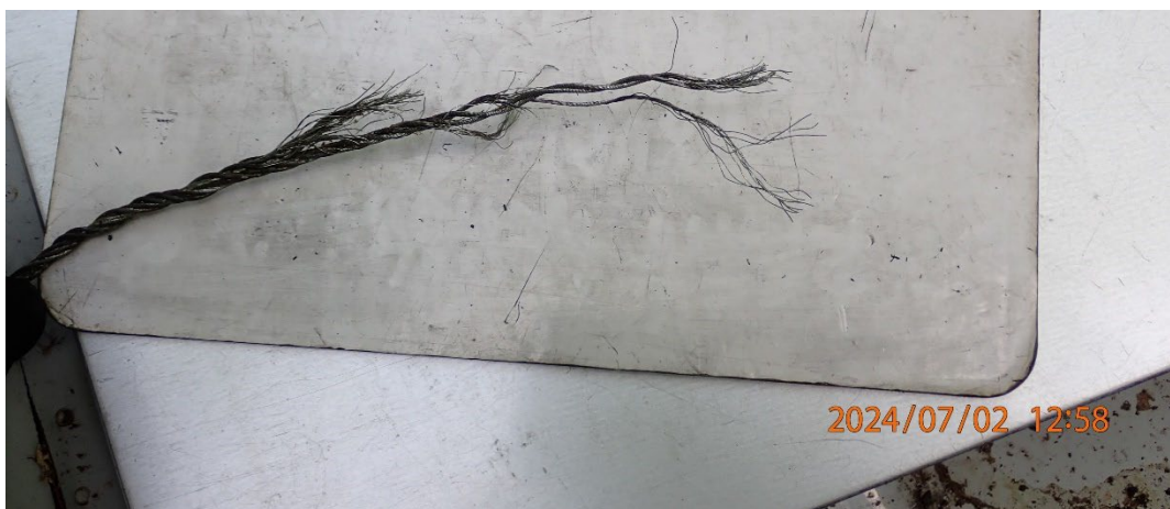
Photo 12: Broomstraw of the left aileron balance cable.
