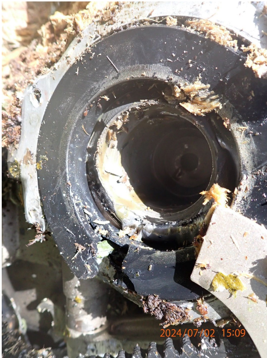
Photo 31: View of the impact fractured engine crankshaft.
