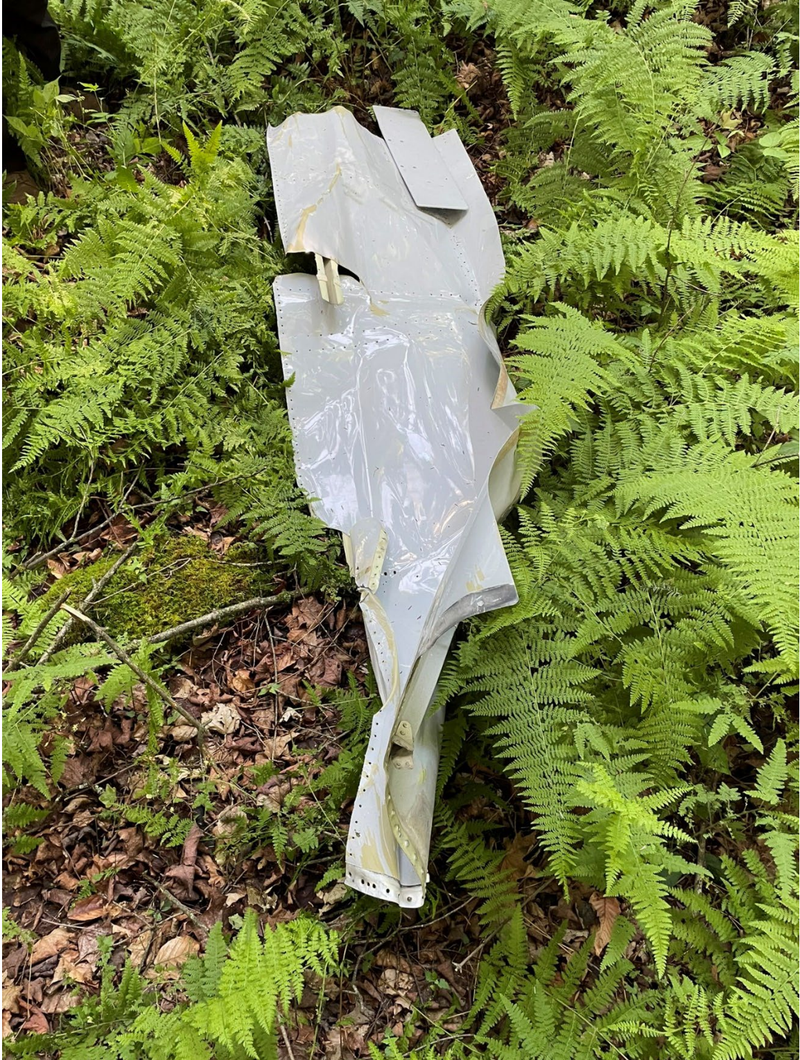
Photo 15: View of right wing skin and right speed brake found in the debris field.
