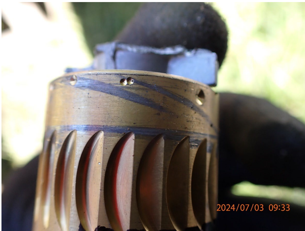
Photo 26: View of rotational scoring on the vacuum driven gyro.
