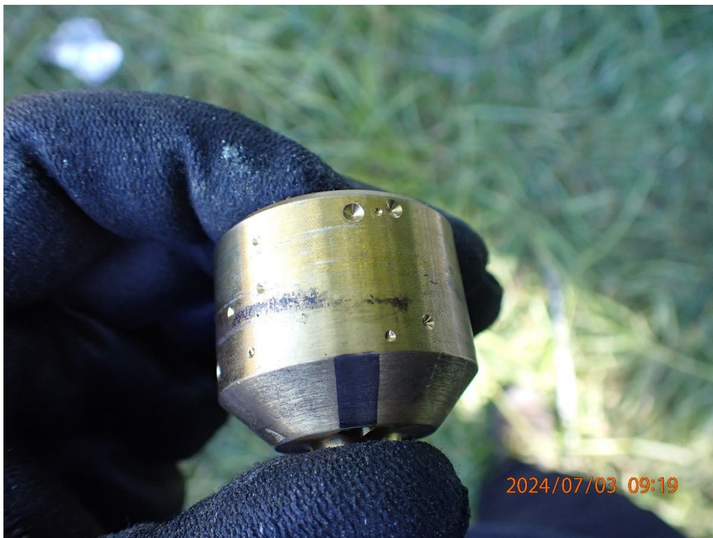
Photo 24: View of rotational scoring on the electric gyro.
