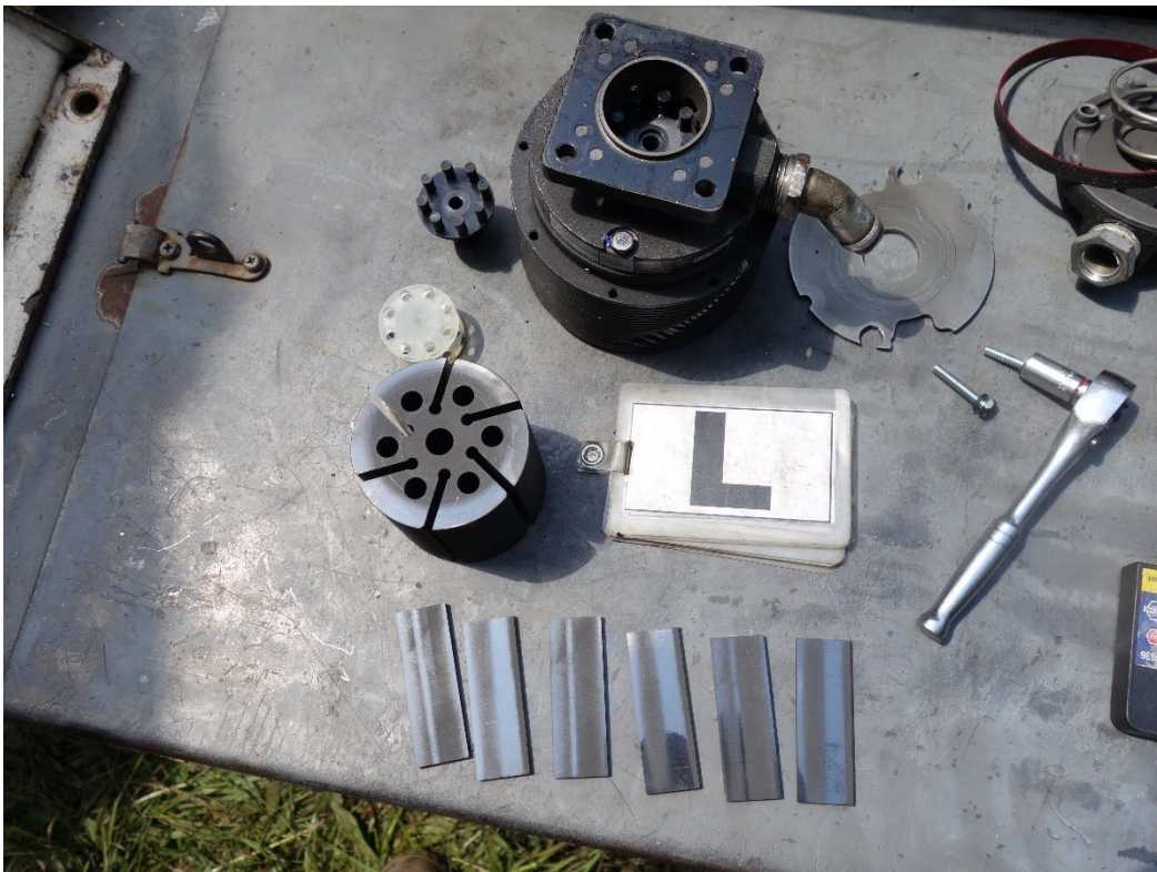
Photo 44: View of the left vacuum pump disassembled. (Photo Courtesy of Piper)
