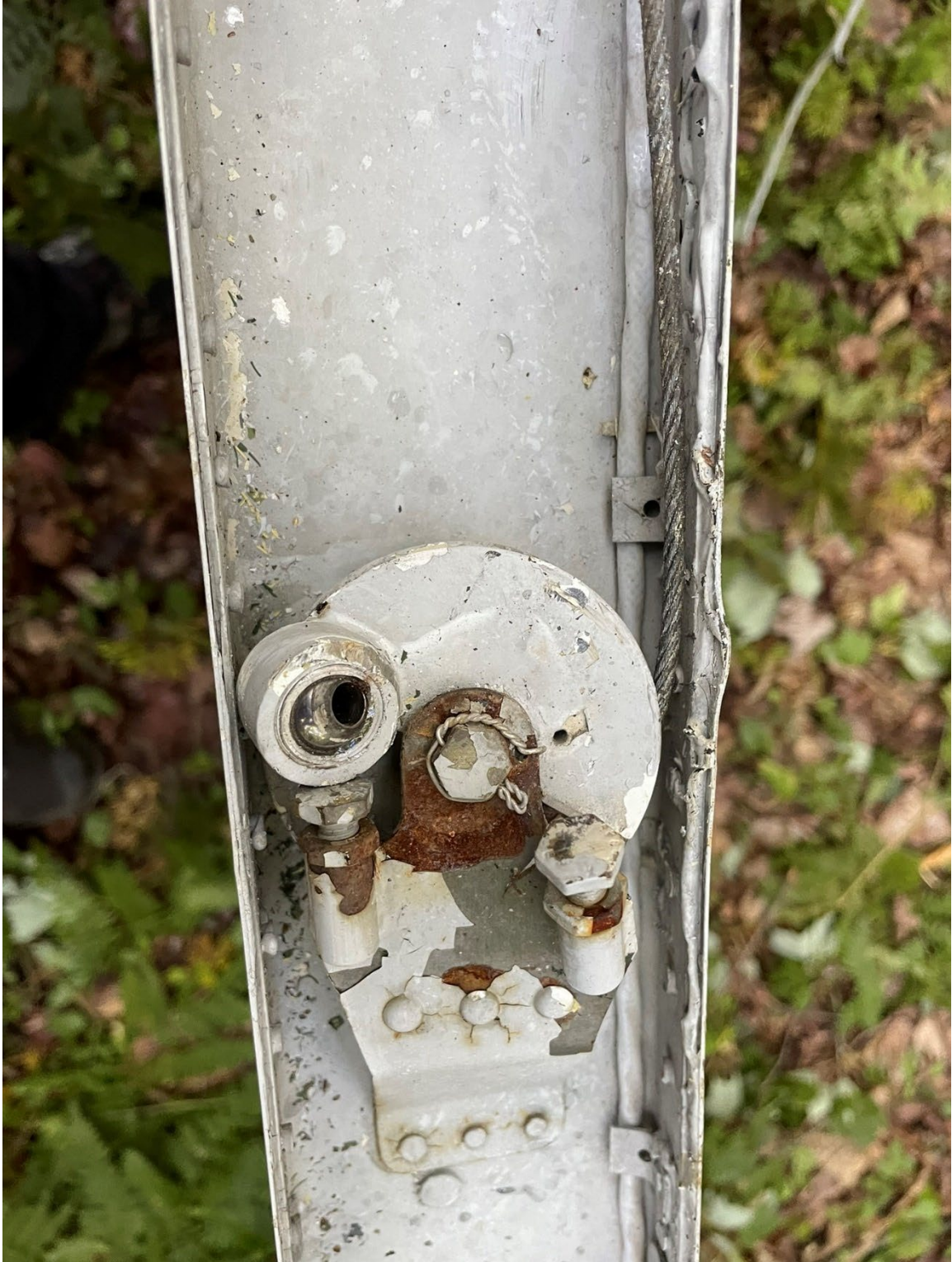
Photo 19: View of right wing sector with right aileron drive cable attached.
