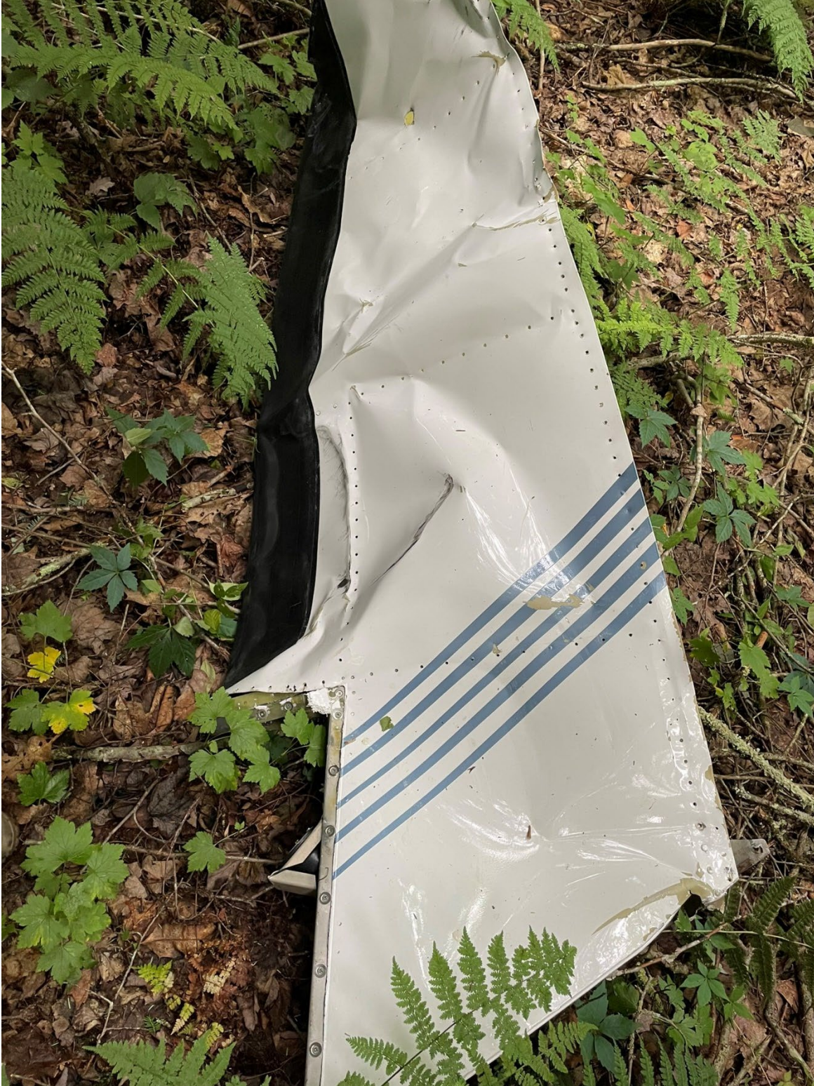
Photo 5: View of the left side of the vertical stabilizer.
