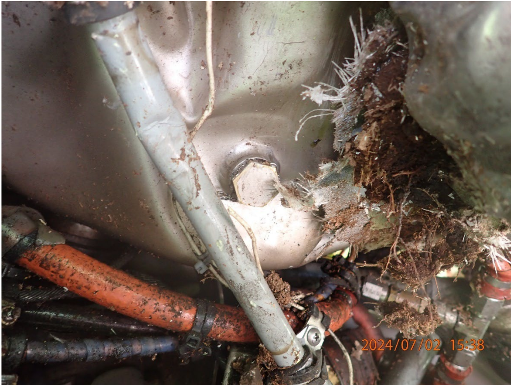
Photo 38: View of the oil drain plug seated in place.
