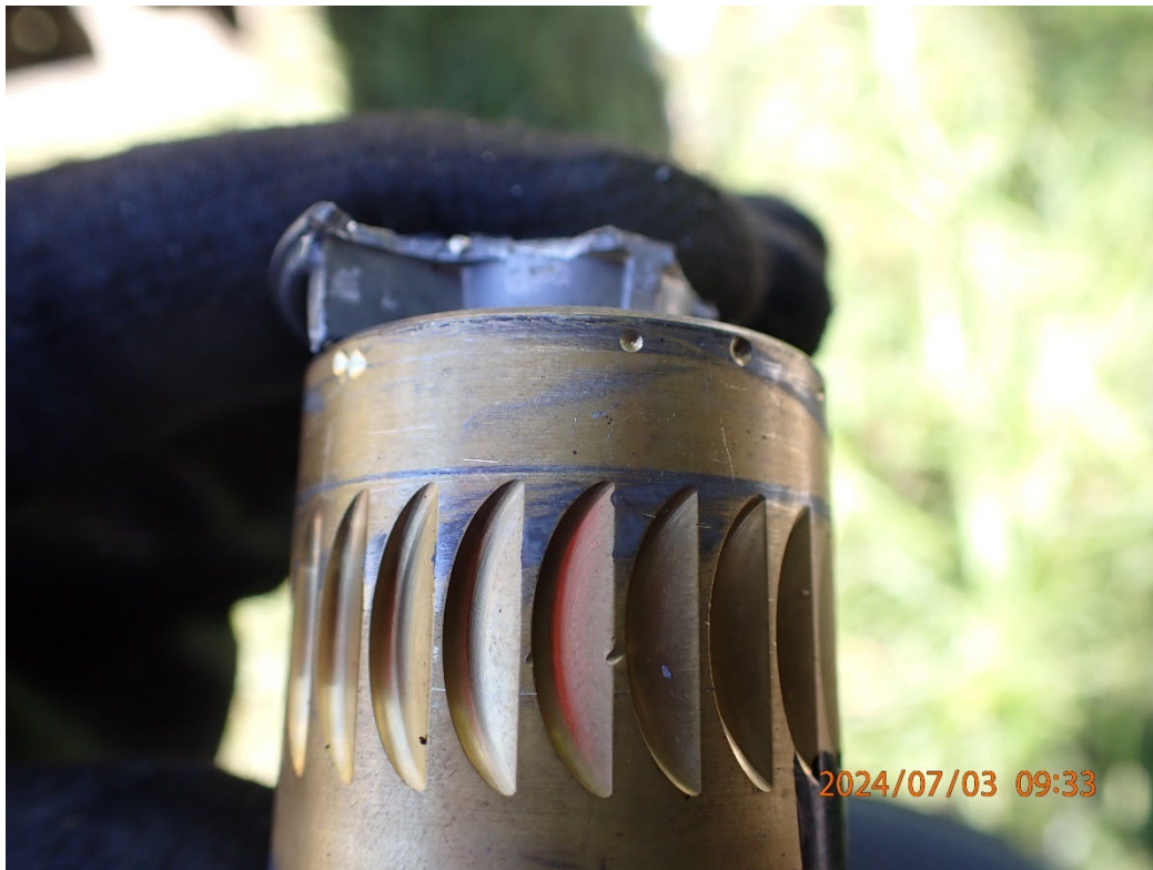
Photo 25: View of rotational scoring on the vacuum driven gyro.
