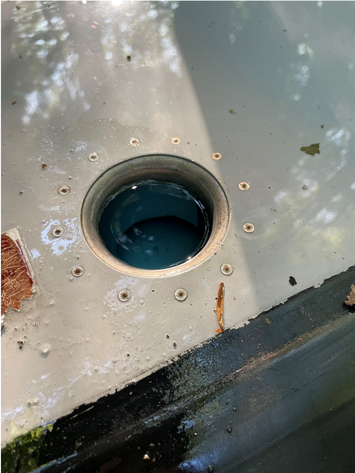
Photo 17: View of fuel remaining in the right wing.
