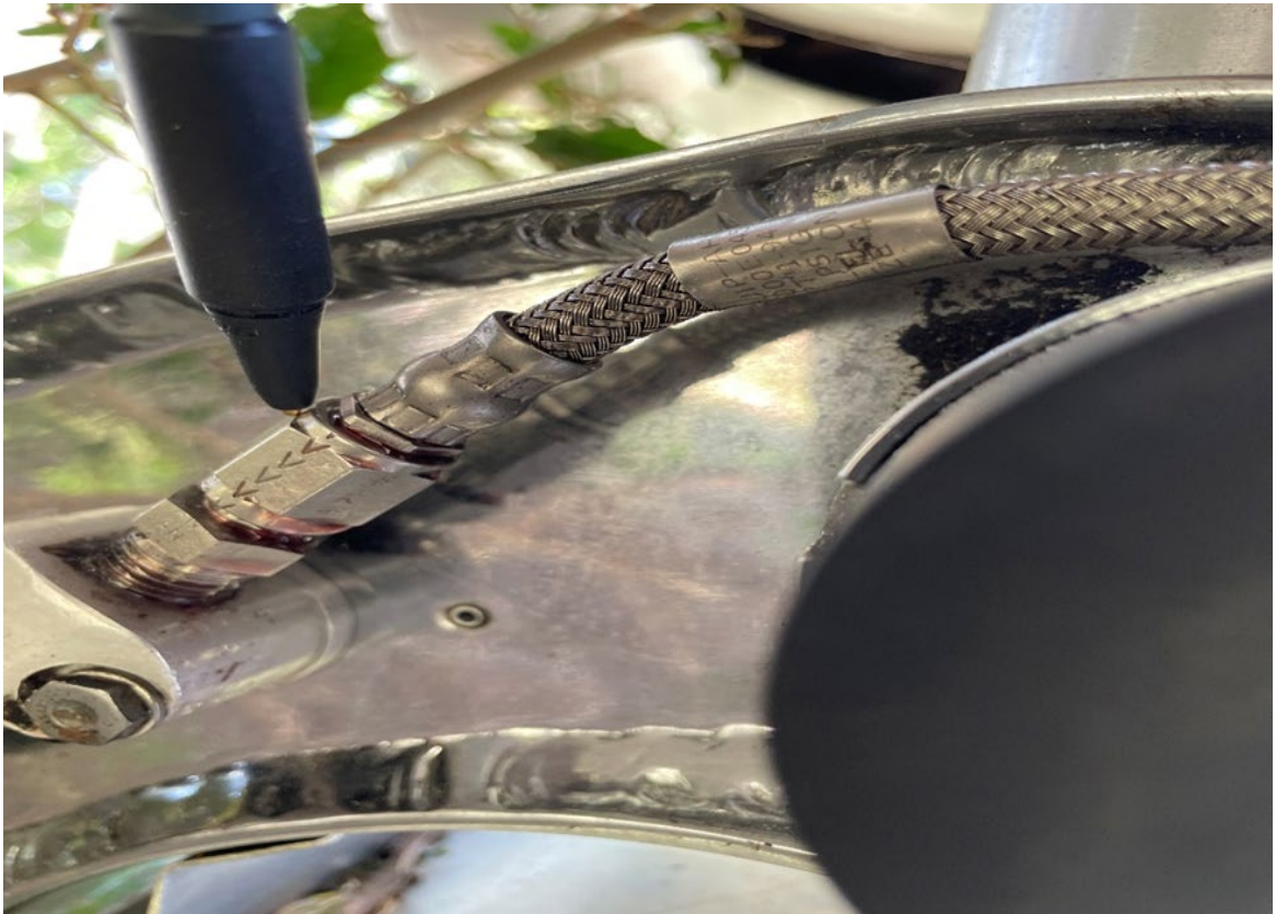
Figure 4. Hydraulic fluid was observed “leaking” around the right-side B-Nut fitting.
