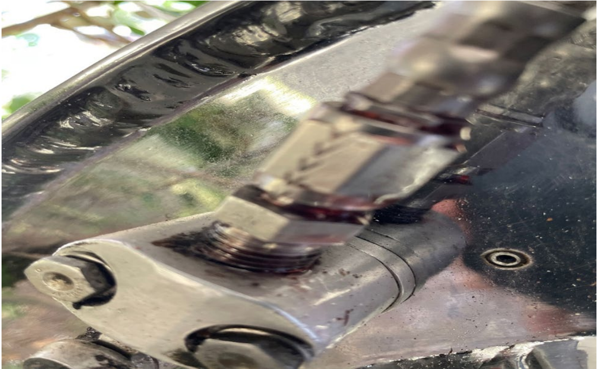
Figure 5. Right-side loose B-Nut fitting & hydraulic fluid leakage.
