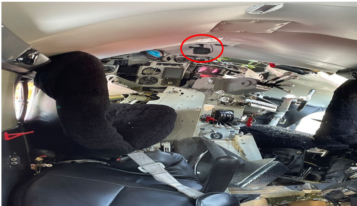
Figure - Cabin interior with mounted GoPro camera circled in red.
