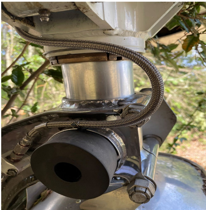
Photograph 5 -View of landing gear strut and brake line.
