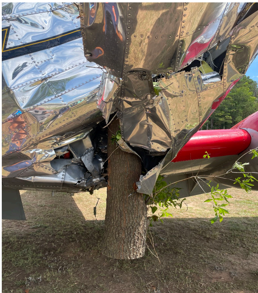
Photograph 6 - View of damaged underside of airplane.
