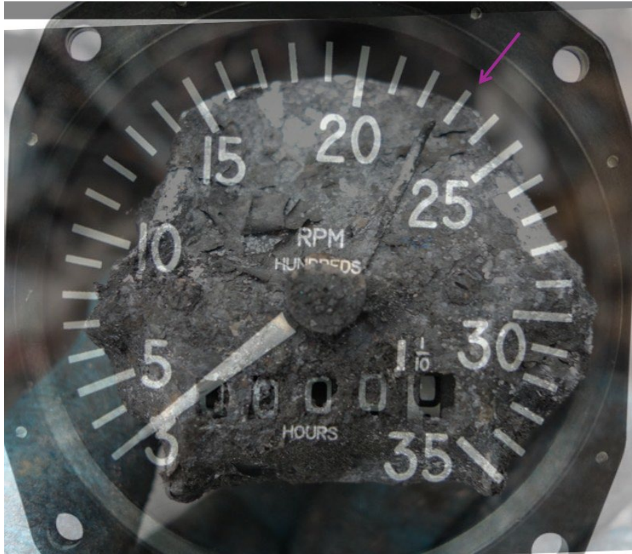
Annotated Piper photograph of the recording tachometer with transparent overlaid photograph of similar make/model tachometer. (NTSB)
