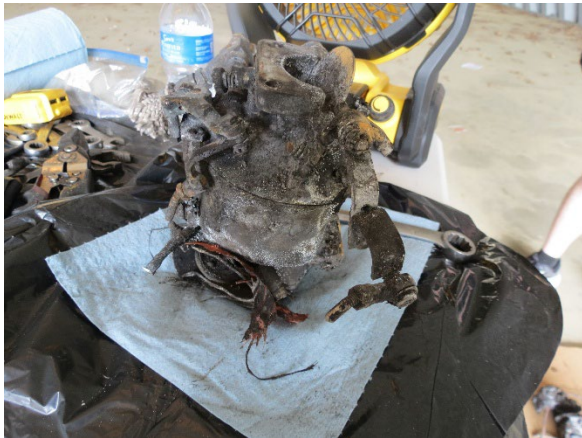
Photograph of carburetor. (Courtesy of Lycoming)
