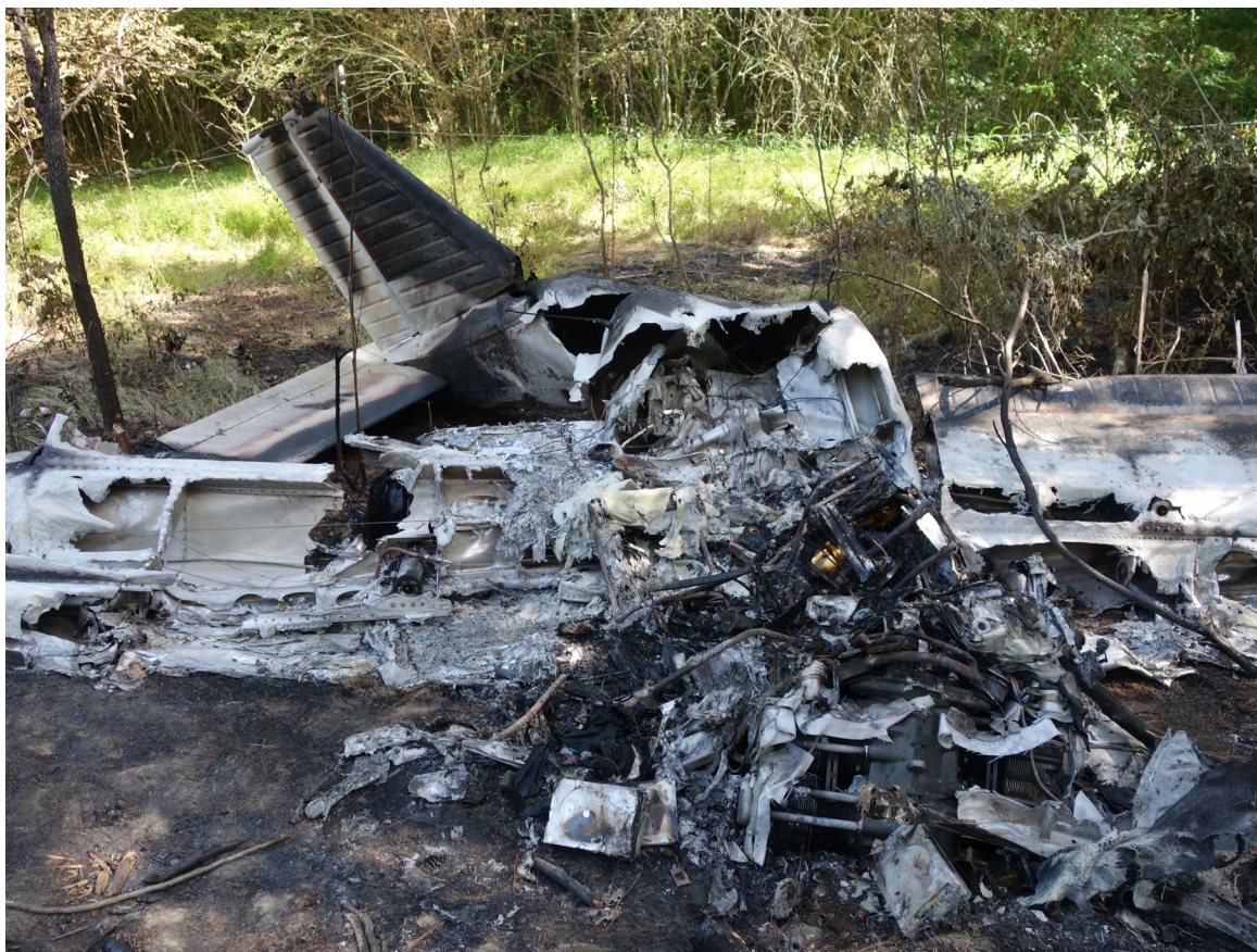
Photograph 2 - Impact and thermal damage noted to fuselage. (Courtesy of Piper Aircraft)
