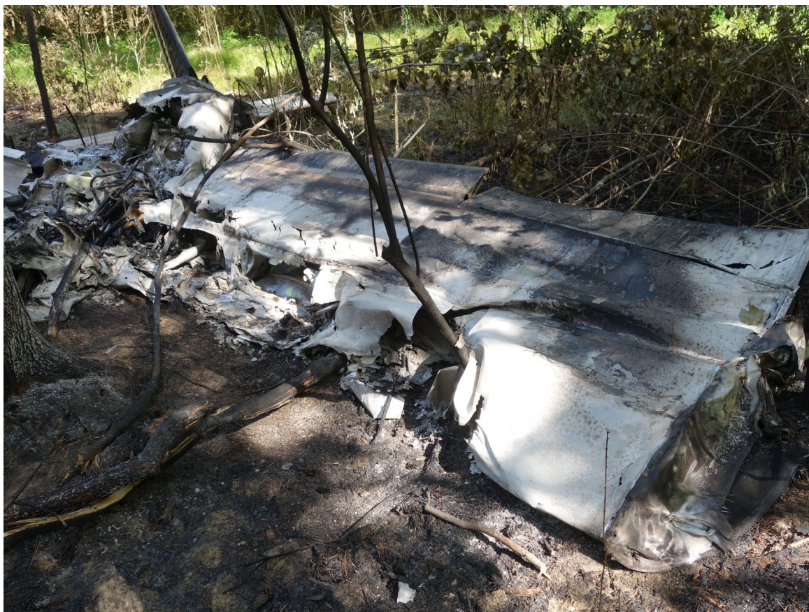
Photograph 4 - Impact and thermal damage noted to left wing. (Courtesy of Piper Aircraft)
