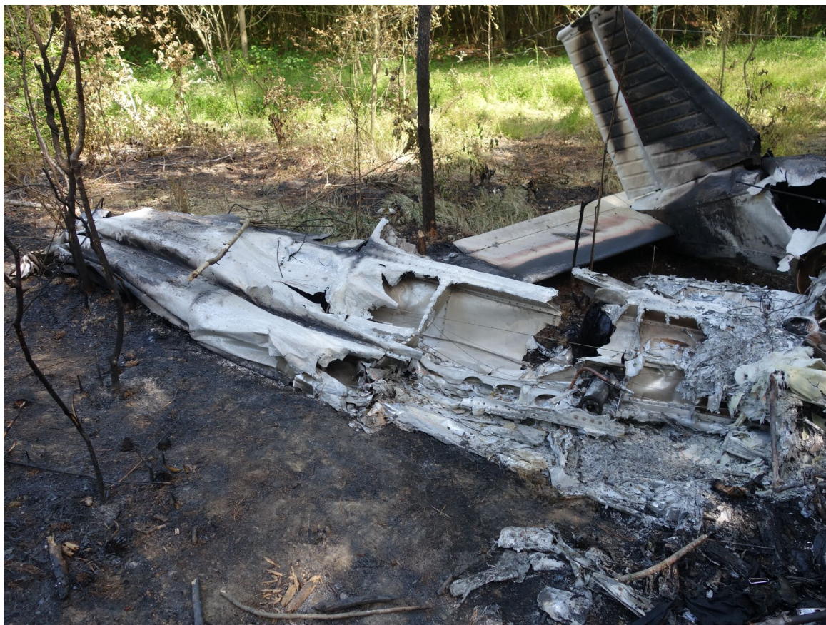
Photograph 3 - Impact and thermal damage noted to right wing. (Courtesy of Piper Aircraft)
