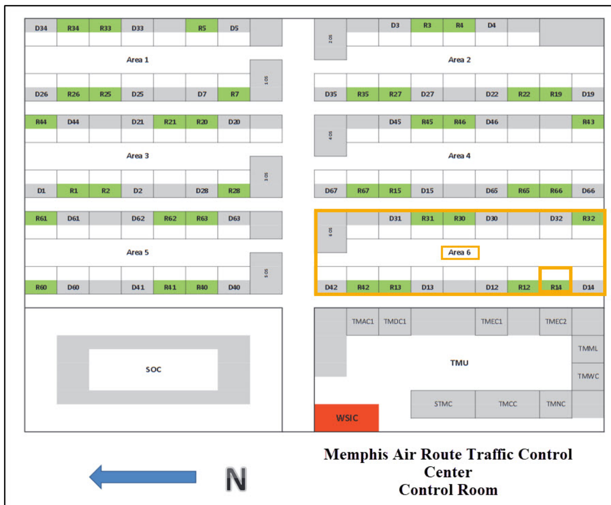
Figure 13. ZME ARTCC control room layout.
