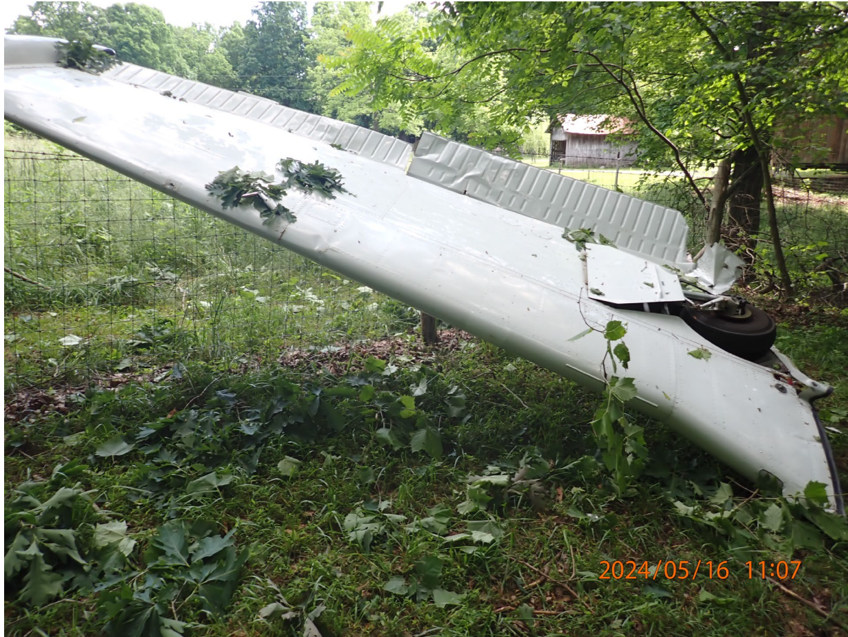
Photograph 4 - View of separated left wing resting against fence. (NTSB)
