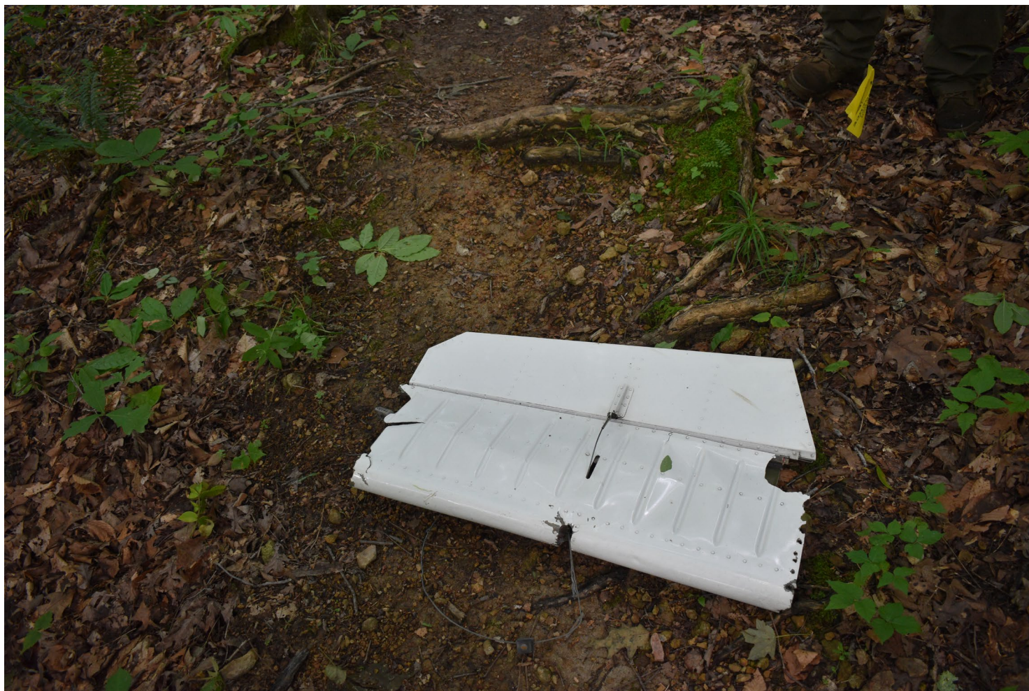
Photograph 7 - Elevator-rudder (ruddervator) located at beginning of wreckage path. (NTSB)
