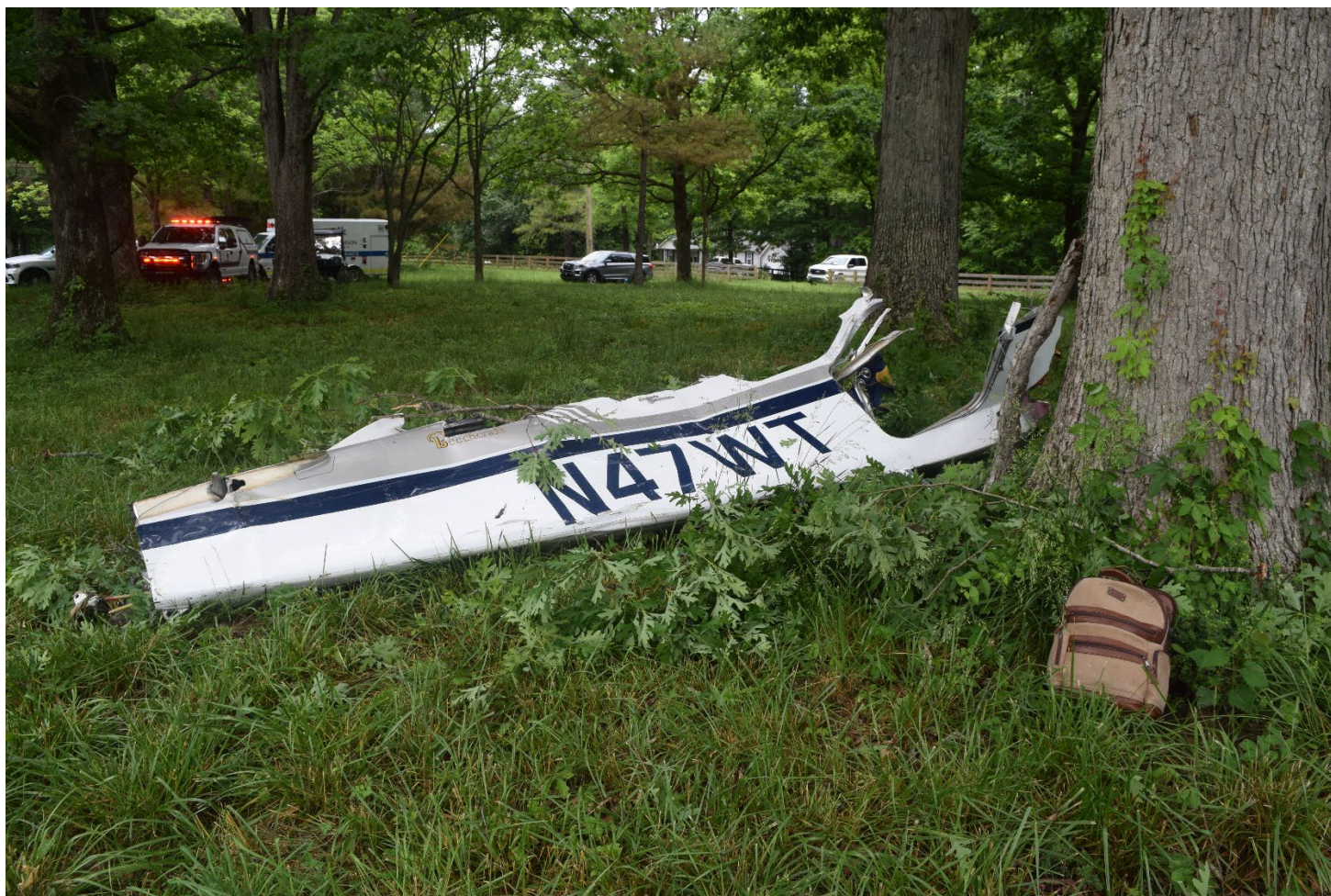
Photograph 2 - View of partial cabin/fuselage against tree. (NTSB)
