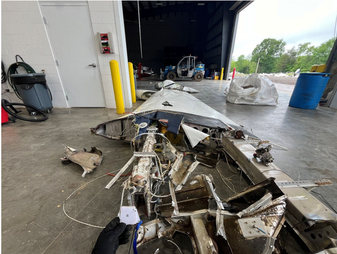
Photograph 11 - View of right wing and spar looking outboard. (NTSB)
