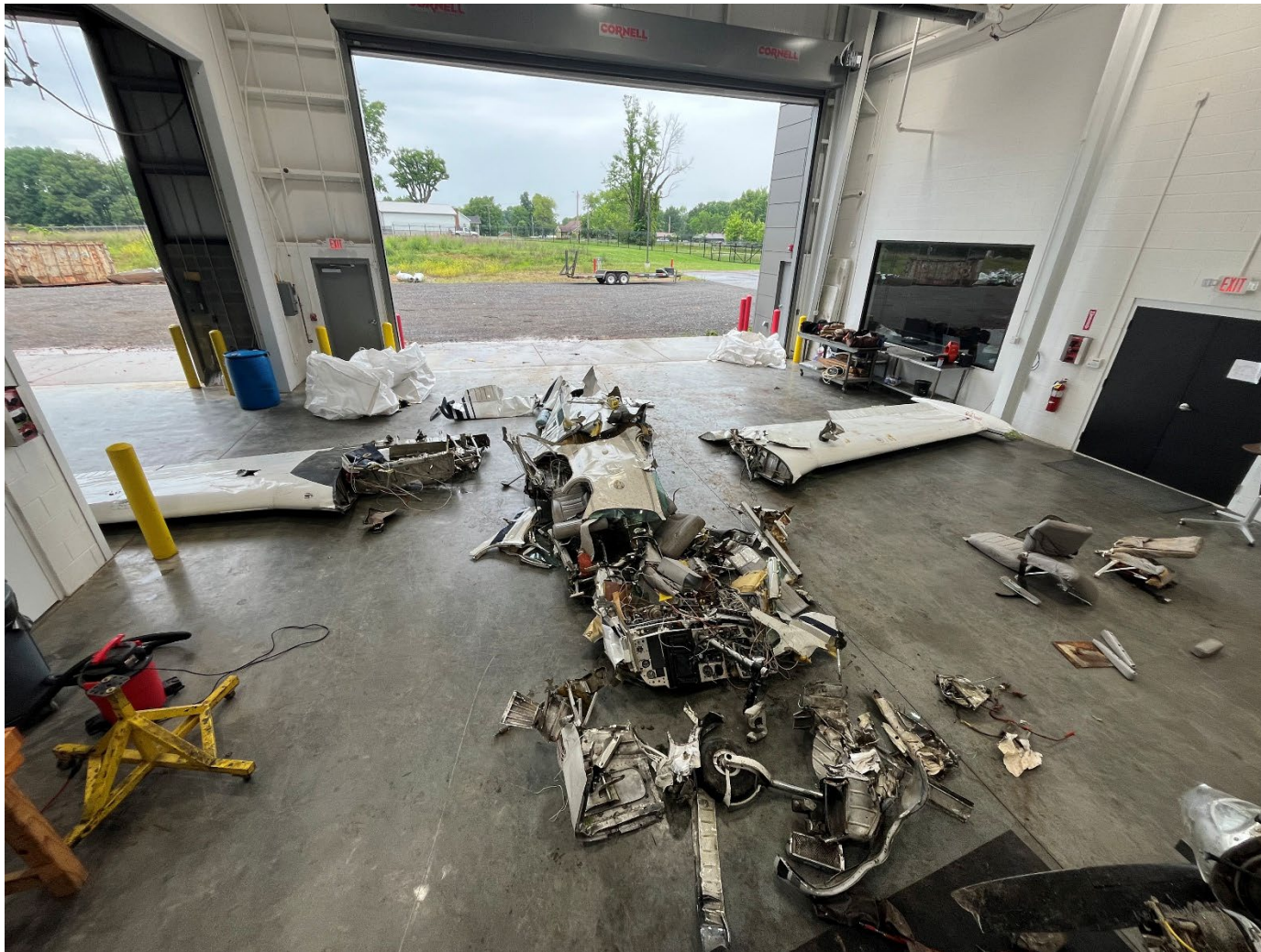
Photograph 8 - Recovered wreckage layout on hangar floor. (NTSB)
