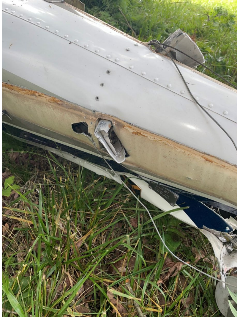
Photograph 9 - View of stabilator spar showing preimpact deformation damage. (NTSB)
