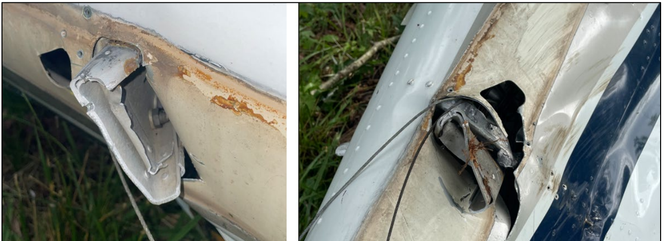
Figure 6 Closeup of stabilizer damage at the fuselage.
