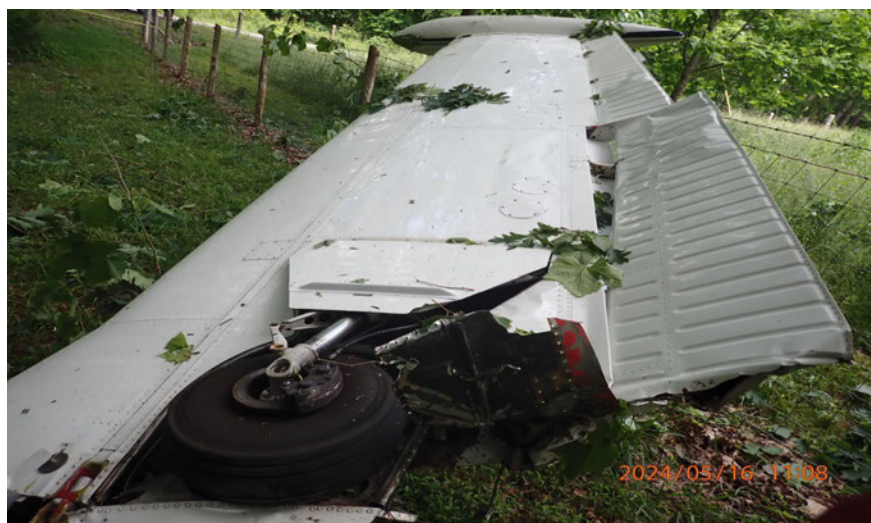
Figure 7 Left wing as observed on site.
