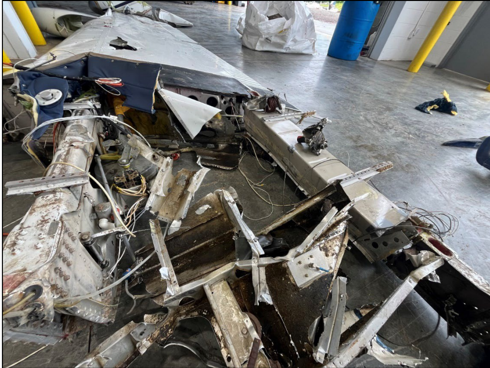
Figure 13 Right wing spar and aft spar structure at examination site.
