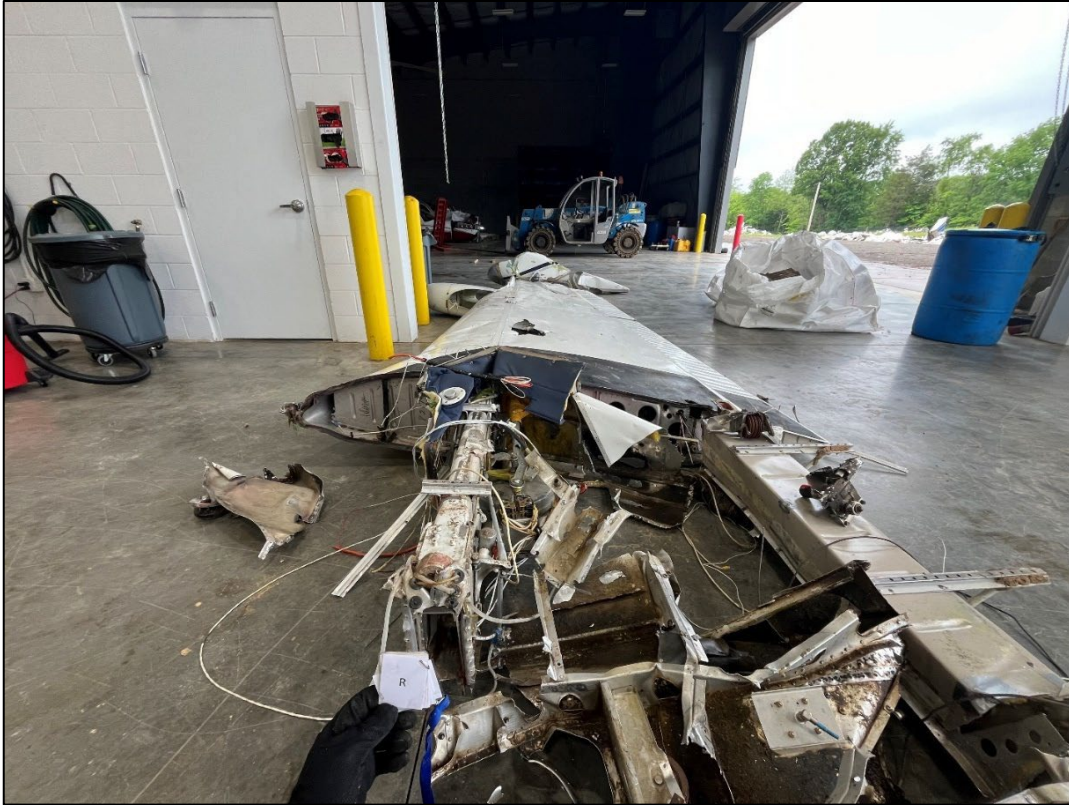
Figure 16 Right wing overview.
