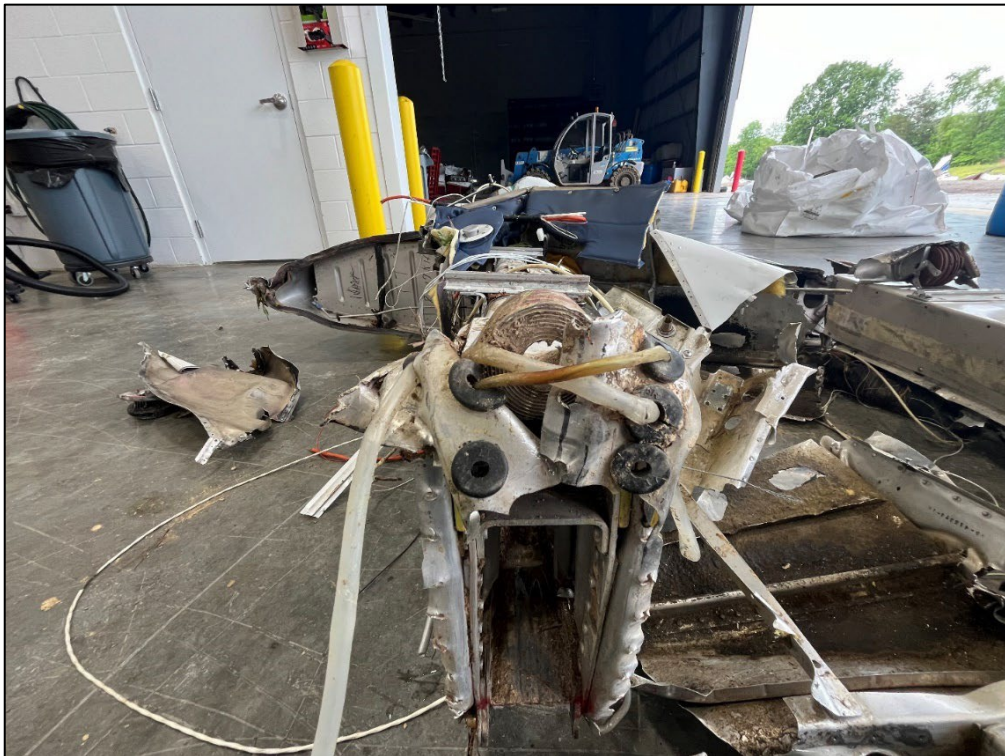
Figure 14 Right wing forward spar fracture surface.
