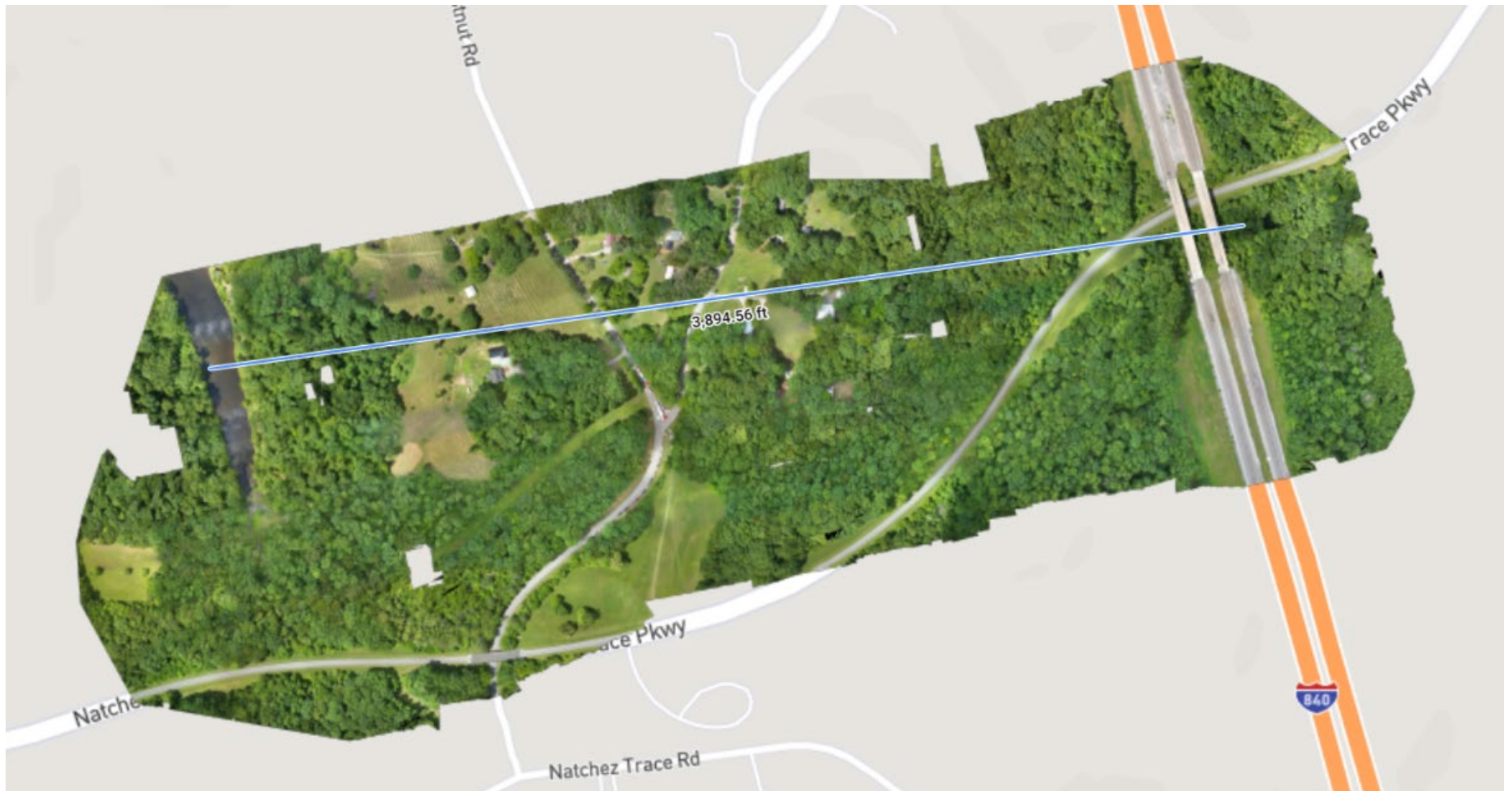
Figure 2. Orthomosaic overlay on Google Earth with debris field (area of initial and final debris) measurement.
