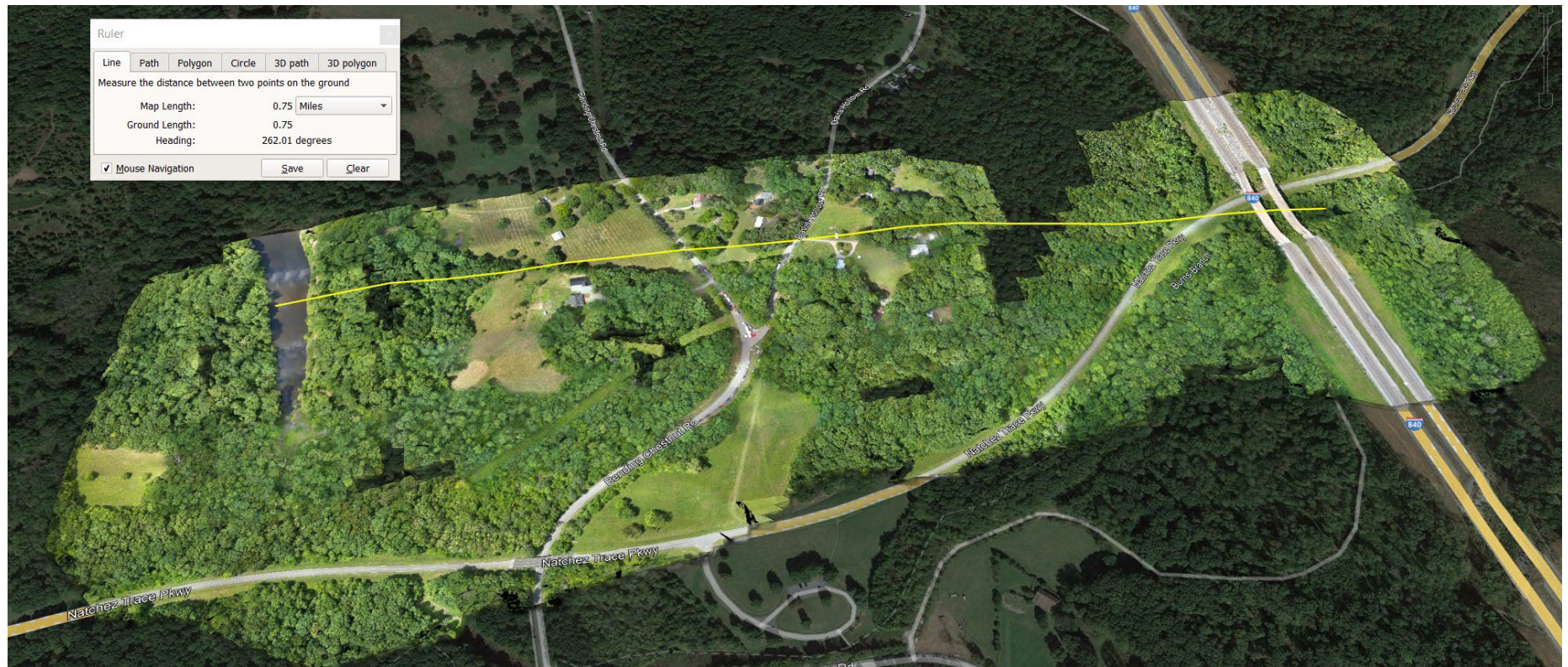
Figure 3. Orthomosaic overlay on Google Earth with debris field measurement (area of initial and final debris) and heading.
