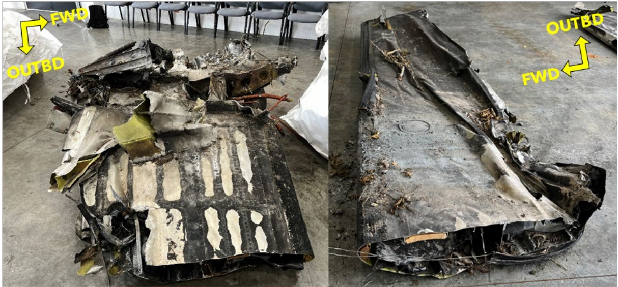
Figure 6. Left Wing Damage (lower surface) inboard (left) outboard (right) (NTSB Photo)
