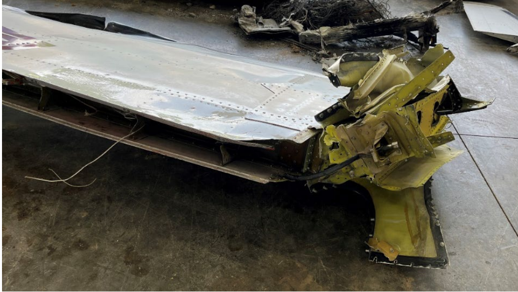
Figure 11. Vertical Stabilizer Deformation (NTSB Photo)
