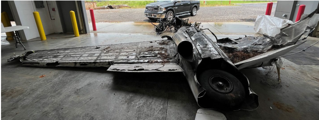
Figure 3. Right Wing Damage (aft looking forward at lower surface) (NTSB photo)
