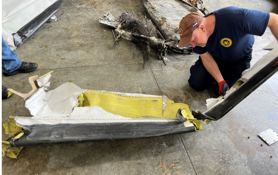
Figure 9. Left Stabilizer Deformation (NTSB Photo)
