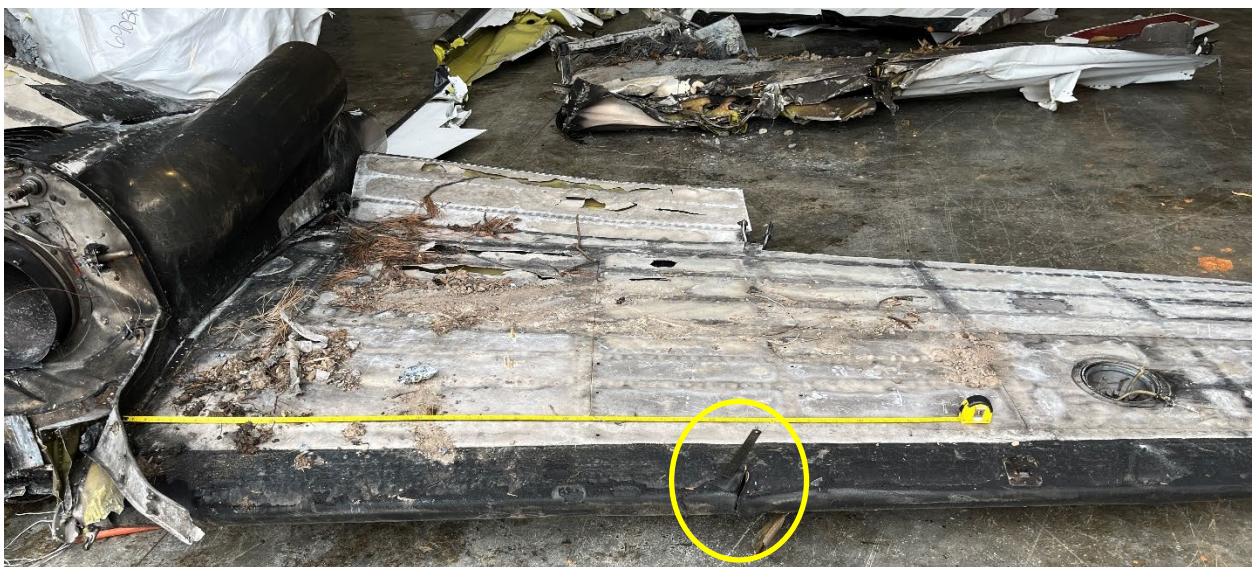
Figure 4. Right Wing Damage (forward looking aft) (NTSB Photo)
