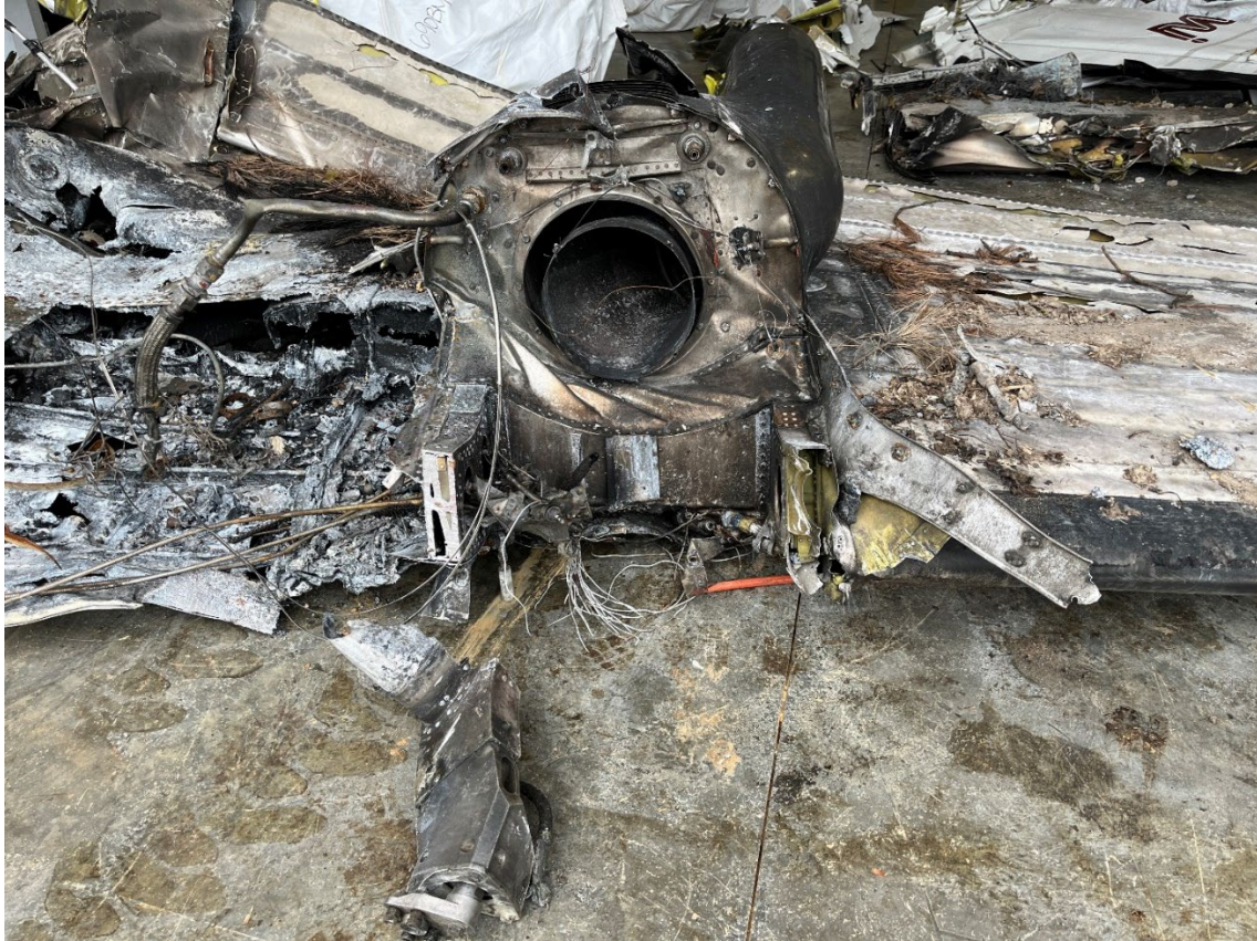
Figure 5. Right Engine Mounts (NTSB Photo)
