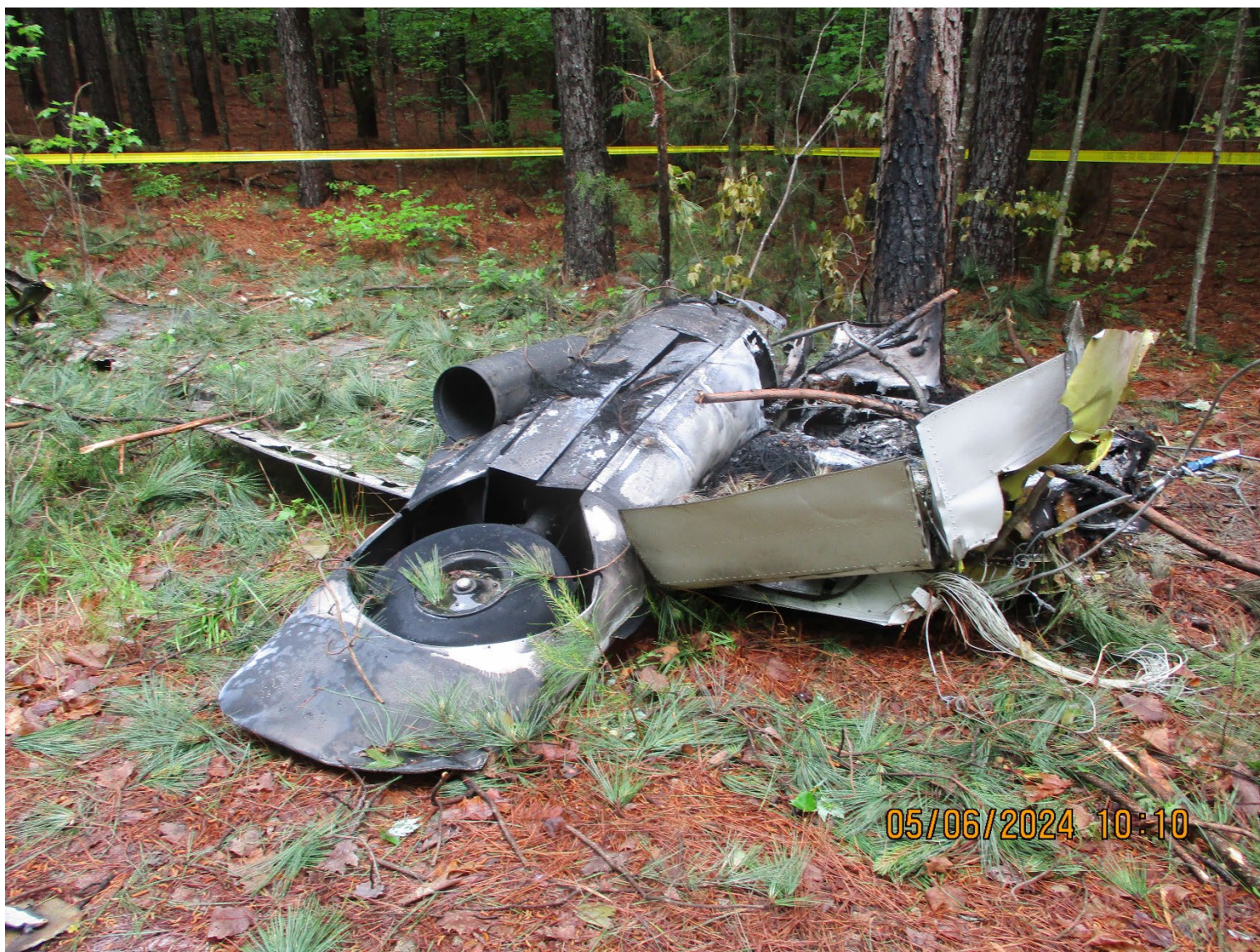
Photograph 2 - Right wing, note: engine missing
