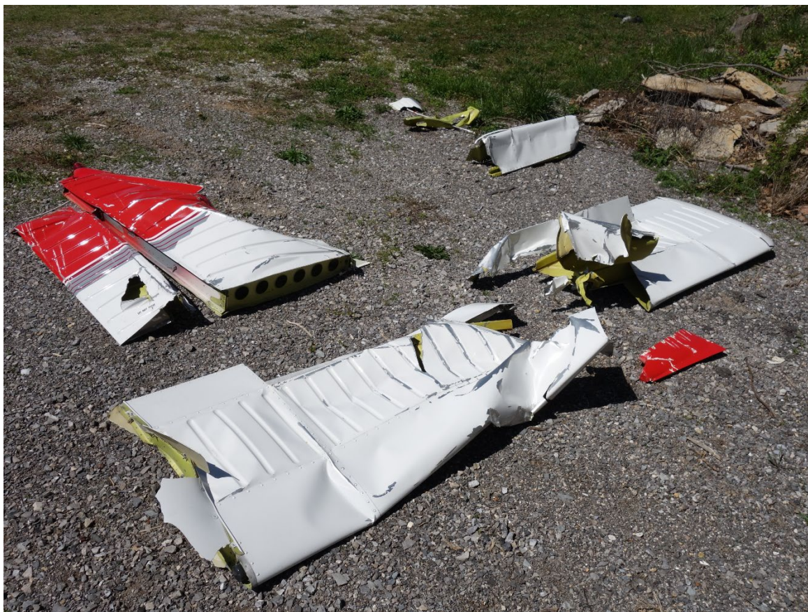
Photograph 3 - View of vertical stabilizer, rudder and horizontal stabilizer.
