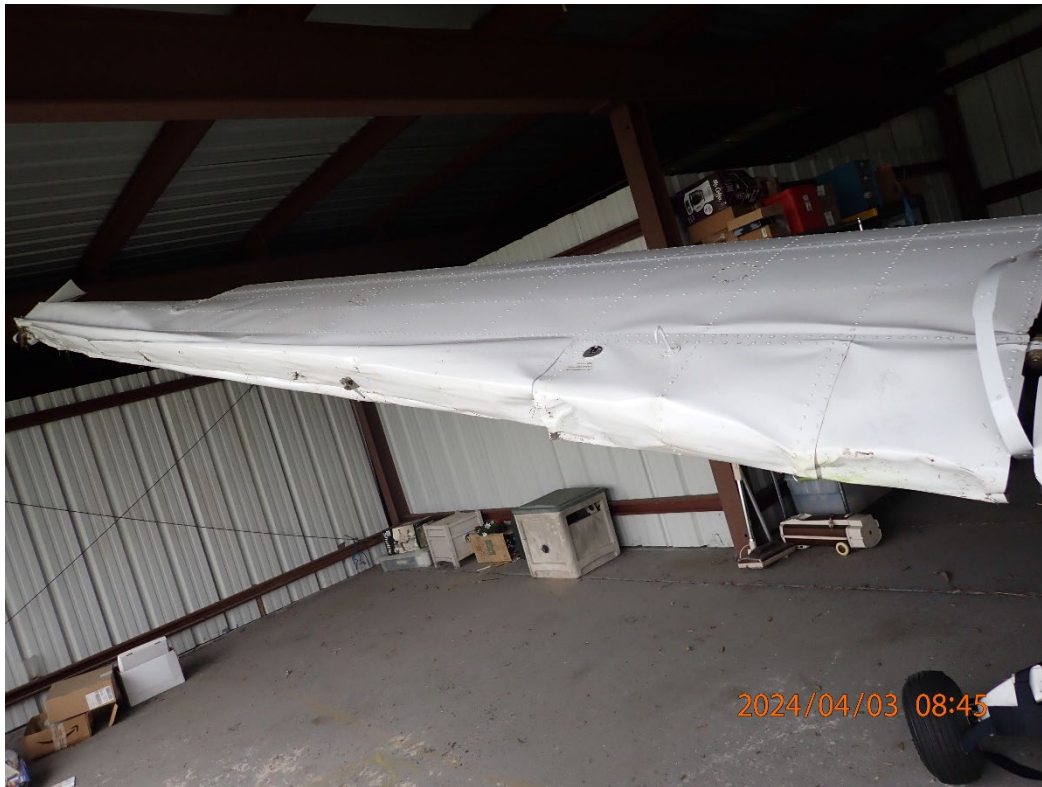
Photo 11: View of damage to the right wing.
