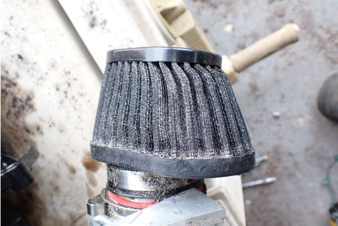
Photo 30: View of air intake filter.
