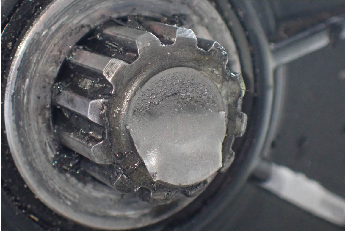
Photo 22: View of the overload fractured propeller driveshaft.
