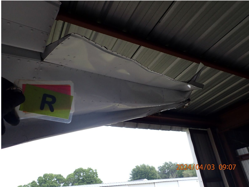
Photo 12: View of damage to the right aileron.
