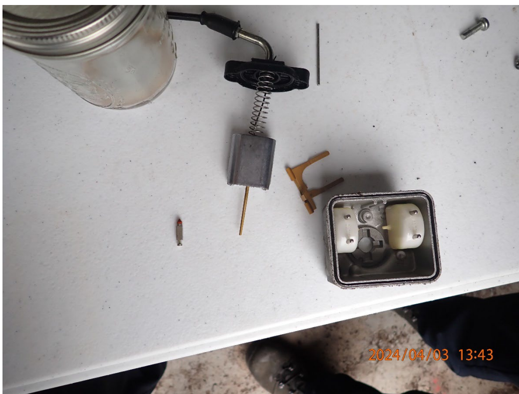
Photo 35: View of the disassembled carburetor pieces.
