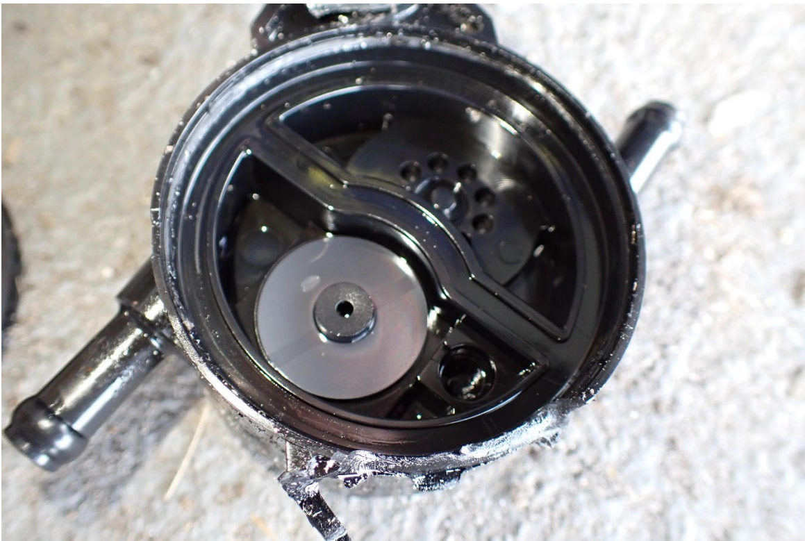
Photo 33: View of the disassembled fuel pump.
