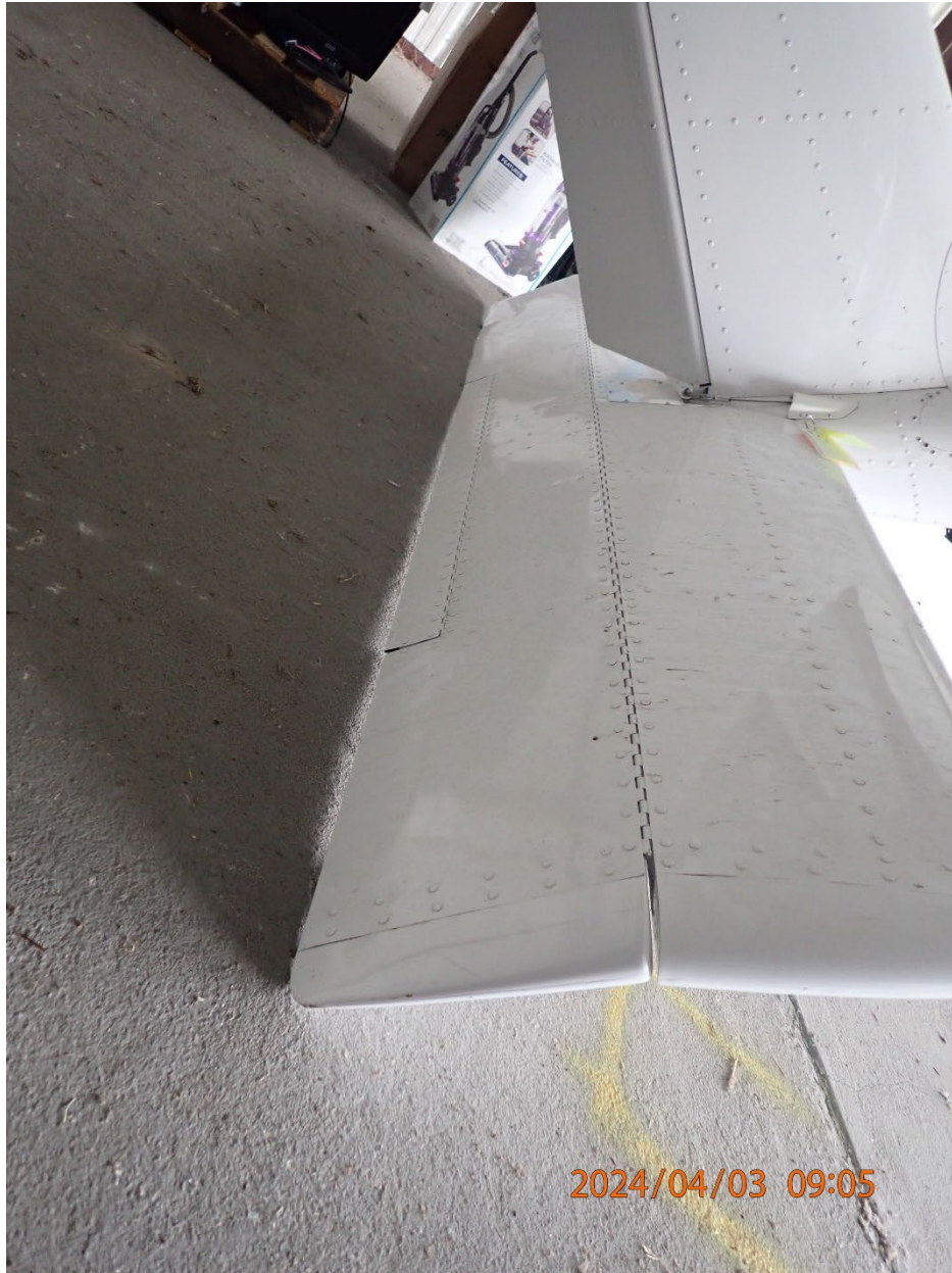
Photo 10: View of the elevator trim tab.
