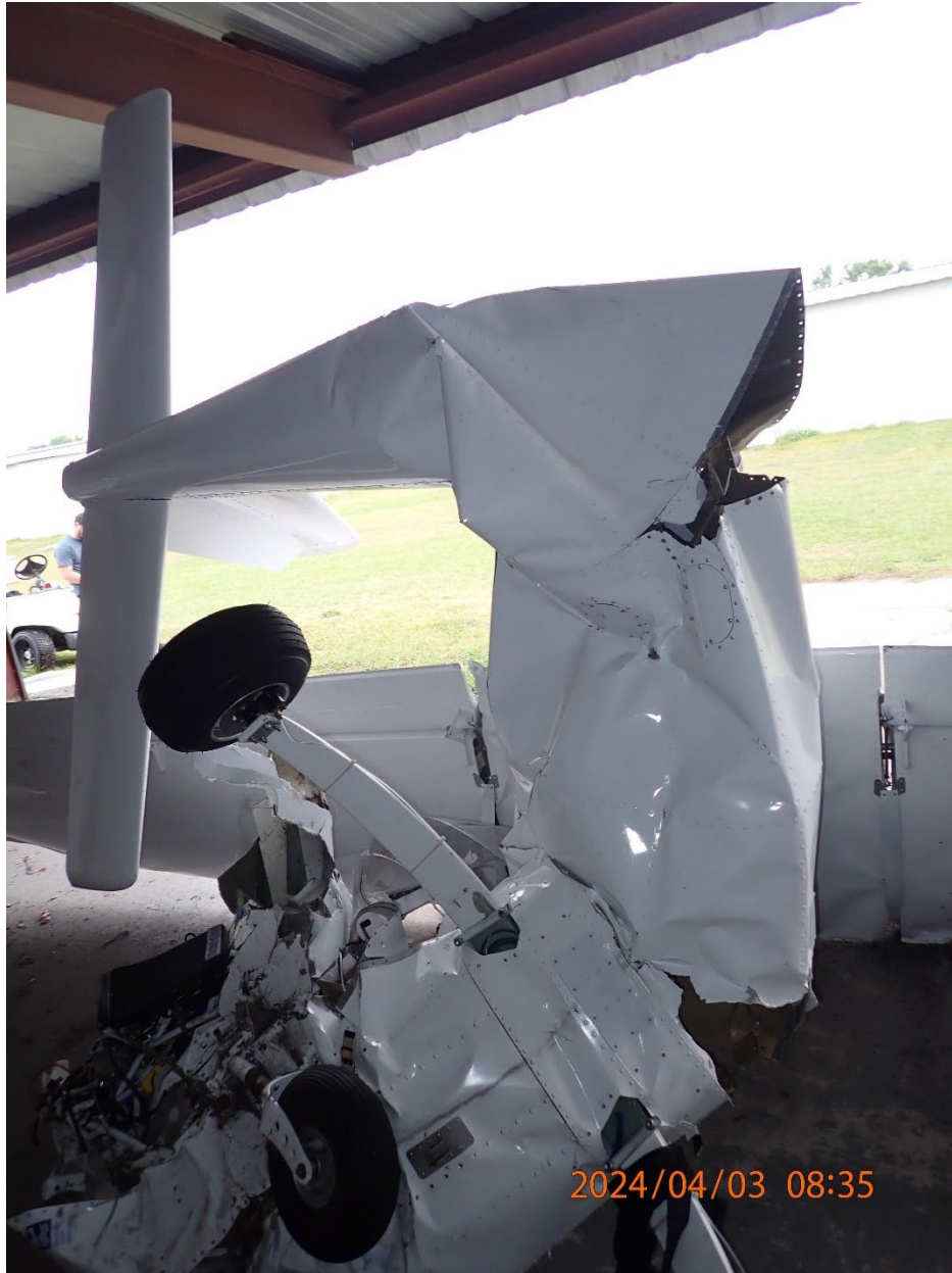
Photo 6: View of damage to the bottom of the empennage and fuselage.
