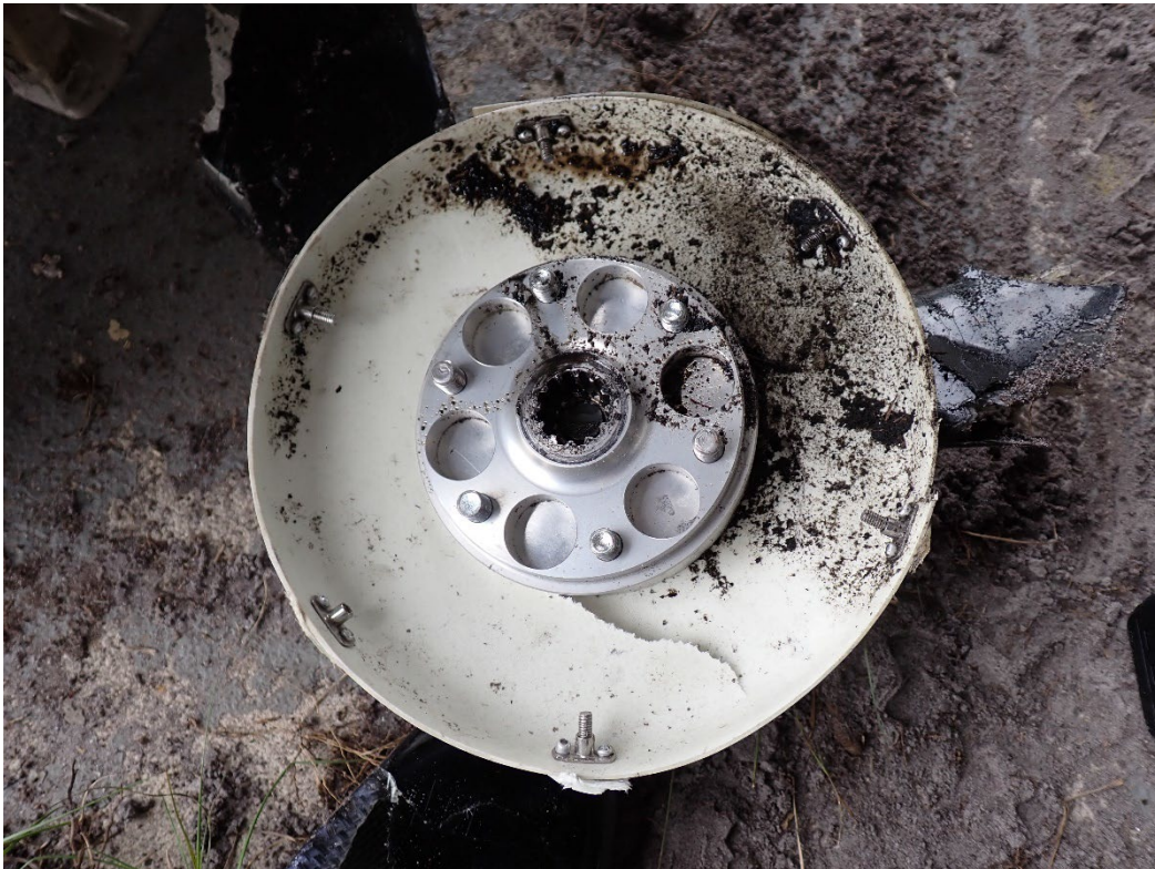
Photo 21: View of the impact separated propeller flange.
