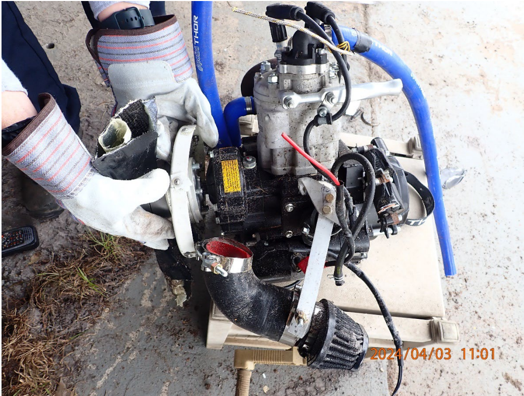
Photo 20: Overview of the impact separated engine.
