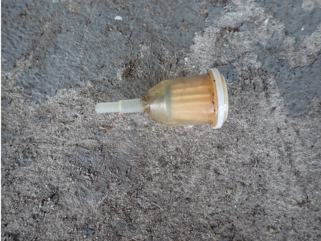
Photo 32: View of the inline fuel filter.
