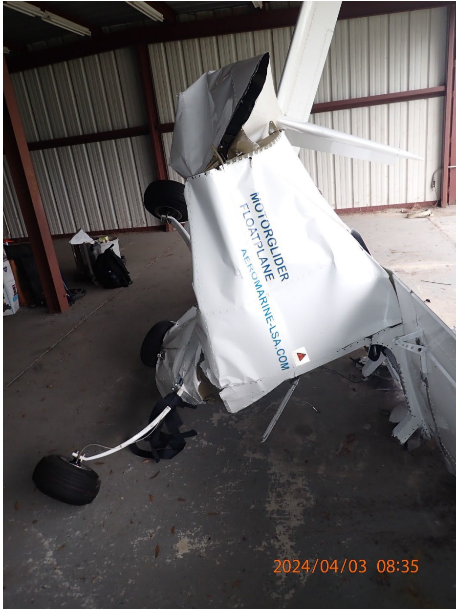
Photo 5: View of damage to the fuselage.
