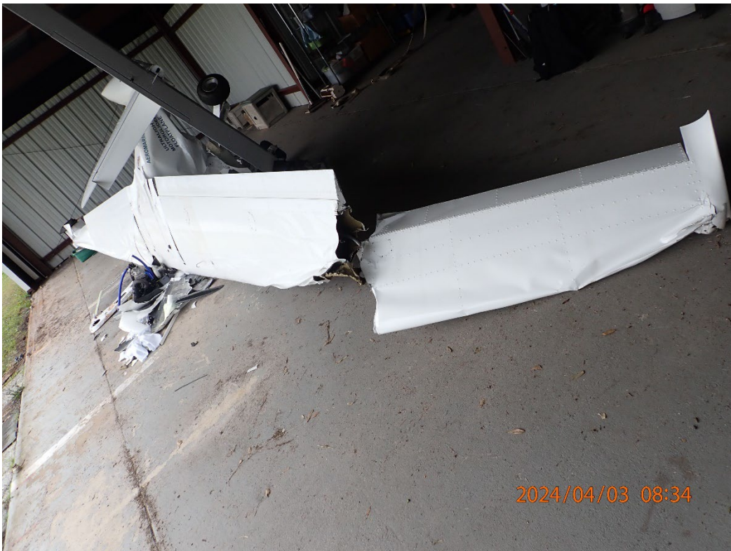
Photo 14: View of damage to the outboard left wing.
