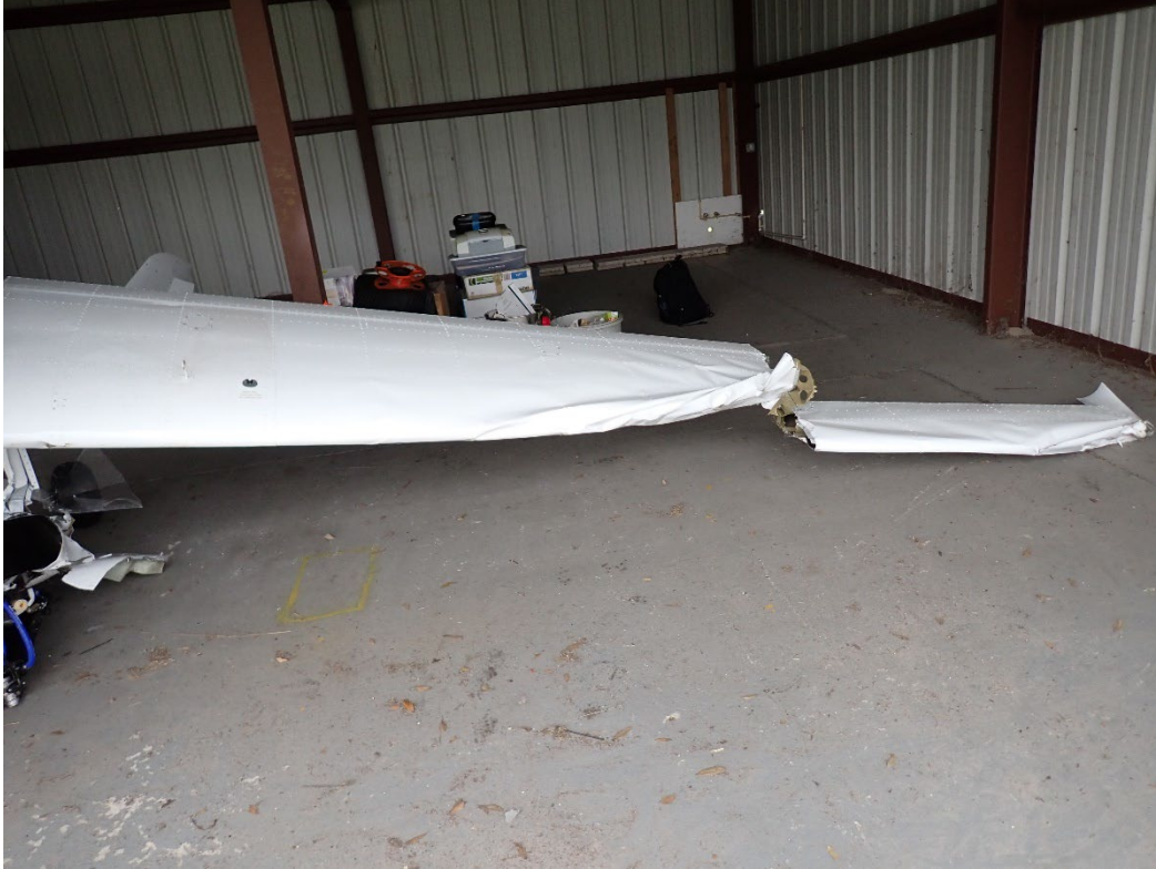
Photo 13: View of damage to the left wing.
