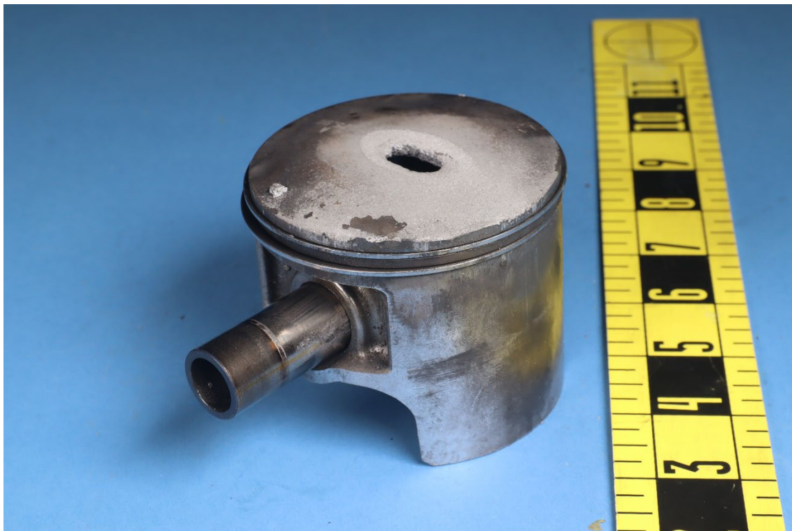
Figure 1. Overall view of the submitted components as received (upper image) and a closer view of the piston assembly showing a hole in the middle of the crown (lower image).
