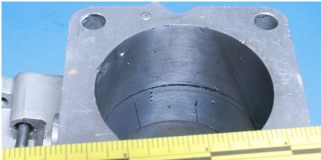
Figure 9. Angled view of the interior of the carburetor housing, after removal of the throttle arm assembly and plate, showing the circular witness mark in the bore from the plate edge.
