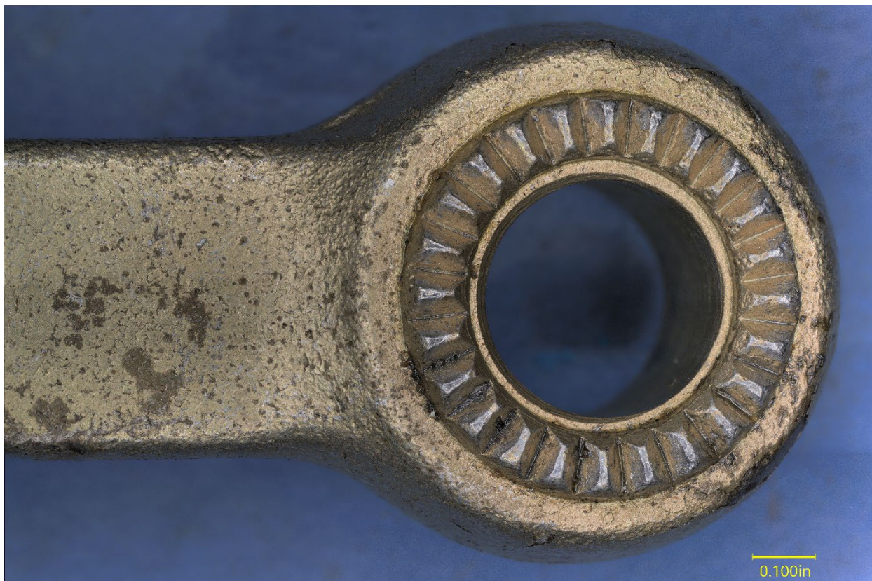
Figure 23. View of the teeth on the throttle lever, after disassembly and cleaning.
