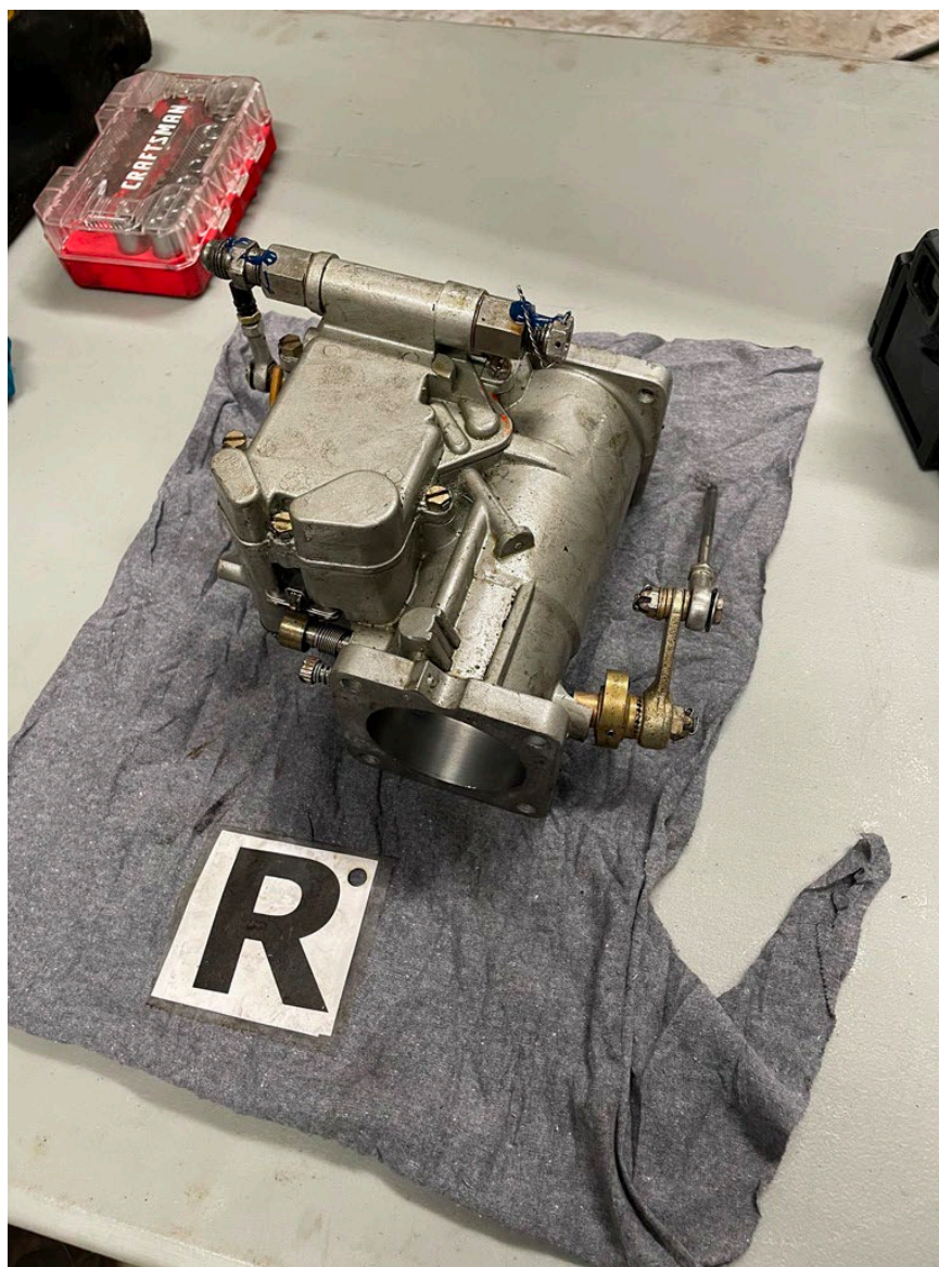
Photograph 5 - Right Engine Carburetor
