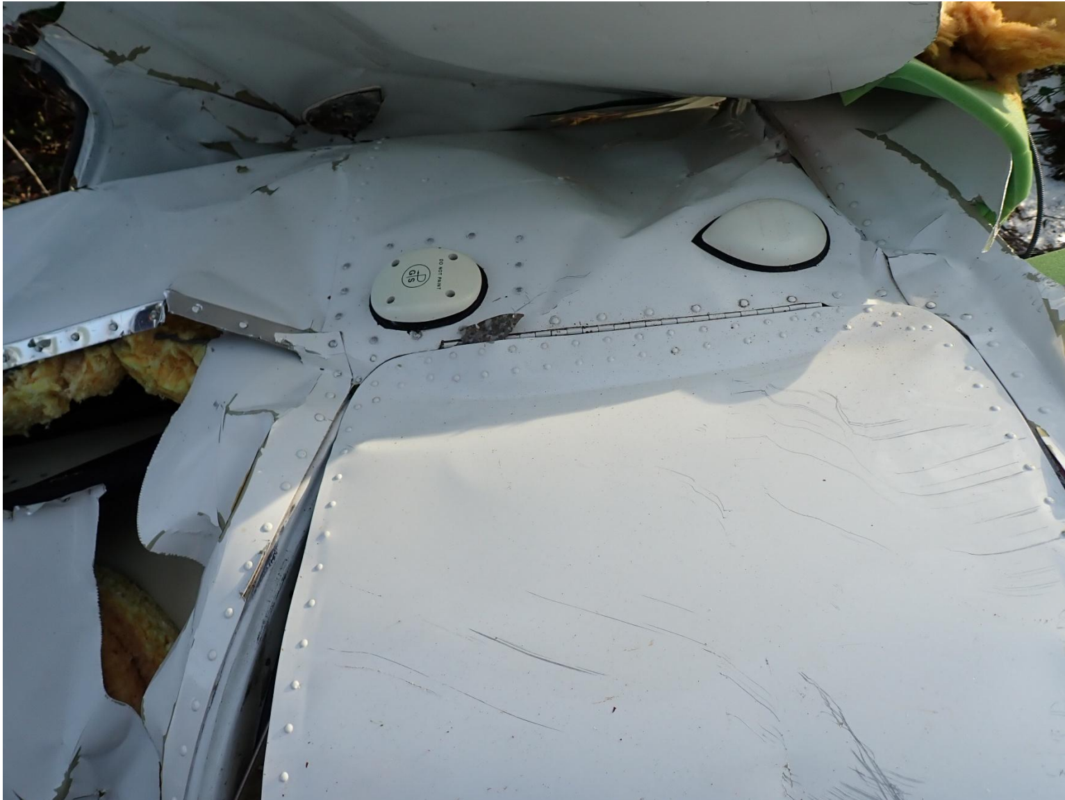
Photograph 4 - Baggage door in the closed position
