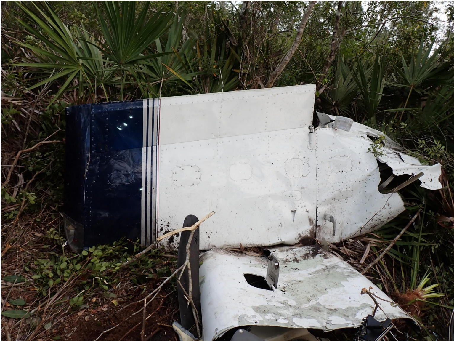
Photograph 2 - Part of the airplane's left wing outboard section
