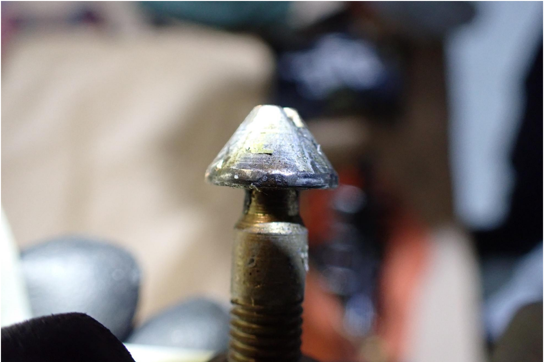
Photograph 9 - Main cabin door upper latch pin
