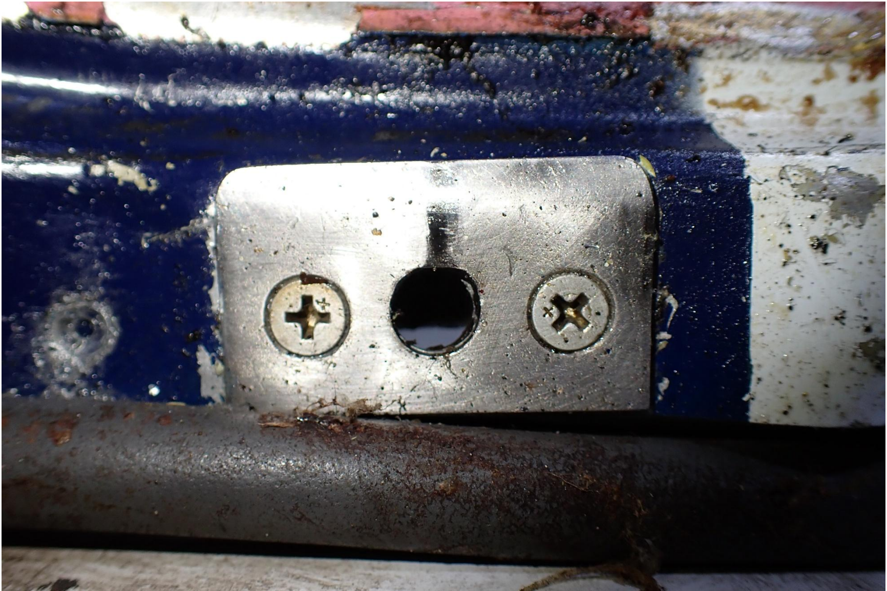
Photograph 7 - Main cabin door aft striker plate
