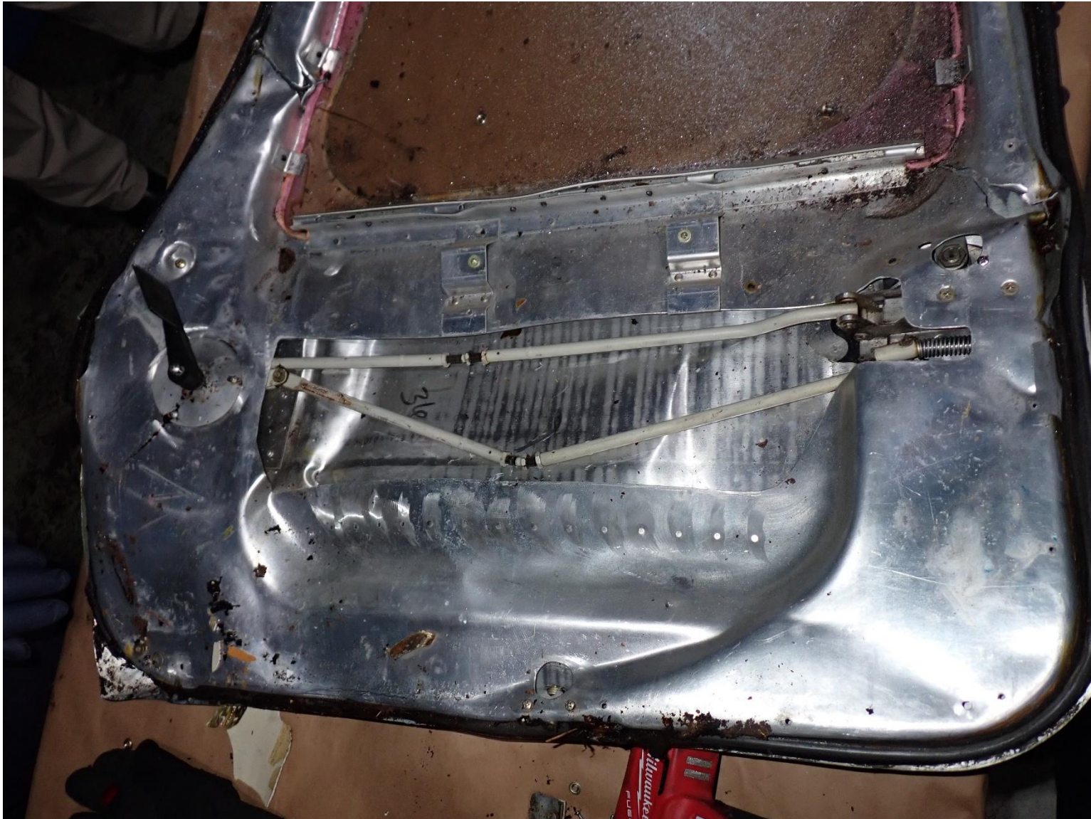
Photograph 5 - Main cabin door after partial disassembly
