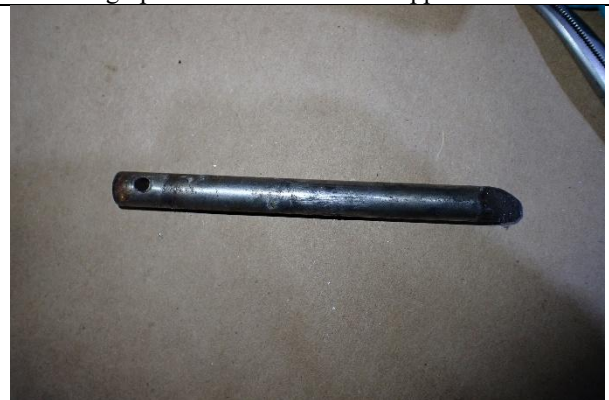
Photograph 17: Main cabin door aft door latch pin
