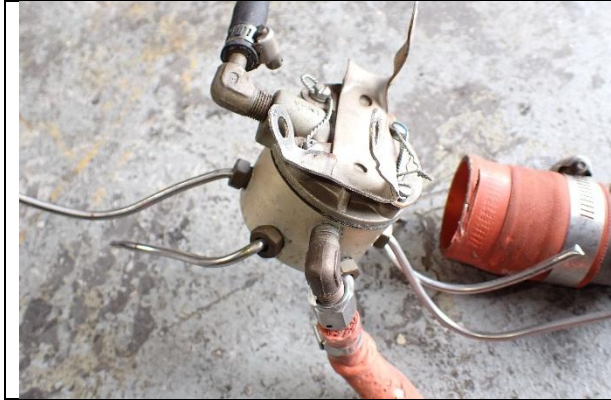
Photograph 40: Fuel manifold valve
