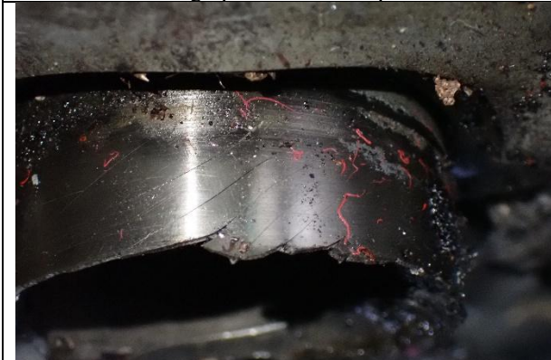
Photograph 32: Cracks in crankshaft
