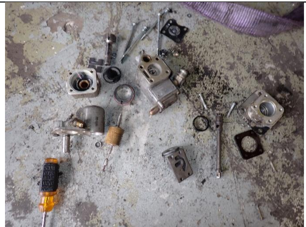
Photograph 35: Engine driven fuel pump (disassembled)
