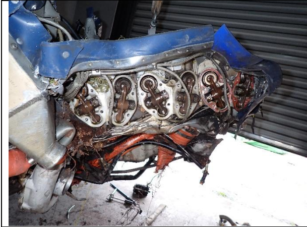
Photograph 28: Engine overhead components (right side)
