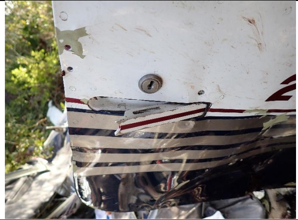
Photograph 7: Main cabin door outer latch handle
