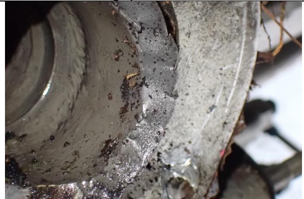
Photograph 33: Crankshaft fracture surface
