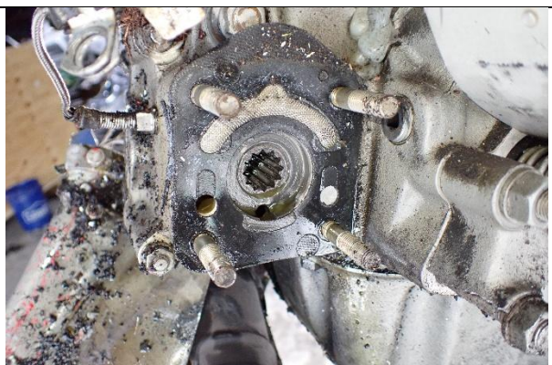
Photograph 48: Propeller governor gasket and screen
