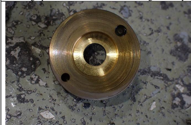
Photograph 38: Fuel metering assembly (disassembled)
