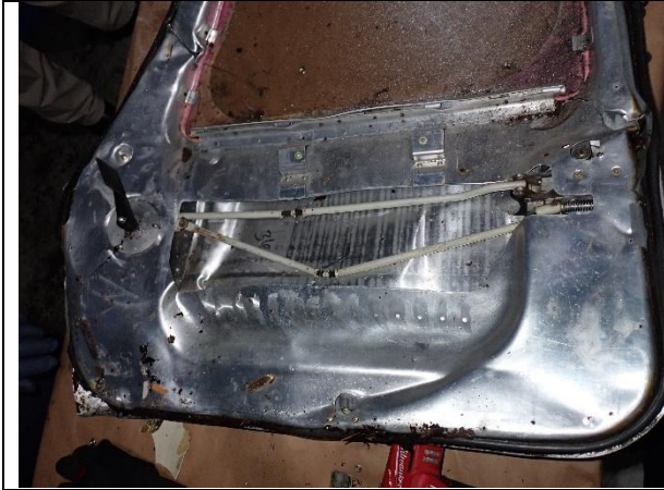
Photograph 12: Main cabin door after trim removal
