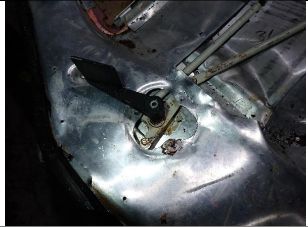
Photograph 13: Main cabin door interior door handle
