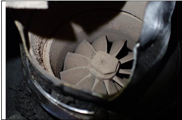
Photograph 43: Turbocharger turbine section
