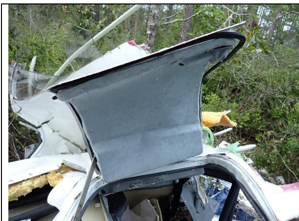
Photograph 18: Baggage door as found at accident site
