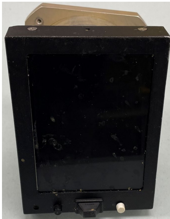
Figure 3. JPI EDM-730 removed and cleaned from the avionics panel.
